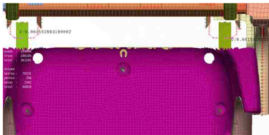
Figure 67 – Reference measurements defined to center the booster seat in the y-direction
