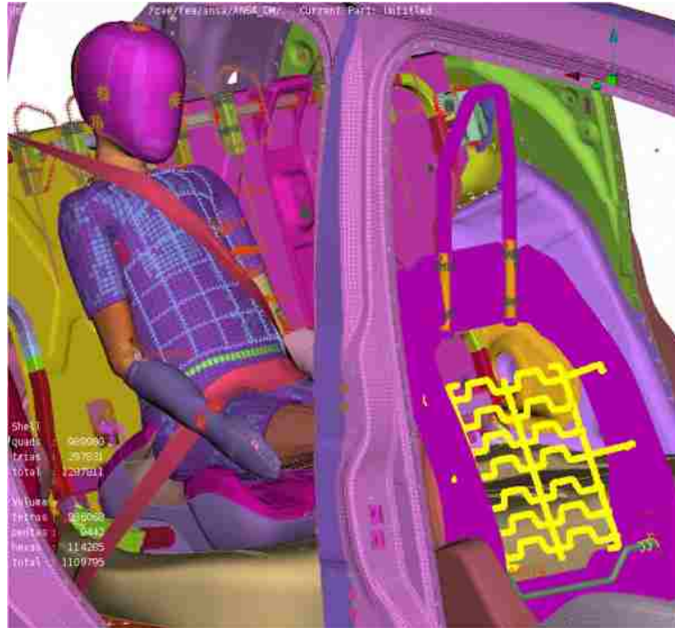
Figure 111 – Evidenced backseat frame of the front passenger seat
