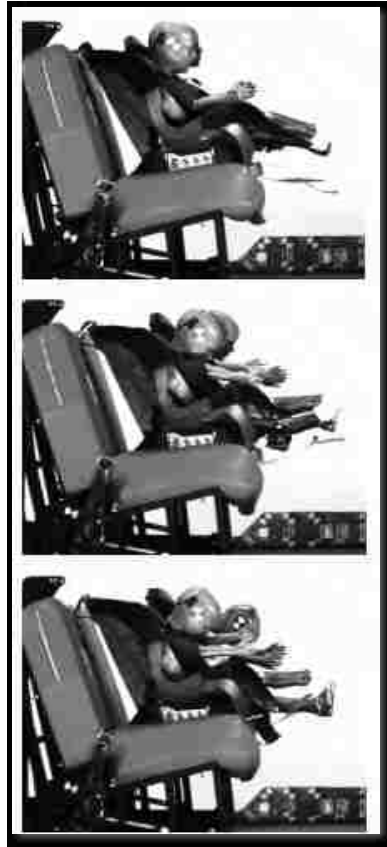
Figure 25 – Head excursion of children with tethered (front) and untethered (rear) top strap of the LATCH [41]
