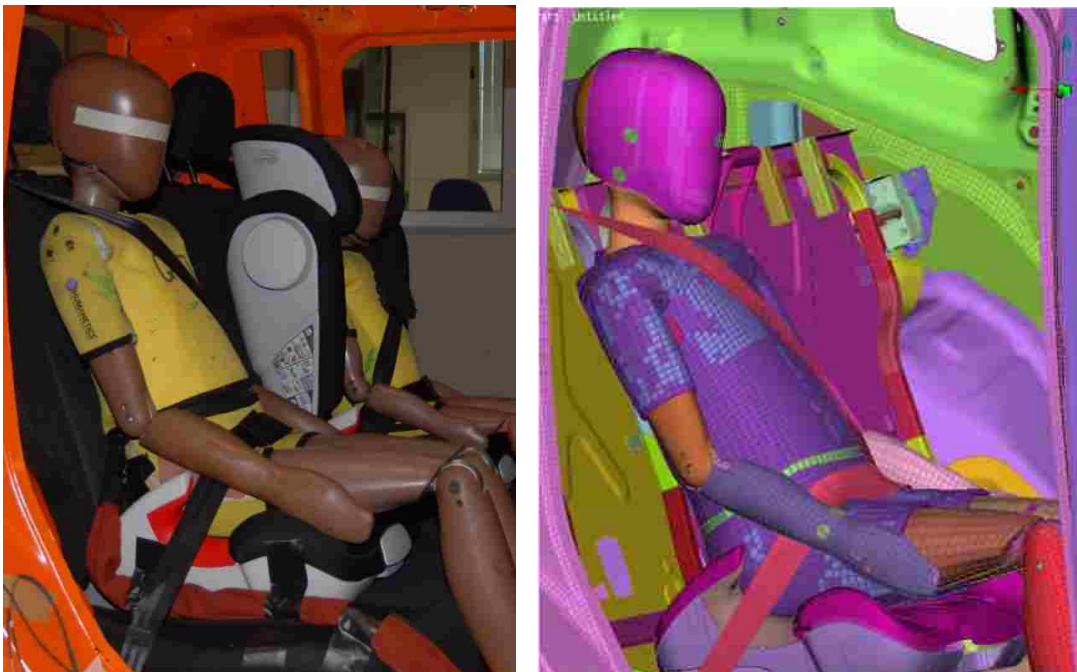
Figure 104 – Right view of experimental and numerical Q10 before the performing of the sled test
