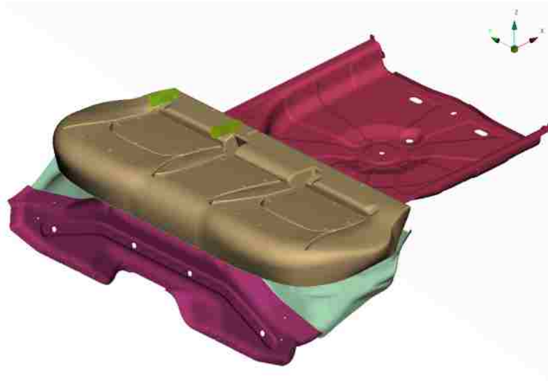
Figure 71 – Master file of foam depenetration simulation
