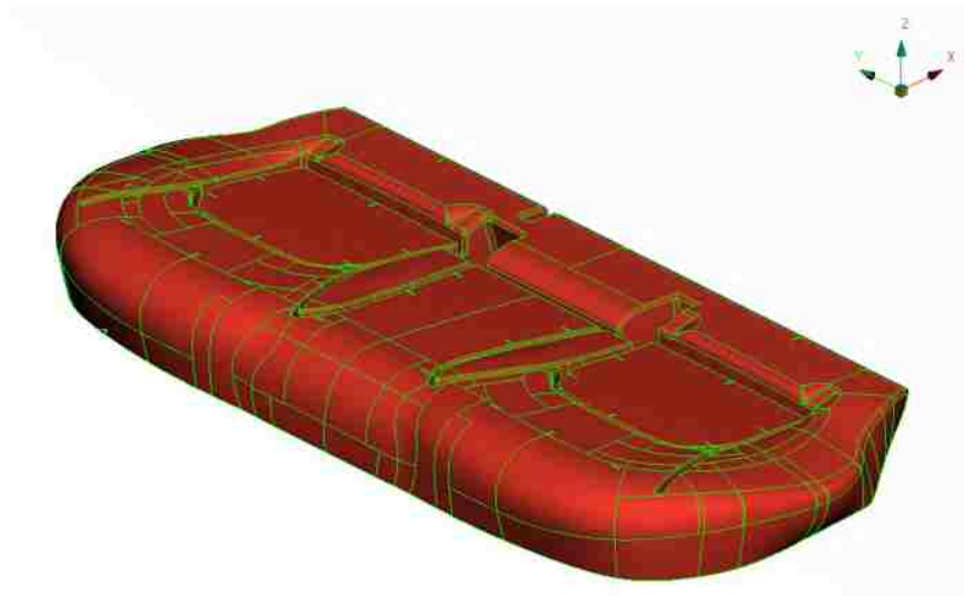
Figure 57 – Healed CAD of the seat foam
