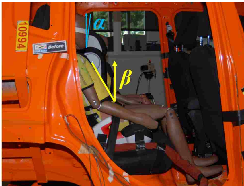
Figure 76 – Additional angle used for positioning the Q10
