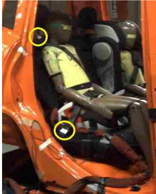
Figure 109 – Location of lap and shoulder belt tensiometers
