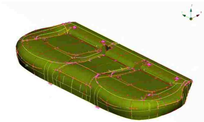
Figure 55 – Isometric view of the CAD model of the backseat foam
