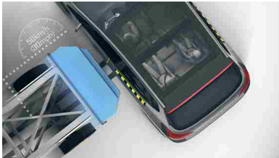
Figure 36 – The Euro NCAP Side Impact Mobile Deformable Barrier test [74]
