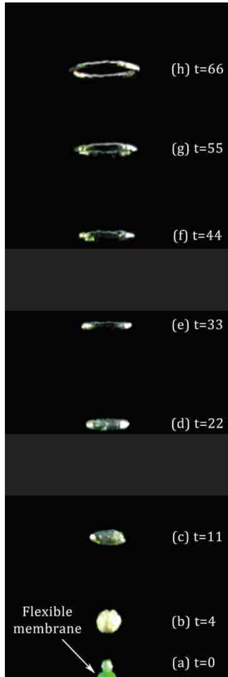
FIGURE 6.4: Formation and translation of the vortex ring bubble corresponding to Bo=85 . Values are dimensionless.
