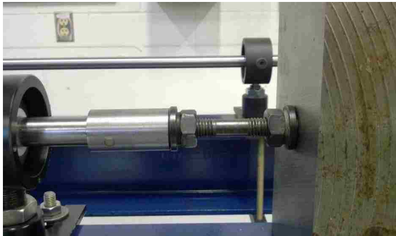
Figure 47: Set up of jack screw used to apply a compressive load on the bars for calibration of strain gauges
