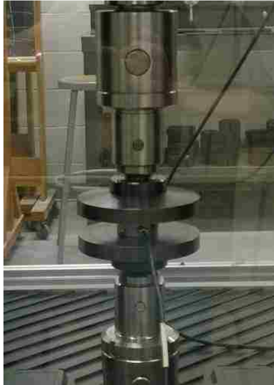
Figure 45: MTS tester applying a load on the LC305 load cell
