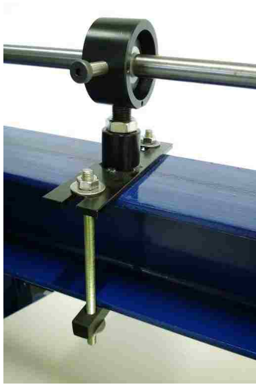
Figure 18: Bar holder clamped to support frame.
