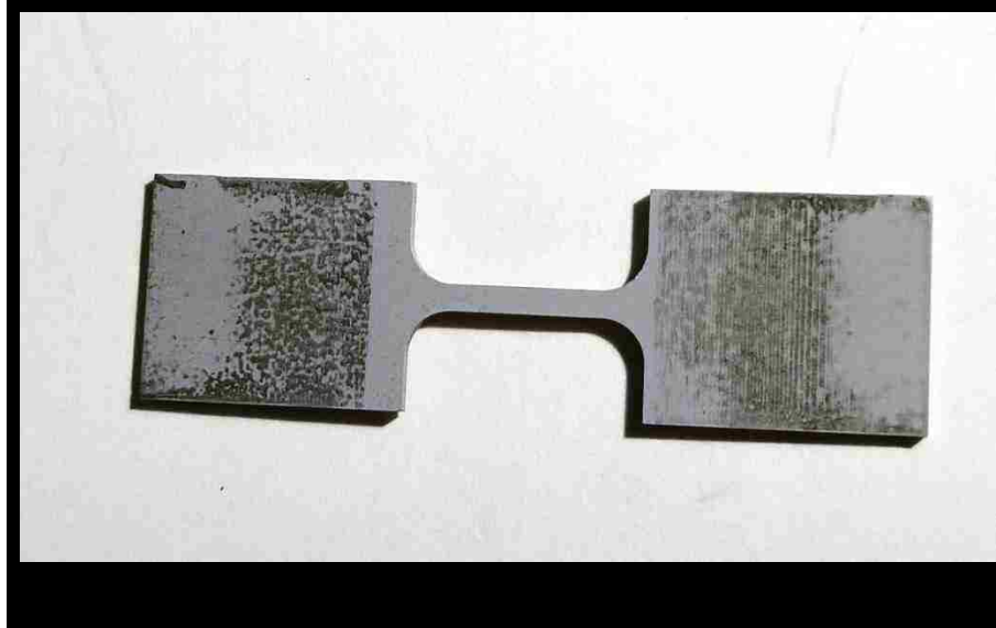
Figure 23: Specimen showing serrations from specimen slot in bars
