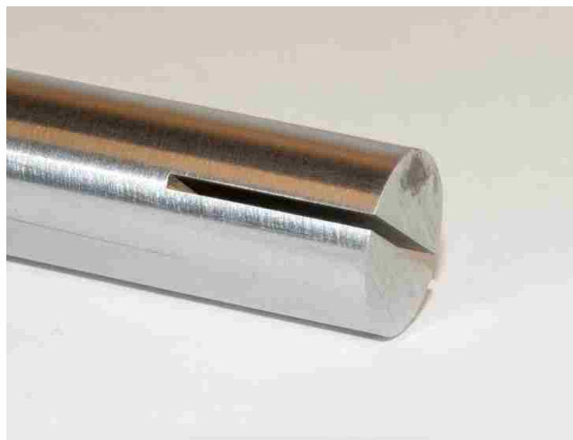
Figure 22: Slot in bars to hold test specimen
