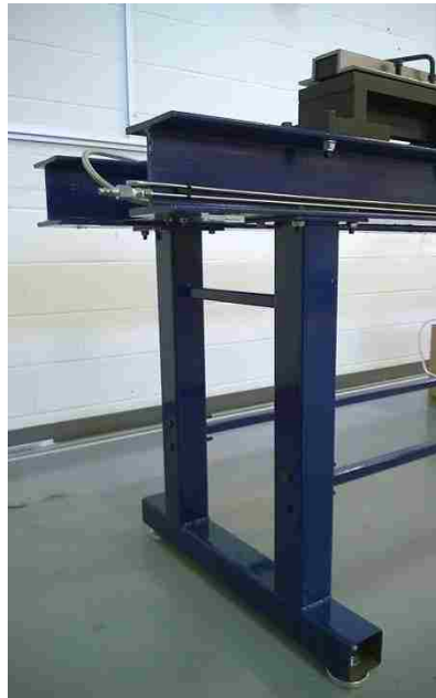
Figure 13: Support frame for SHPB apparatus
