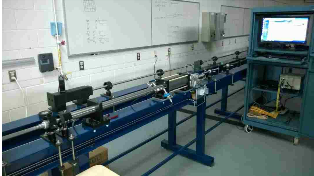
Figure 38: Computer cabinet for storing DAQ system
