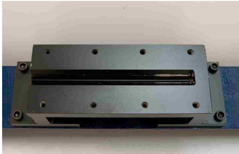
Figure 30: V groove in momentum trap base
