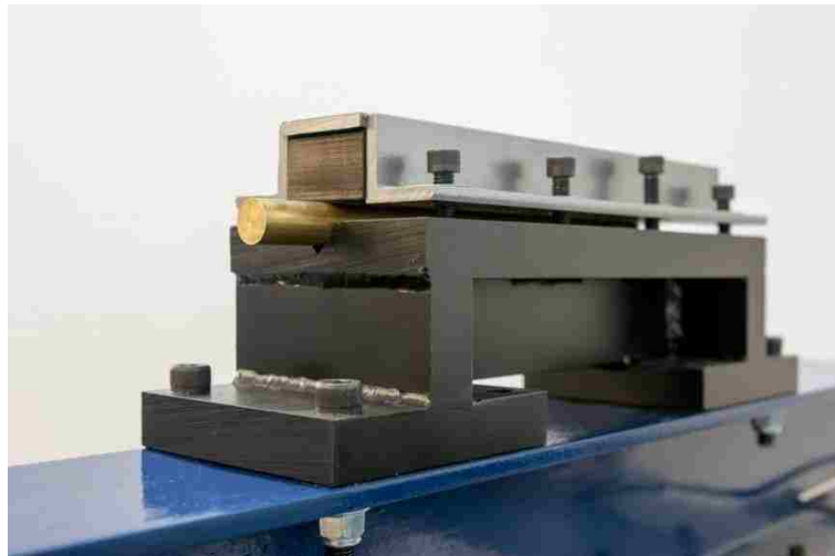
Figure 29: Momentum trap assembly
