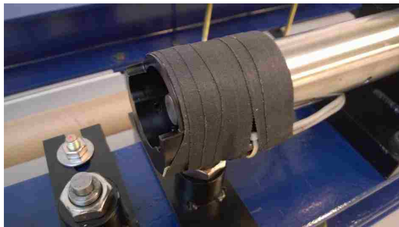
Figure 41: Optical gate to measure striker velocity
