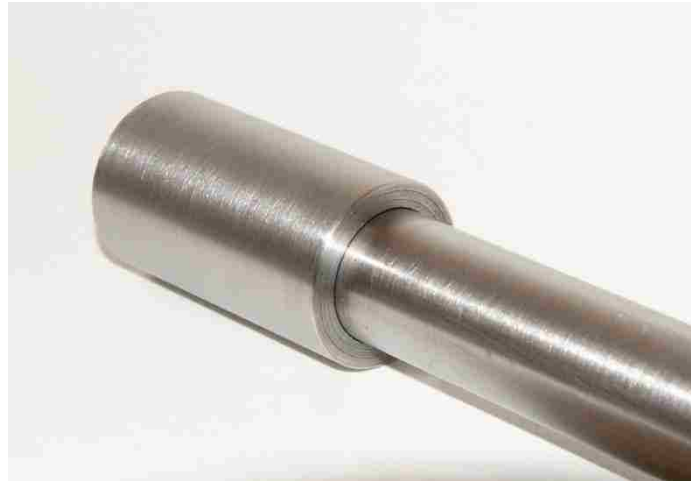
Figure 20: Close up view of the bar and anvil attached
