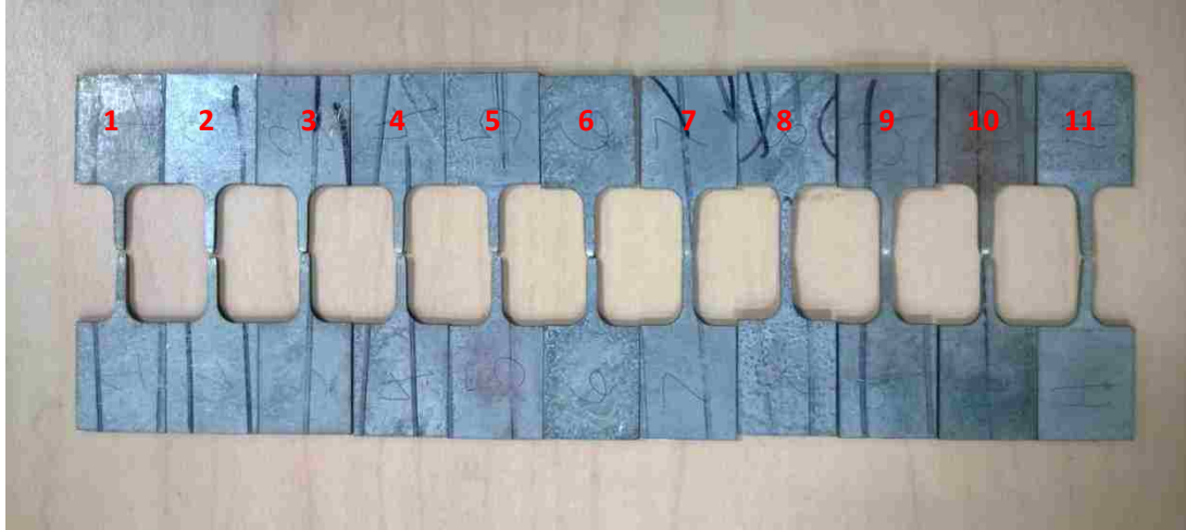
Figure 62: RD fracture location
