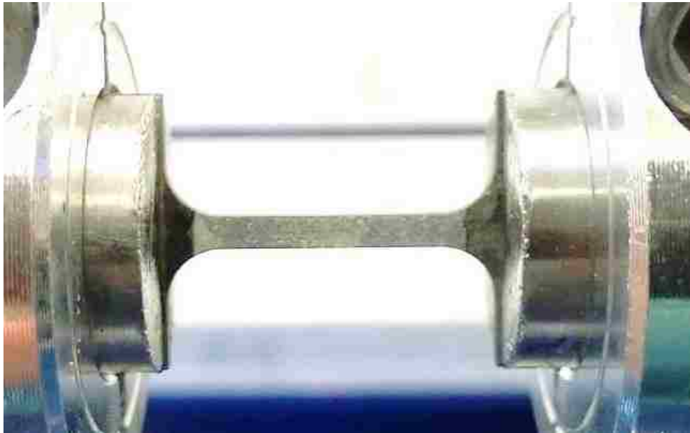
Figure 60: Mounted specimen with black marker at bar/specimen interface to show if slipping occurs
