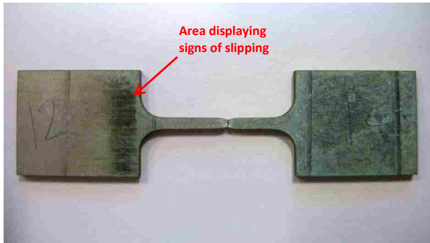
Figure 66: Sample specimen showing evidence of slipping in bar specimen slot
