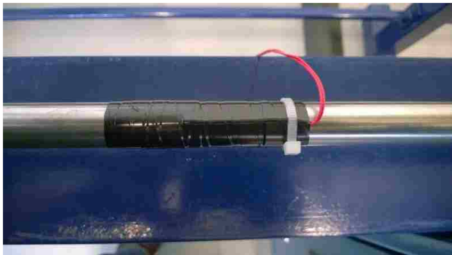
Figure 39: Strain gauge wrapped with electrical tape
