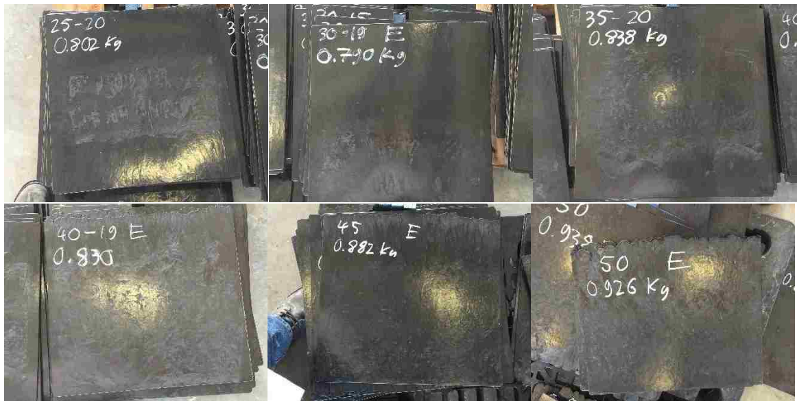
Figure 4.3 Carbon fiber-reinforced thermoplastic panels produced by LFT-D
