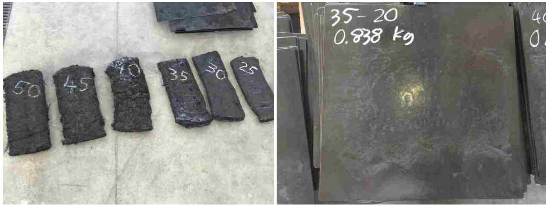
(a) (b) Figure 4.2 Carbon fiber-reinforced thermoplastic charge and panel by LFT-D
