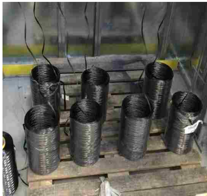
Figure 2.3 7 carbon fiber in rovings prepared for LFT-D feeding
