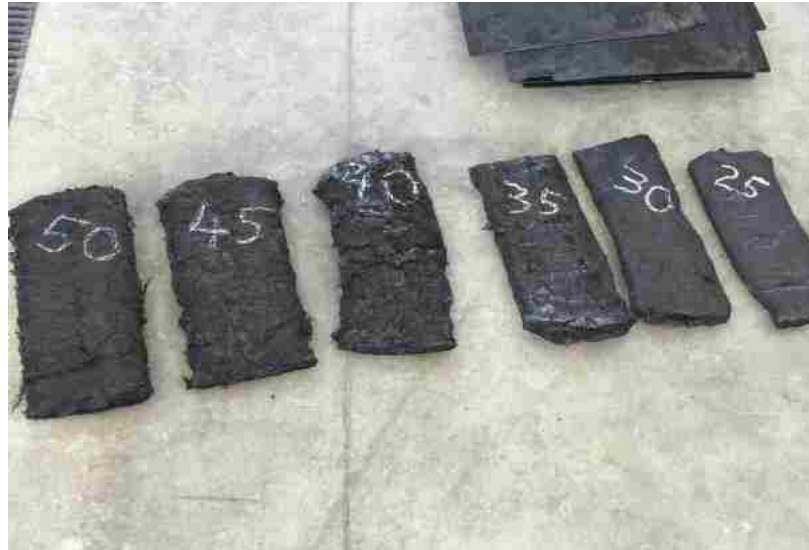
Figure 2.3 8 Charge produced by LFT-D prepared for press
