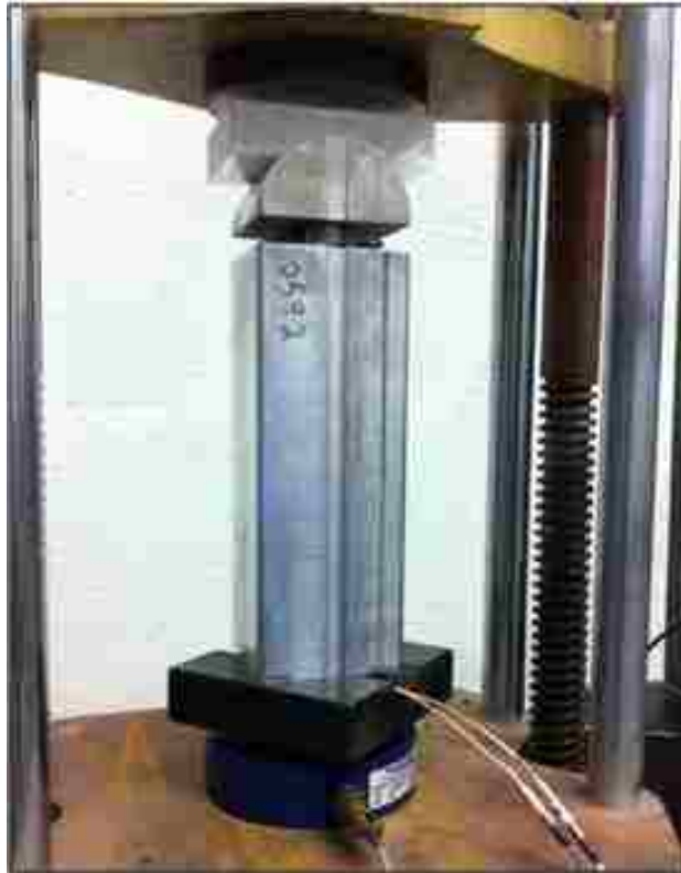
Figure 8: Projectile Load Cell Calibration Process
