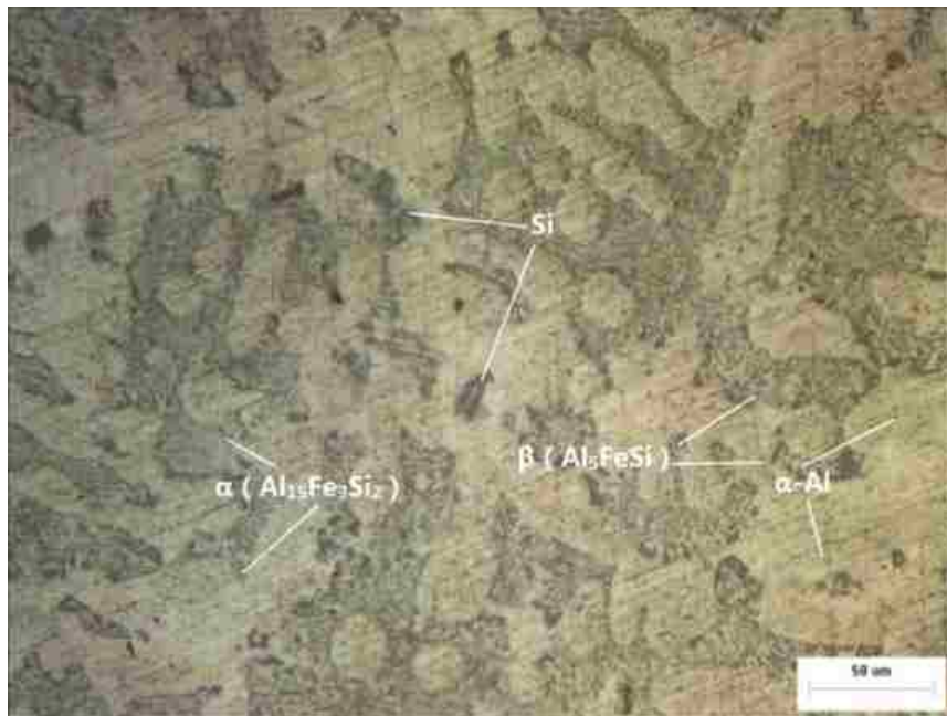
Figure 2.3-3 Optical micrograph showing microstructure of the recycled alloy
