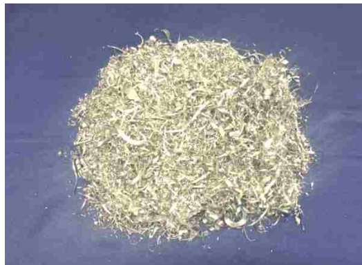
Figure 2.2-1 Machining chips of aluminum alloy A380.
