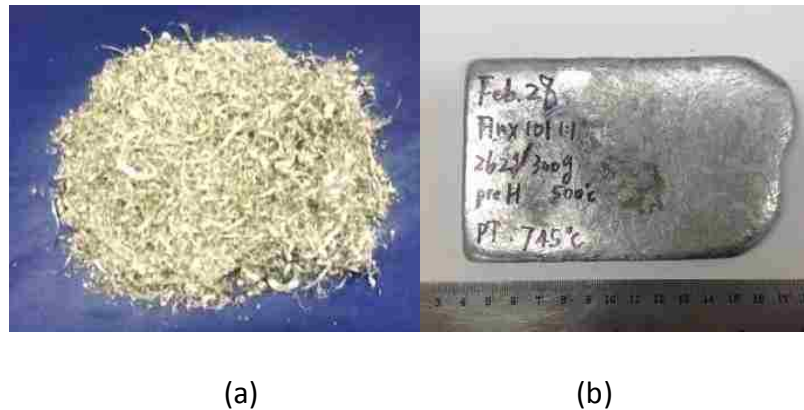
Figure 4.2-2 (a) machining chips of aluminum alloy 380, and (b) a cast plate of the recycled alloy.
