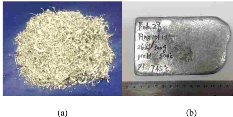
Figure 5.2-2 (a) machining chips of aluminum alloy 380, and (b) a cast plate of the recycled alloy.
