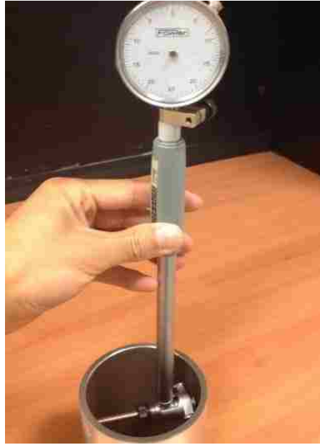
Fig.7.3 Diameter measurement using a dial bore gage.
