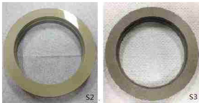
Fig.5.2. PEO coated samples S-2 and S-3.
