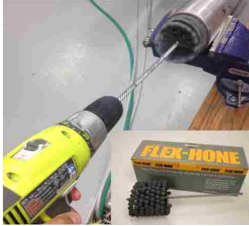
Fig.7.2. Honing brush and the honing process.
