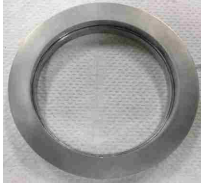
Fig.5.1 The ring-shaped aluminum 6061 sample.
