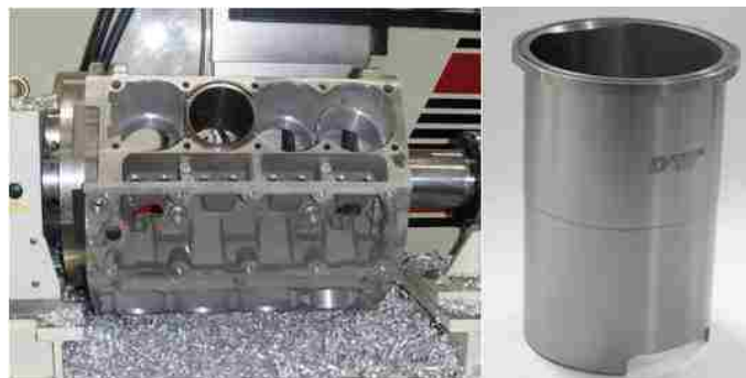
Fig.2.3 Aluminum cylinder engine block with inserted cast iron liners [22].
