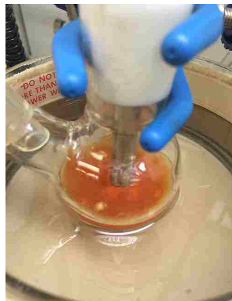
A. B. Figure 6.67. Ti-O Homolysis test; A. \text{Cp}_2\text{TiCl}(\text{OEt}) in THF at 60^\circ\text{C} at the start of reaction (yellow); B. Change in color from yellow to orange after 3 hours.
