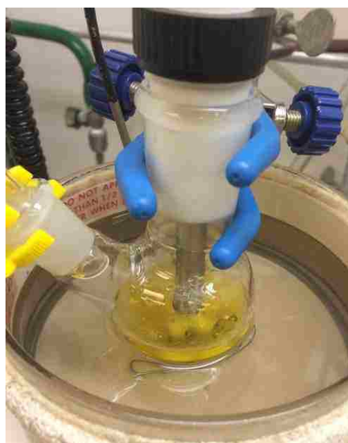
A. B. Figure 6.67. Ti-O Homolysis test; A. \text{Cp}_2\text{TiCl}(\text{OEt}) in THF at 60^\circ\text{C} at the start of reaction (yellow); B. Change in color from yellow to orange after 3 hours.
