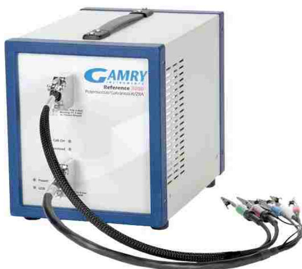
Figure 6.6. A photo of the Gamry Potentiostat/Galvanostat/ZRA model 3000 available at Lehigh University in Prof. Kai Landskron lab.
