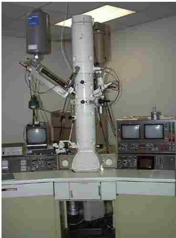
Figure 6.5. A photo of the JEOL JEM-2000FX microscope at Lehigh University department of Materials Science and Engineering [189].
