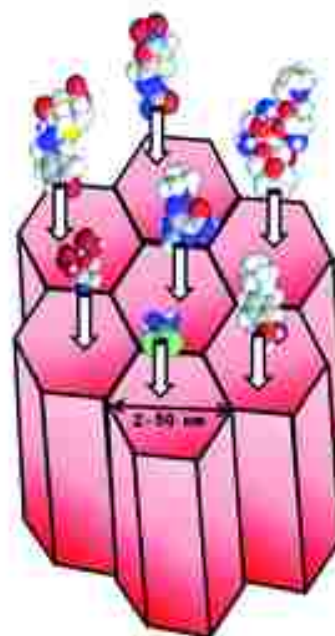
Fig 1-16. Top: Functionalization of silica pore wall, Bottom: Drug loading. Ref[5]
