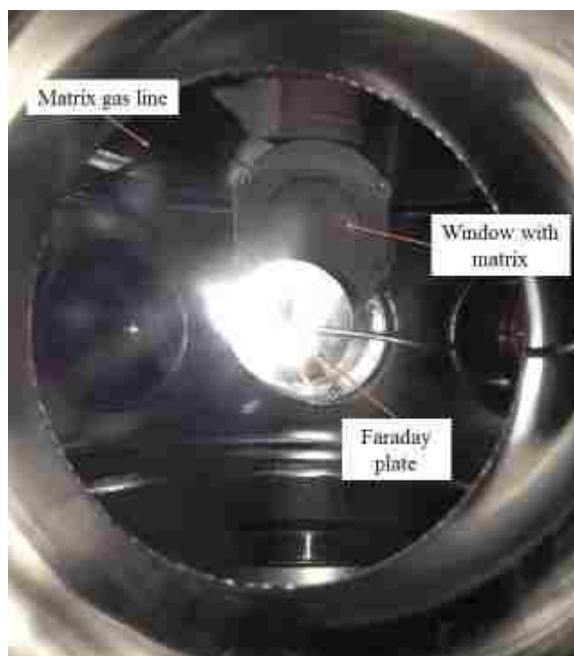
Figure 2.11 Picture through Kodial glass viewport showing IR window after 4 hours of matrix deposition.
