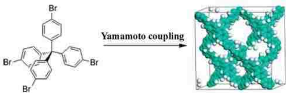
Figure 1-2. Synthesis scheme of a PAF-1 with ultrahigh surface area by the Yamamoto-type Ullmann cross-coupling reaction. Ref. 27.
