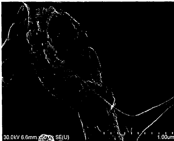
Figure 15 - SEM Micrograph of C_5N Lamellar Structure
