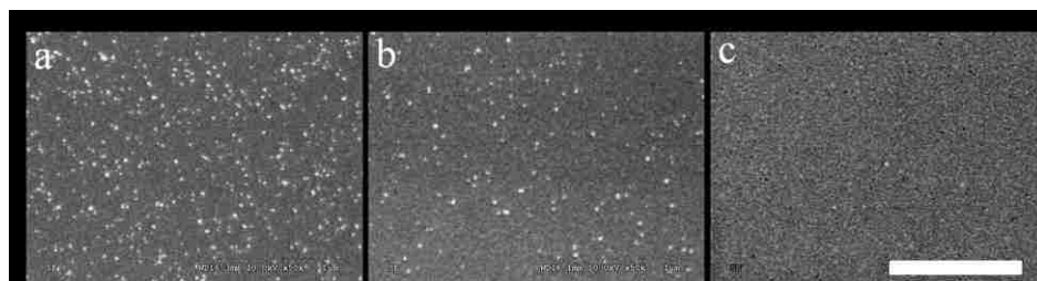
Figure 3.6 Scanning Electron Microscopy (SEM) images of competitive adsorption of MutEG and DNA. The relative MutEG and DNA concentrations are 10 (a), 200 (b) and 2000 (c) respectively. The scale bar is 1 \mu\text{m} .
