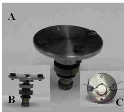
Figure 2.1 (A) Molybdenum sample stub. (B) Side view of the molybdenum sample stub. (C) Top view of the Mo sample stub with the Pt(111) crystal mounted with Ta wires and Mo screws.
