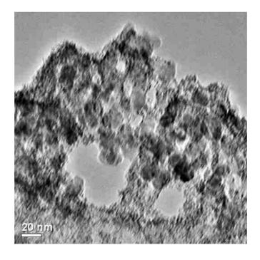
Figure 2.2 TEM picture neat SiC nanoparticles
