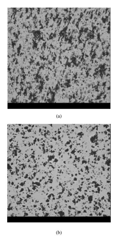
Figure 2.7 Morphology of graphite dispersions: (a) 0.75 vol% of neat graphite, (b) 0.75 vol% of AG-graphite. (Scale bar=5  $\mu$ m)
