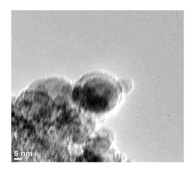
Figure 3.4 TEM picture of neat  $TiO_2$  nanoparticles
