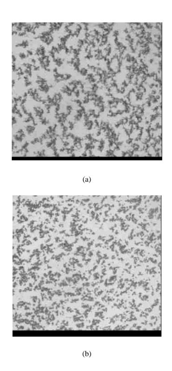
Figure 2.9 Morphology of SiC dispersions: (a) 0.5 vol% of neat SiC, (b) 0.5 vol% of AG-SiC. (Scale bar=100  $\mu m)$
