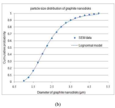
Figure 2.1 Morphology of neat graphite nanodisks, (a) SEM picture, (b) size distribution curve fitted by lognormal model.
