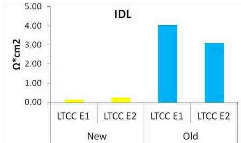
Figure 24: Instrument detection limits with lock-in amplifier and LTCC device with smaller electrode array (New) and without (Old)
