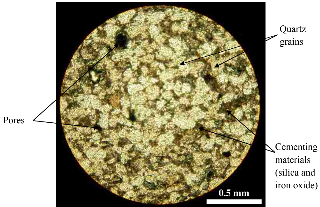
Figure 3.2 Photomicrograph of the sandstone used in the experiment
