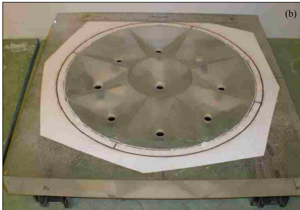
Figure 3.6 The bottom plate that divides the flow area into nine equal-area sections: conceptual design (a) and the finished bottom plate (b).
