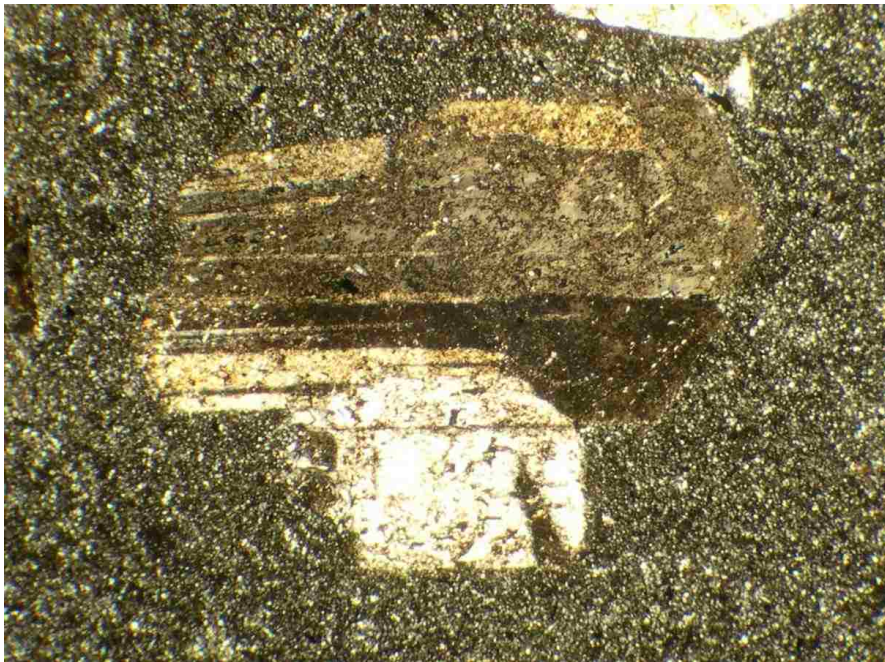
Figure 24, Photomicrographs of type 3 plagioclase feldspars altered to pure albite (R0733, hypabyssal dacite sill of the River Mountains stratovolcano suite; W30, Wilson Ridge pluton late phase rhyodacite dike)
