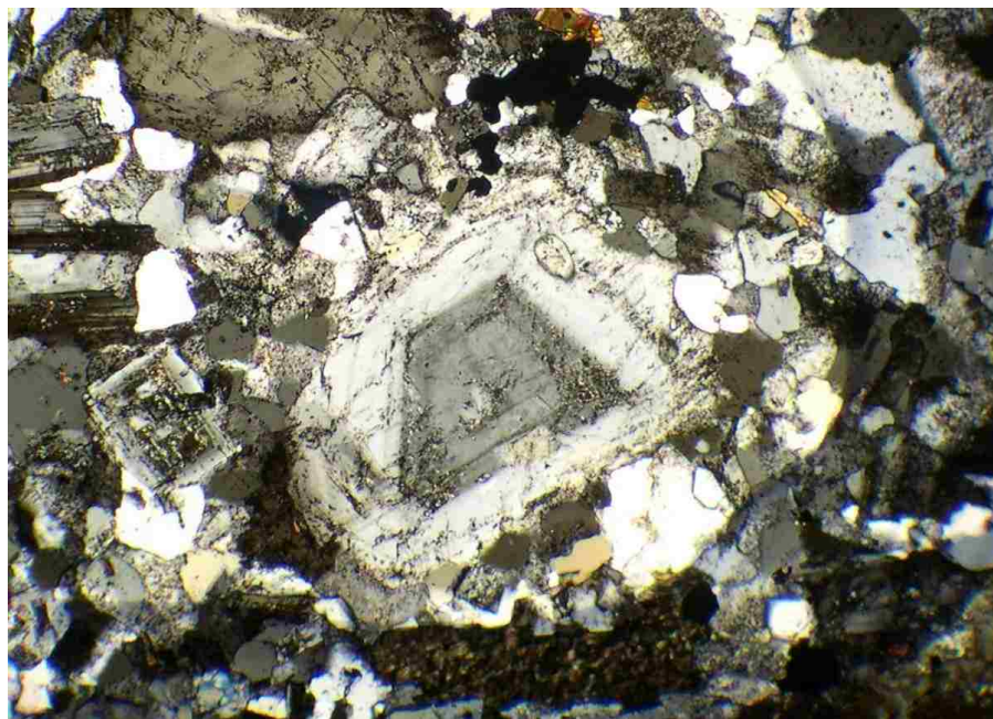
Figure 23, Photomicrographs of type 2 plagioclase feldspars with dramatic changes in An# from rim to core accompanied by changes in Fe contents reflect magma mixing. Samples R34, (RM dacite intrusion) and W076 (WRP quartz monzonite).
