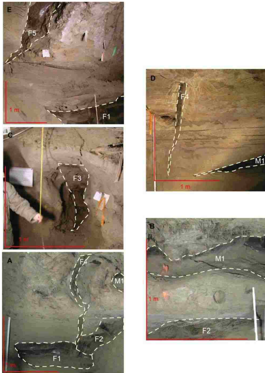
Figure 3.5. Photographs of five freeze and melt events. Photographs showing the relative position and stratigraphic placement of five freeze (F1 through F5) events and one melt (M1) event (dashed outlines) from the CRREL Permafrost Tunnel. A) Wedge 35S in F1 (0.5 m above ground level inside tunnel), the secondary wedge at 35S in F2, the 34S Pool in M1, and the F4 wedge above Wedge 35S. B) Closer view of the 34S pool in M1 (~ 1.2 m above ground level) and the 35S secondary wedge beneath it in F2. C) Wedge 18N in F3 (~1.5 m above ground level), with an approximately 1.5 m person standing beside the wedge. D) Wedge 52.5N in F4 (~ 3 m above ground level) with 50S pool ice in M1 below it. E) Wedge 64S in F5 (4 + m above ground level) extends up into the ceiling of the tunnel and lies stratigraphically above Wedge 64S in F1.
