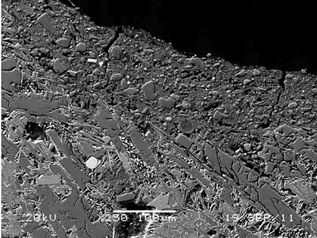
Figure S37. Pronghorn sample P31JC. Possible dissolution textures and increased porosity in the interior of the sample, but also either an alteration rind or a deposit on the original sample surface.
