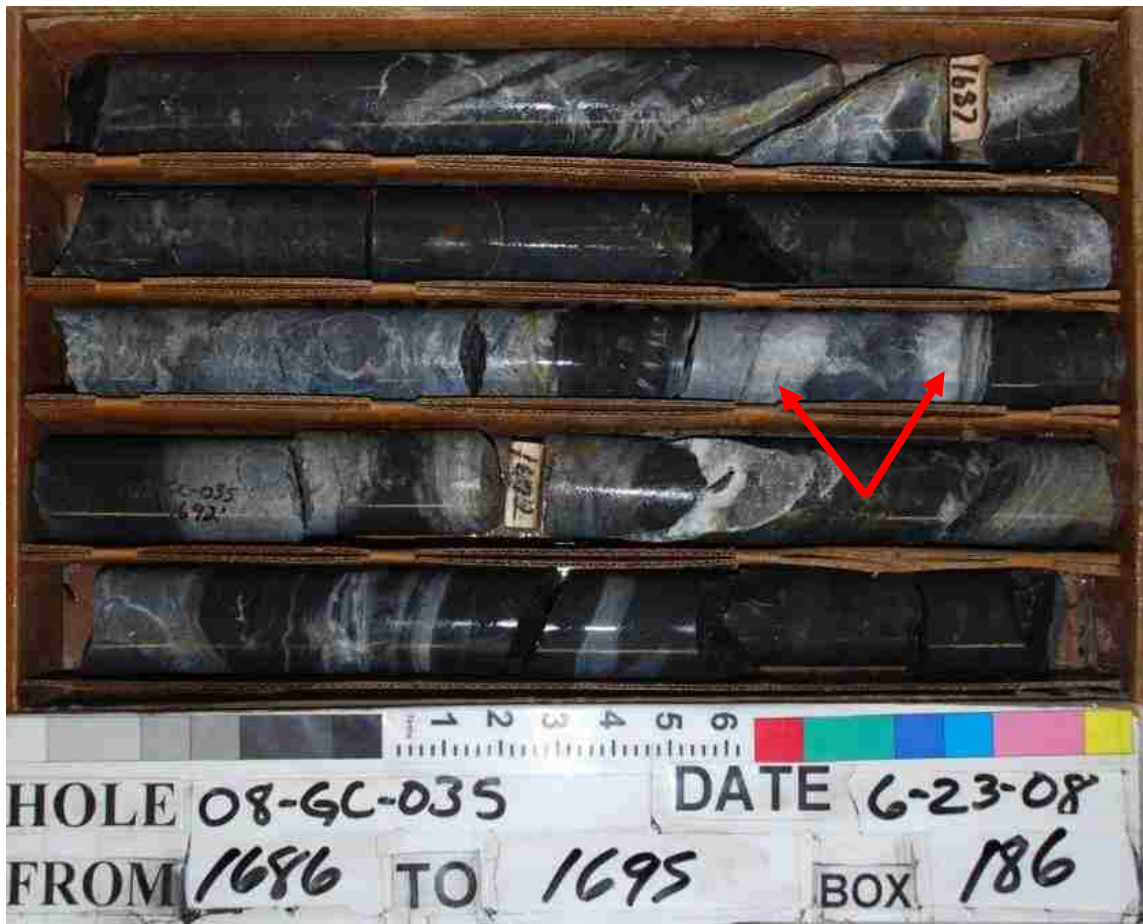
Figure 9. A section of siliceous carbonaceous mudstone with inter-beds of limestone turbidites. The limestones in the section locally have some alteration to calc-silicate minerals (red arrows) which is common in the upper intercepts of the siliceous carbonaceous mudstones in Cross Section B (63.5 mm diameter core).
