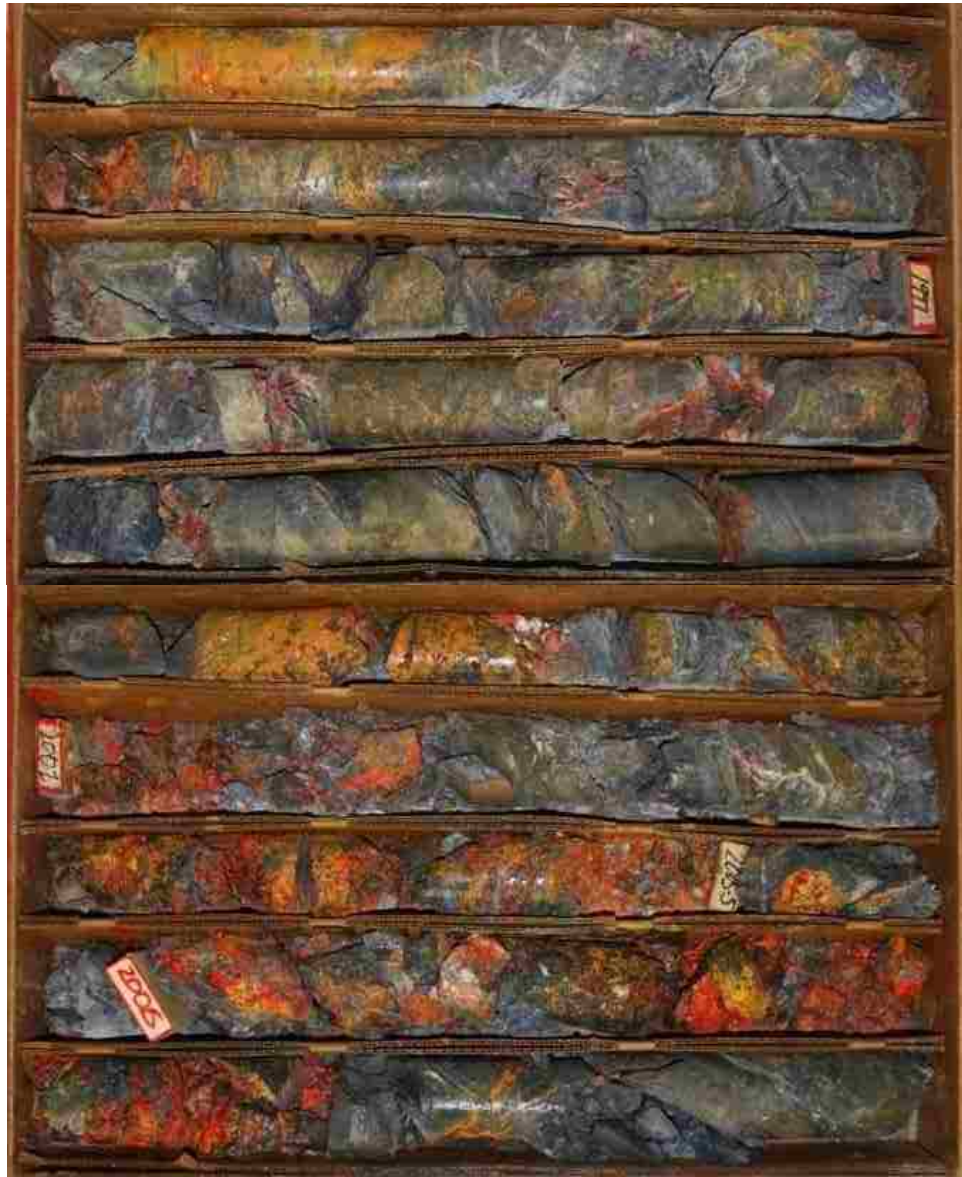
Figure 38b. (Continued from 36a) Continuing down-hole the siliceous carbonaceous mudstones inter-bedded with limestones from 1988.8'-2010' show strong decalcification and silicification indicating these rocks were not calc-silicate altered by the intrusion of the Osgood Stock. These rocks range in grade from 0.200 to 1.000 oz/t Au. The zone continues until it reaches the Getchell Fault at ~2046' (63.5 mm diameter core).
