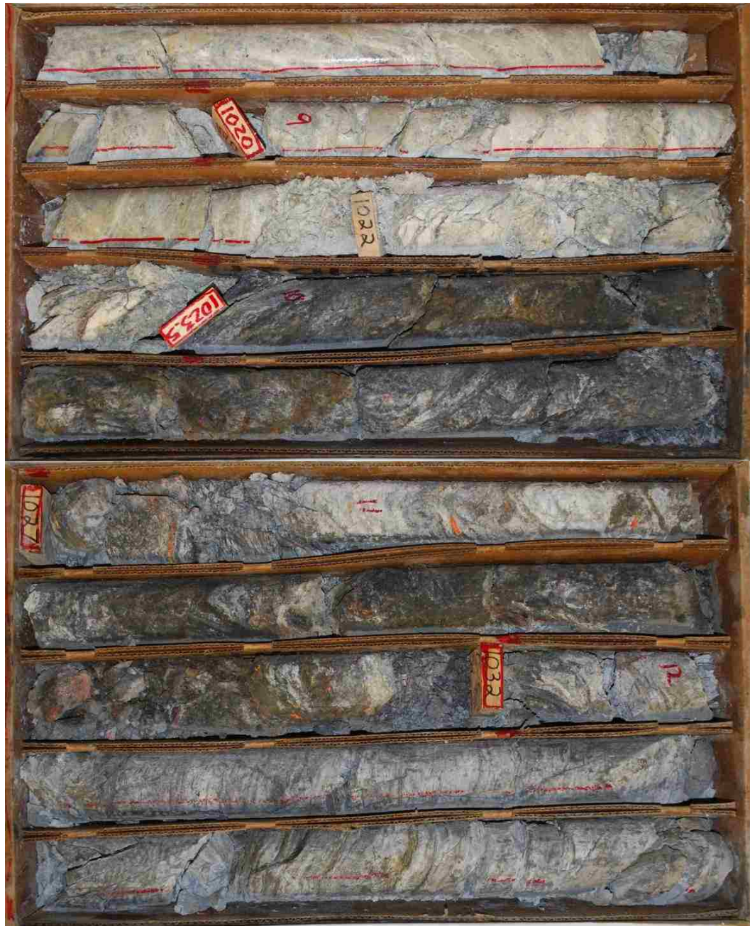
Figure 47. An interval of type II mineralization from drill hole 08-GC-035. Strong bleaching occurs above the mineralized zone, starting at 997 and continuing to 1023, unlike the type I mineralization which generally has little to no bleaching. The bleached zone is not mineralized, grades <0.001 oz/t Au. High-grade mineralization starts abruptly in an argillized gouge zone with abundant sooty pyrite; 1023'-1027' grades 1.645 oz/t and 1027'-1032' averages 1.185 oz/t. There is some disseminated mineralization extending below the fault and 1032'-1037' averages 0.285 oz/t; below mineralization and alteration decline rapidly and 1037'-1042' averages 0.0375 oz/t, 1042'-1045.3' averages 0.005 oz/t (63.5 mm diameter core).
