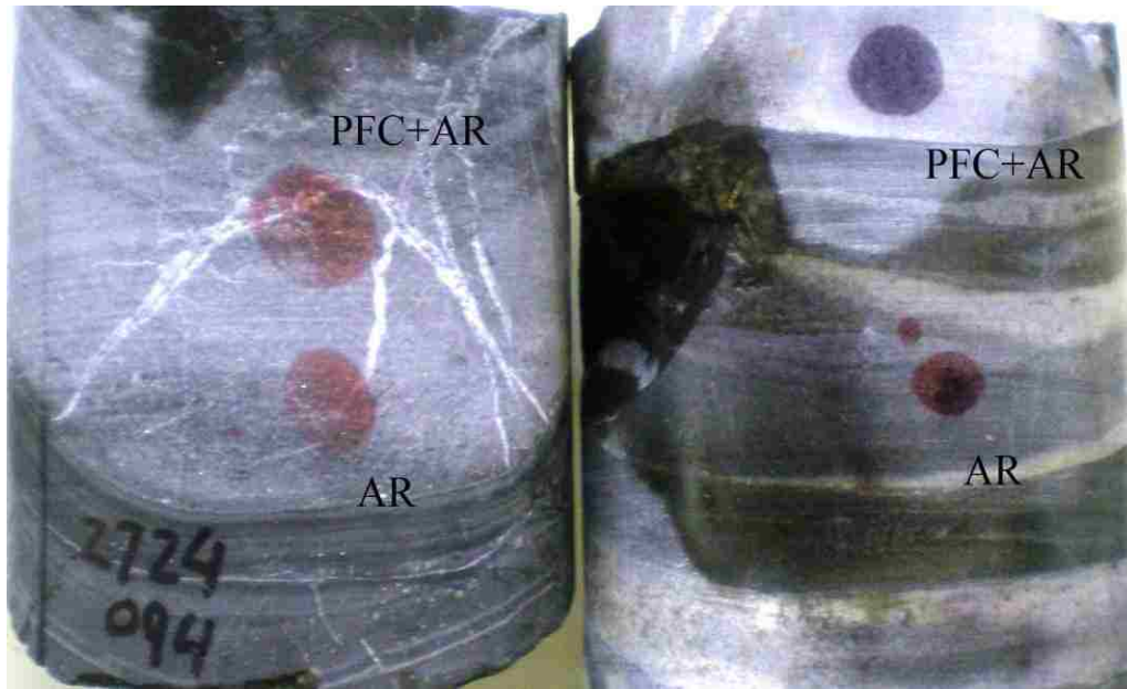
Figure 48. Staining results on limestone inter-bedded with siliceous carbonaceous mudstone and argillaceous mudstone (left and right respectively). The upper spot is 50/50 mixture of potassium ferricyanide and Alizarin red S, the lower spot is only a solution of Alizarin red S, both in a 2% HCl solution. The limestone inter-bedded with siliceous carbonaceous mudstone on the left stains red indicating no iron in the carbonate. The limestone inter-bedded with argillaceous mudstone on the right stains purple indicating the presence of iron in the carbonate (63.5 mm diameter core).
