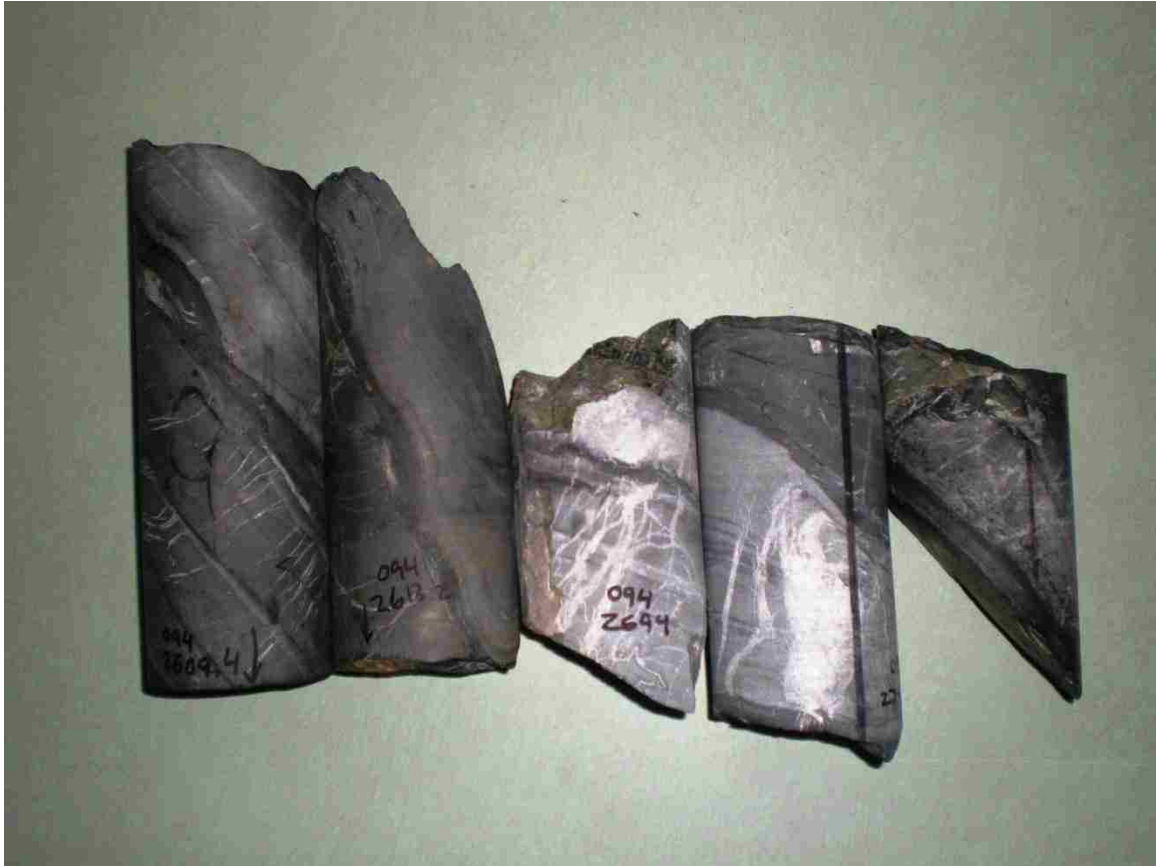
Figure 14. Samples, spanning 150 feet of core, composed of siliceous carbonaceous mudstone inter-bedded with limestone from one interval in core representing one clast. Bedding angles vary from near perpendicular to near parallel to core axis. This change in bedding orientation is likely due to folding within the clast of siliceous carbonaceous mudstone. Changes in bedding orientation may vary from clast to clast but also may be variable within one clast (63.5 mm diameter core).
