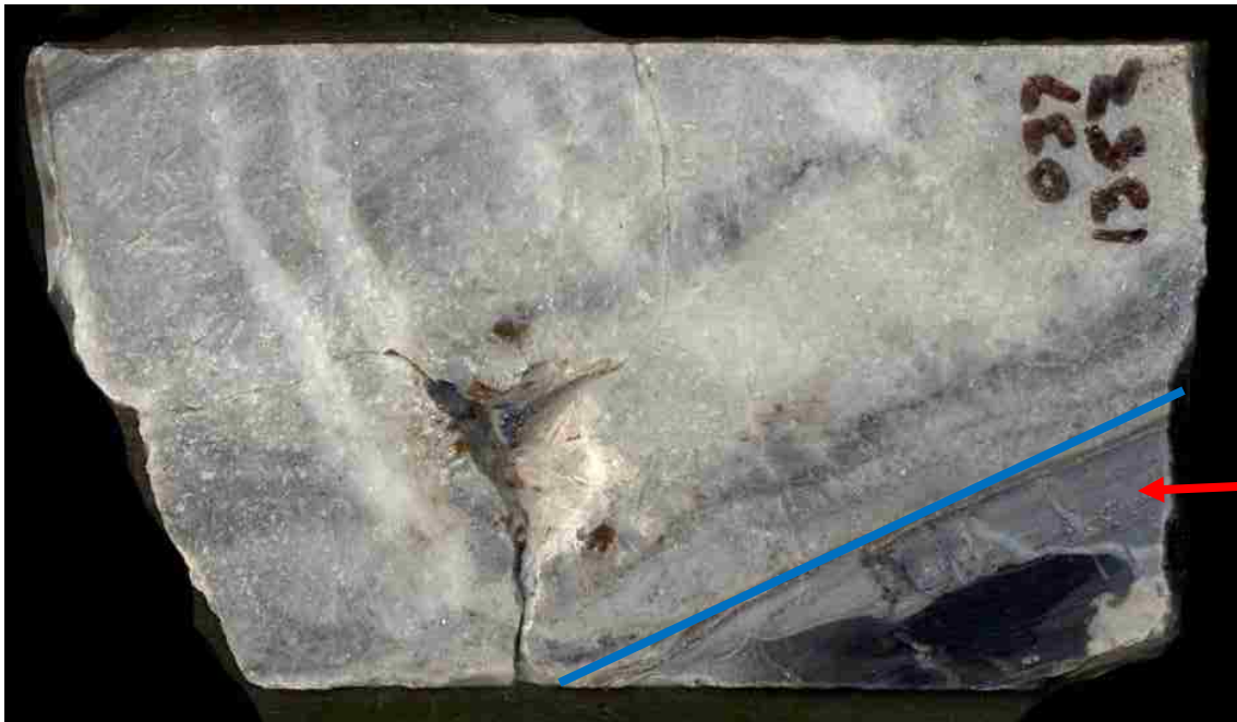
Figure 27. A sample of calc-silicate altered limestone inter-bedded with siliceous carbonaceous mudstone. The dominant calc-silicate mineral is wollastonite (white/gray) with minor amounts of vesuvianite (brown). The siliceous carbonaceous mudstone bed adjacent to the calc-silicate altered limestone bed (right of blue line) has been bleached (red arrow) (63.5 mm diameter core).
