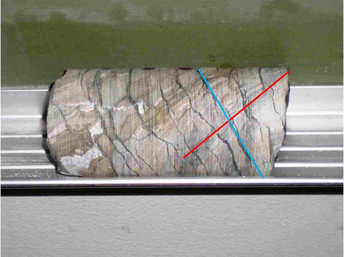
Figure 18. A sample of argillaceous limestone, locally known as the Powder Hill Limestone with weak calc-silicate alteration. The bedding (red line) is cut by a later well developed cleavage fabric (blue line) which is common in this unit. The cleavage planes cause minor offset in the limestone beds (63.5 mm diameter core).
