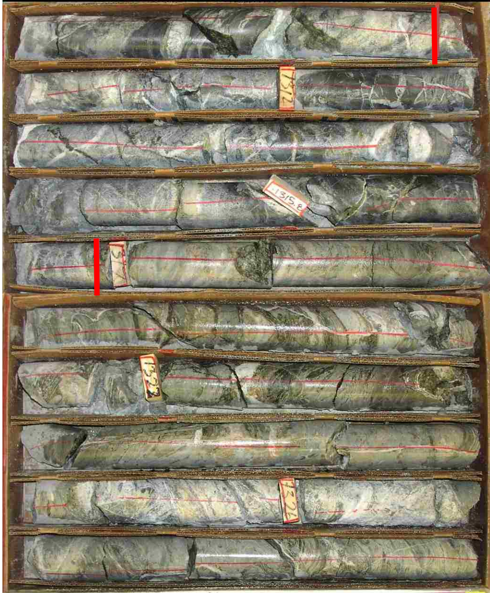
Figure 26. A small clast of limestone inter-bedded with siliceous carbonaceous mudstone (1311'-1317' between red lines) in a matrix of argillaceous mudstone and limestone. The argillaceous mudstone and limestone are strongly calc-silicate altered while the clast composed of the limestone inter-bedded with the siliceous carbonaceous mudstone is not (63.5 mm diameter core).
