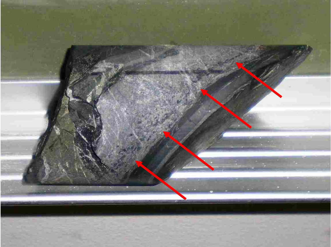
Figure 11. A sample of limestone turbidite (gray bed) with a basal conglomerate of rip-ups from the underlying siliceous carbonaceous bed (red arrows). The bed pictured is over-turned, however, other beds in the same drill core have normal bedding indicators. It is unclear if this is a result of internal folding of the clast or whether the clast is over-turned (63.5 mm diameter core).
