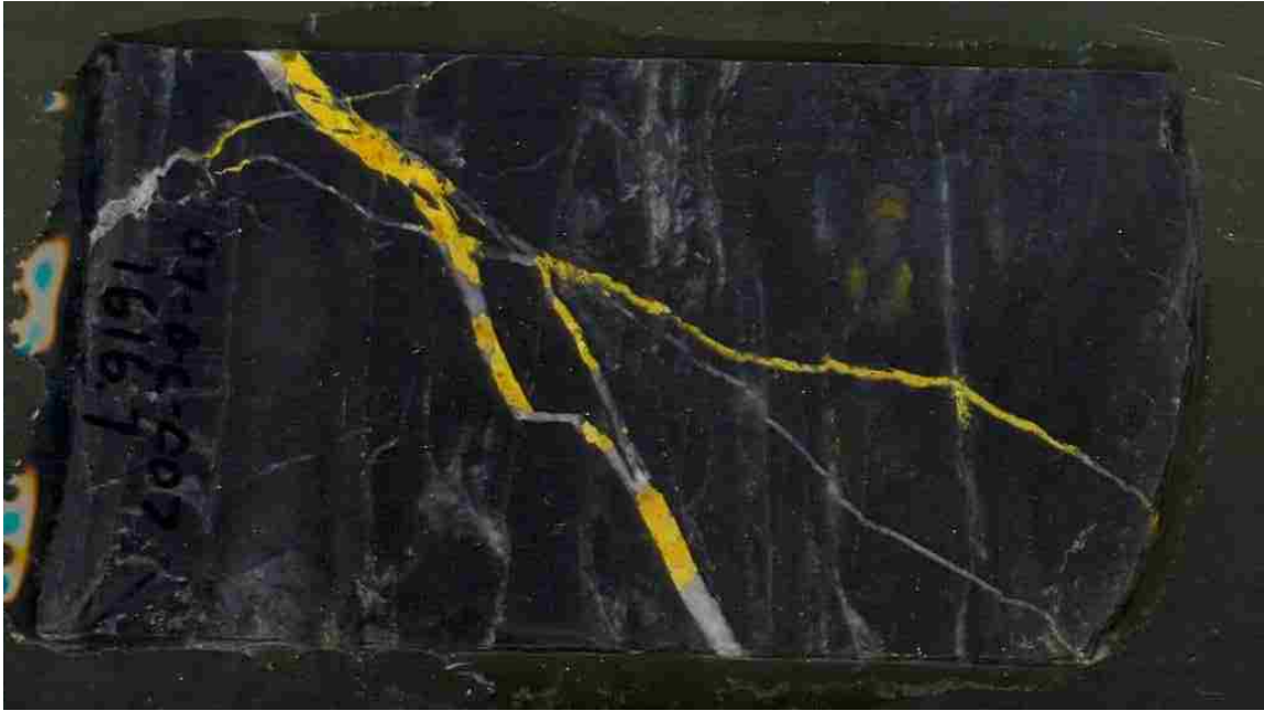
Figure 37. A sample of siliceous carbonaceous mudstone with late veins containing calcite (white) and orpiment (yellow). The sample comes from just above a mineralized zone in drill hole 07-GC-007 associated with the Getchell parallel fault in the hanging wall on Cross Section B.
