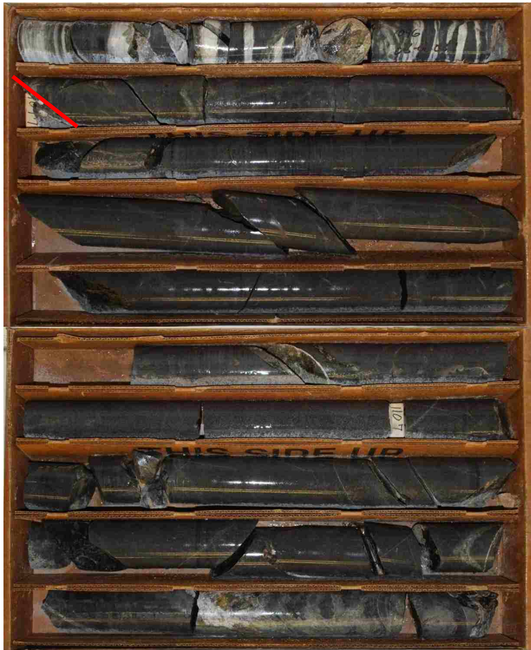
Figure 23. A contact (red line) between a section of argillaceous mudstone inter-bedded with limestone (above) with a diabase dike (below). The diabase is very fine grained and dark gray to green in color (63.5 mm diameter core).
