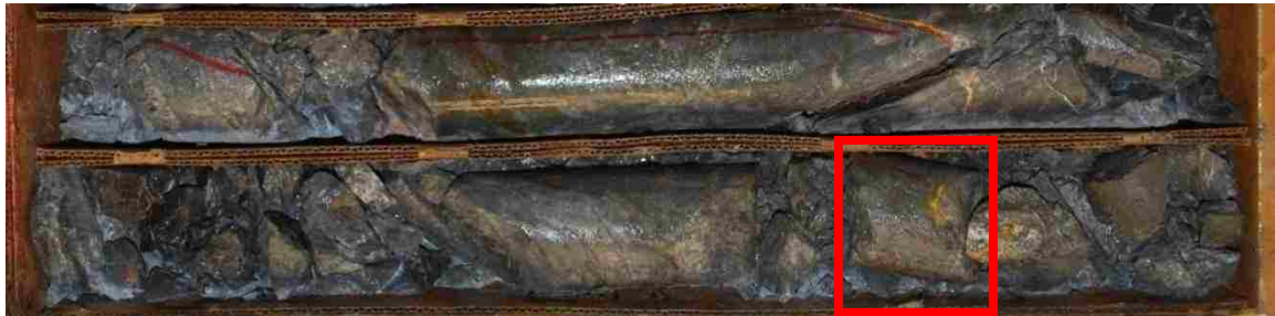
Figure 41. A sample from 1887' (red box) ten feet below the sample above. This sample is from a mineralized five foot section averaging 0.1255 oz/t. The rock is intensely decalcified, and silicified limestone inter-bedded with silicious carbonaceous mudstones with weak realgar mineralization. XRD spectrum indicates that the sample is dominantly quartz with lesser kaolinite, realgar, marcasite and pyrite (63.5 mm diameter core).
