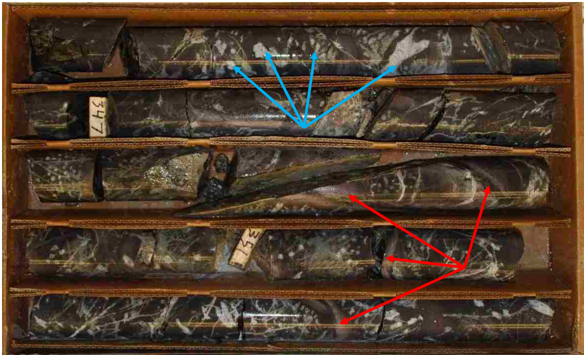
Figure 22. A section of vesiculated Upper Basalt which caps the stratigraphy in the study area. The vesicles have been filled with calcite (blue arrows). Several pillow margins are also visible (red arrows) (63.5 mm diameter core).
