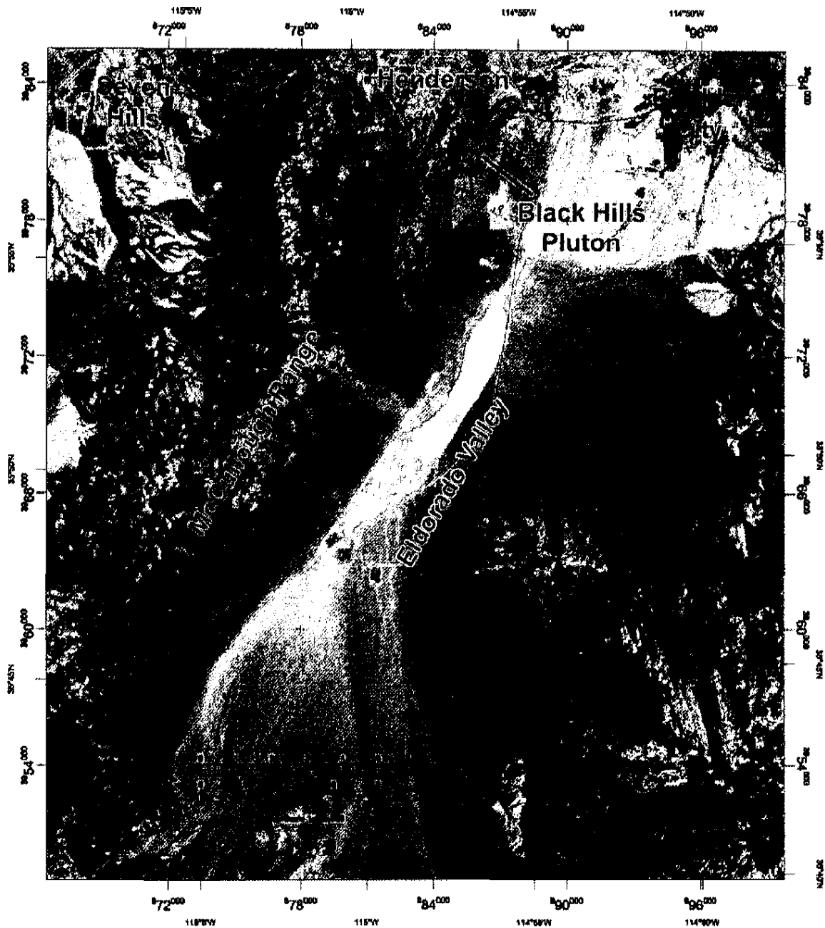
Figure 25. Landsat 7 ETM+ false color image with band ratios 1/7, 3/1, and 7/5 applied to RGB respectively (GLCF, 2005). Values in the image occupy a very narrow pixel range, so that only yellow and pink colors are displayed and differences in lithology are difficult to determine.
