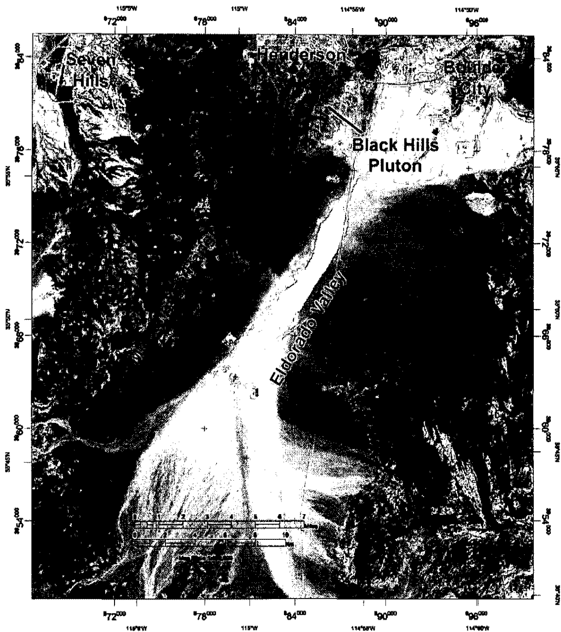
Figure 23. Selected bands of a Landsat image can be assigned RGB colors to produce a false color image (GLCF, 2005). In this case, RGB are applied to bands 3, 2, and 1 respectively to produce an image that approximates true color (Landsat 321 image).
