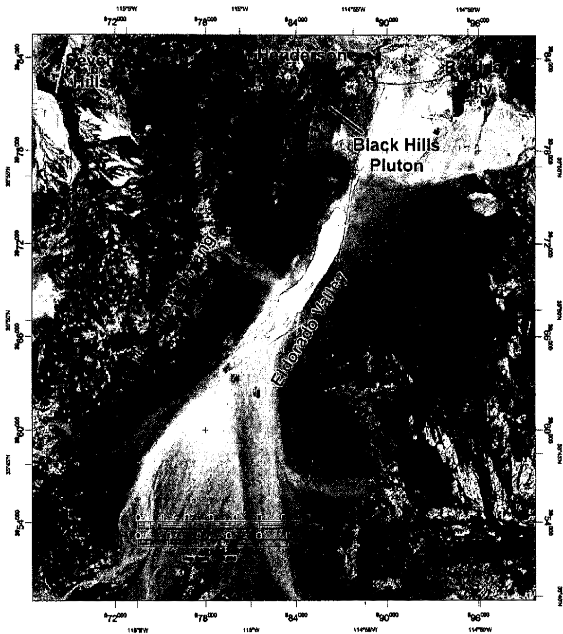
Figure 20. Image showing raw Landsat 7 ETM+ data from band 5 (GLCF, 2005), which has a median wavelength of \sim 1.650 \mu\text{m} (Jensen, 2000). This corresponds to a portion of the NIR spectrum.
