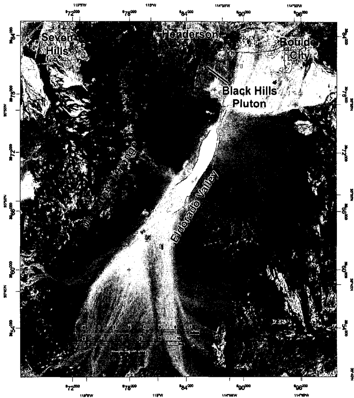
Figure 19. Image showing raw Landsat 7 ETM+ data from band 4 (GLCF, 2005), which has a median wavelength of \sim 0.830 \mu\text{m} (Jensen, 2000). This corresponds to a portion of the NIR spectrum.
