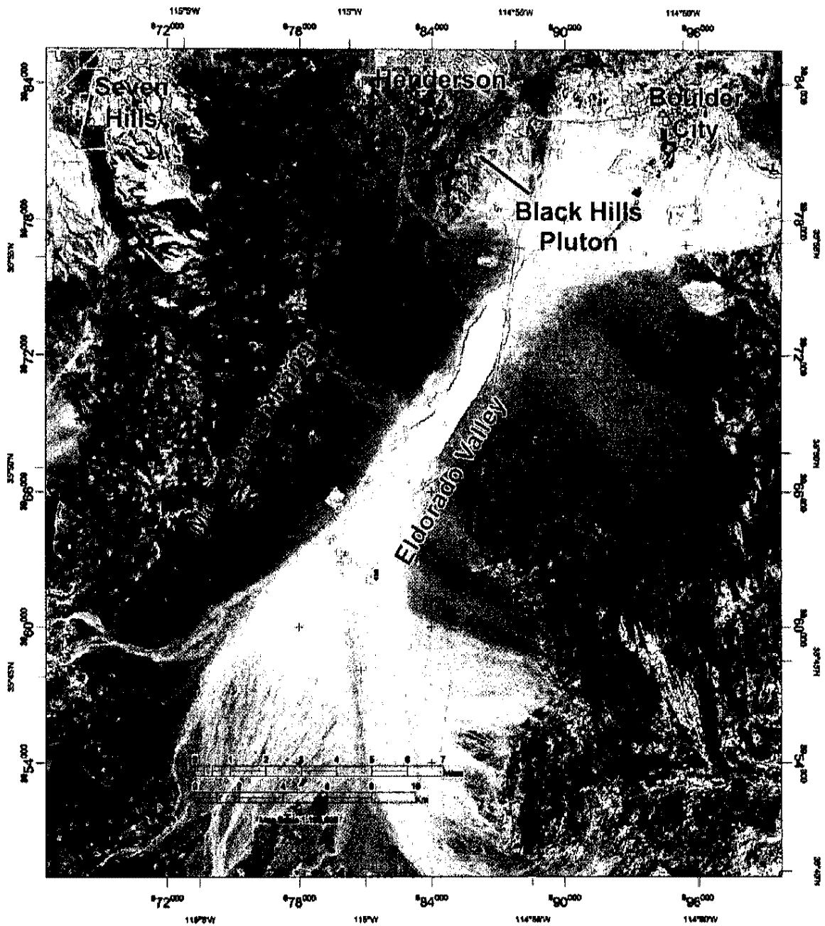
Figure 16. Image showing raw Landsat 7 ETM+ data from band 1 (GLCF, 2005), which has a median wavelength of \sim 0.485 \mu\text{m} (Jensen, 2000). This roughly corresponds to blue light in the visible spectrum.
