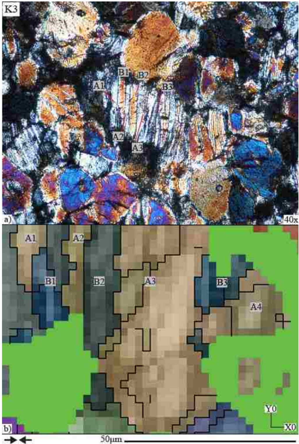
Figure 3.12. Kink band domains for grain K3 in optical and orientation map image. a) optical image of grain K3; b) orientation map image of grain K3.
