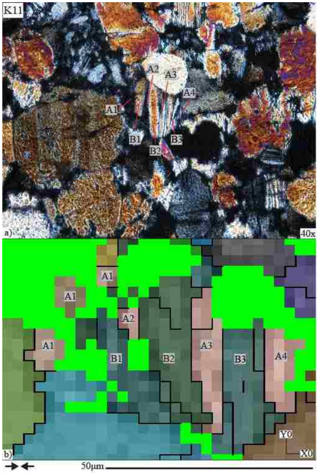
Figure 3.20. Kink band domains for grain K11 in optical and orientation map image. a) optical image of grain K11; b) orientation map image of grain K11.
