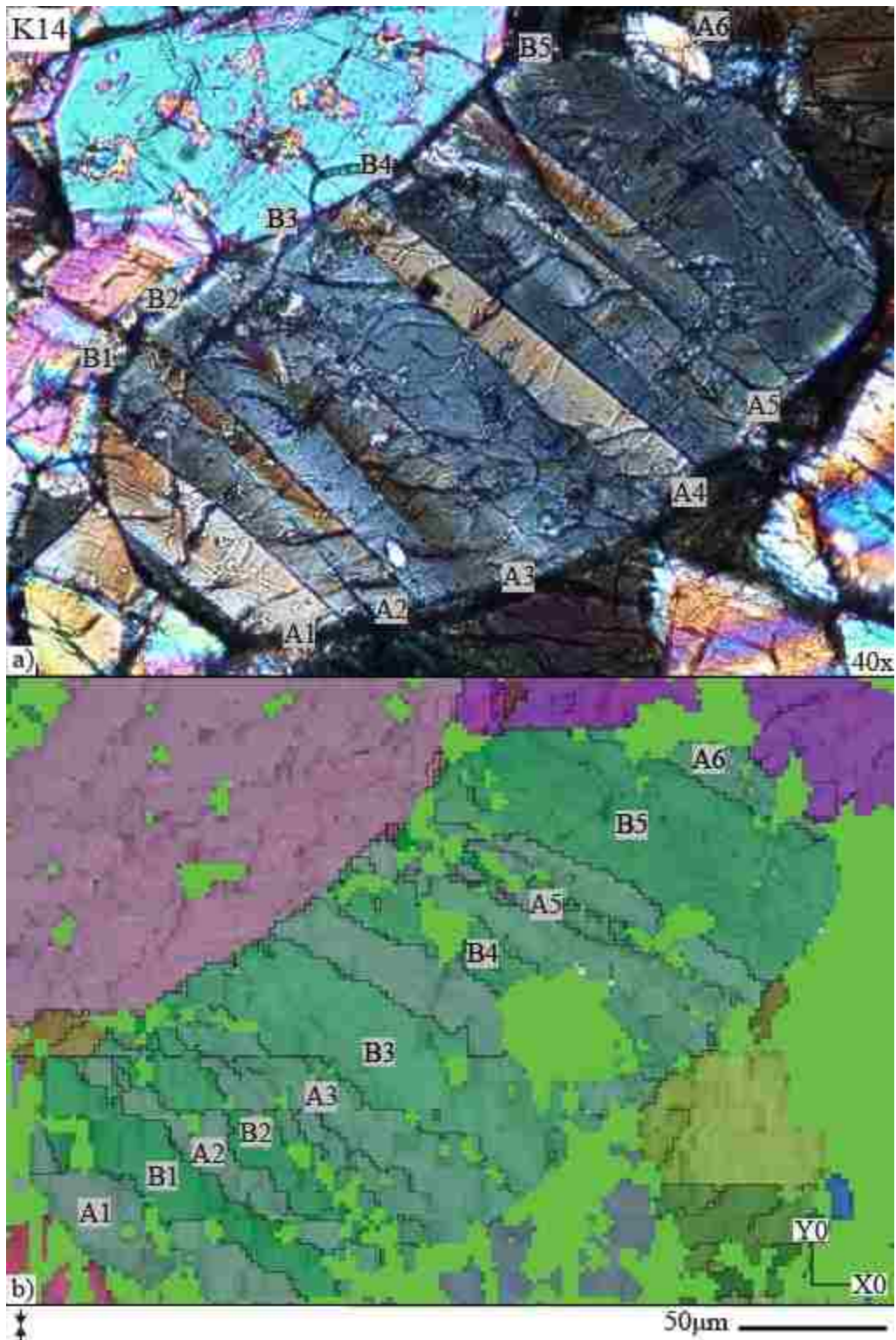
Figure 3.23. Kink band domains for grain K14 in optical and orientation map image. a) optical image of grain K14; b) orientation map image of grain K14.
