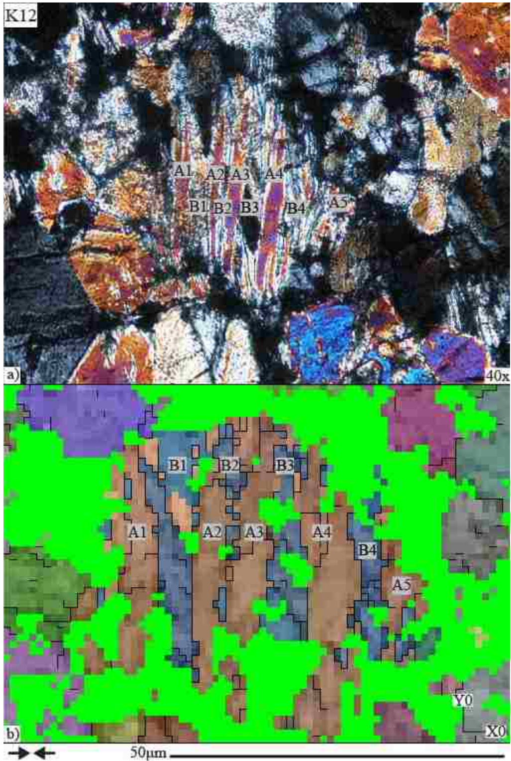
Figure 3.21. Kink band domains for grain K12 in optical and orientation map image. a) optical image of grain K12; b) orientation map image of grain K12.
