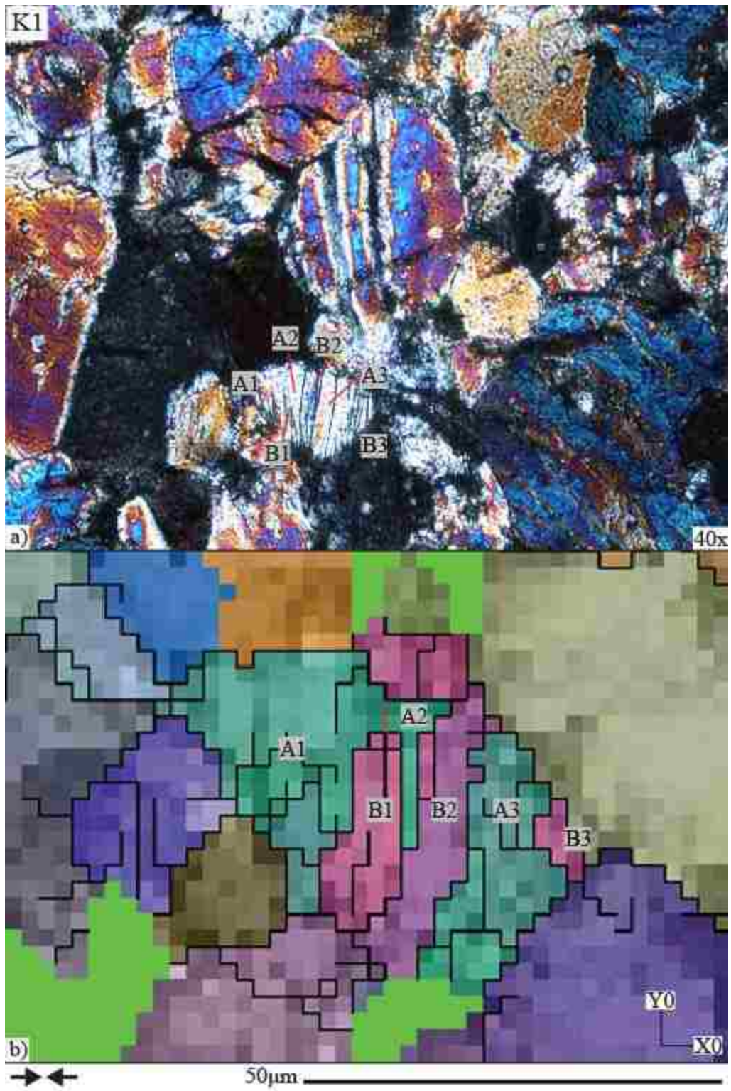
Figure 3.10. Kink band domains for grain K1 in optical and orientation map image. a) optical image of grain K1; b) orientation map image of grain K1.
