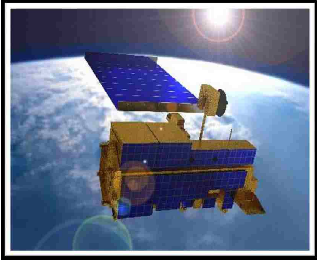
NASA's EOS Terra satellite has a spatial resolution of ~1km/pixel and an absolute accuracy of 1K ( http://terra.nasa.gov/About/ ).
