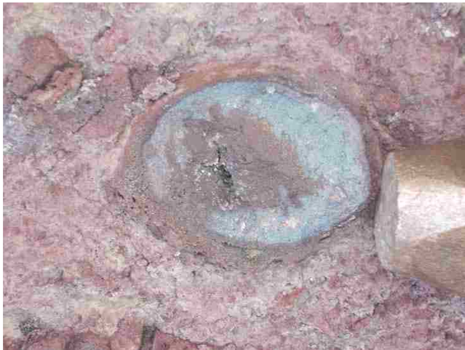
Picture 4: Zoned bomb embedded in welded scoria of the Crater. Bomb displays red vesicular core and blue degassed rim.
