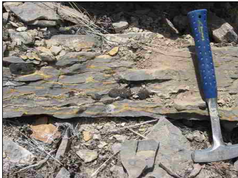
Figure 11: SP 186. Bioclastic wackestone/packstone (gray) with silty dolomitic partings (weathered to buff yellow). Undulating bedding planes likely from post-depositional compaction.
