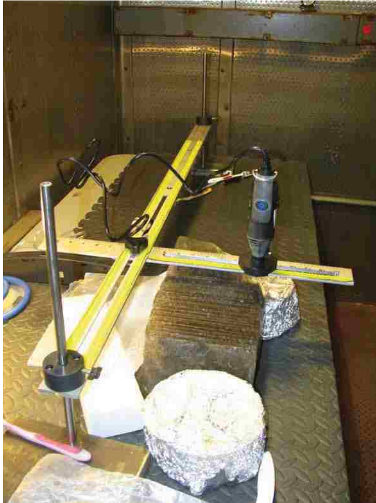
Figure 9. High-resolution isotope sampling device, with partially sampled ice block.
