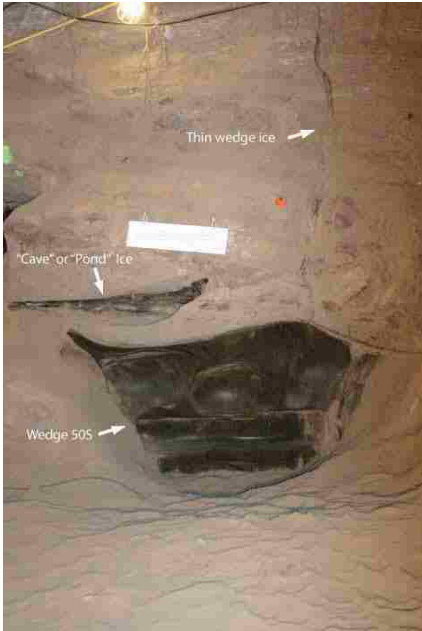
Figure 7. Image of wedge 50S after sampling, with interpretive sign for scale. "Cave" or "pond" ice, as well as wedge 50S and the thin wedge ice are indicated with arrows. The rectangular recess is the location of the sampled wedge ice for this study.
