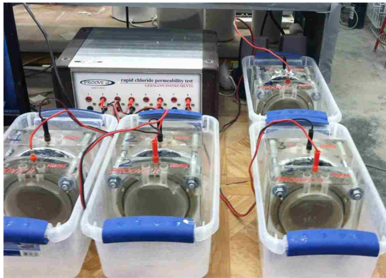
Figure 3.16 RCPT test cell and device
