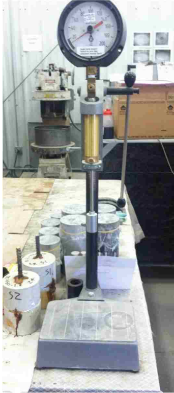
Figure 3.19 Setting time test device for concrete
