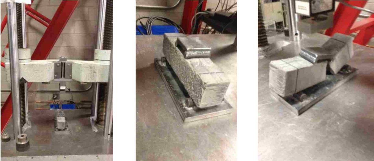
Figure 3.15 Flexural strength test setup
