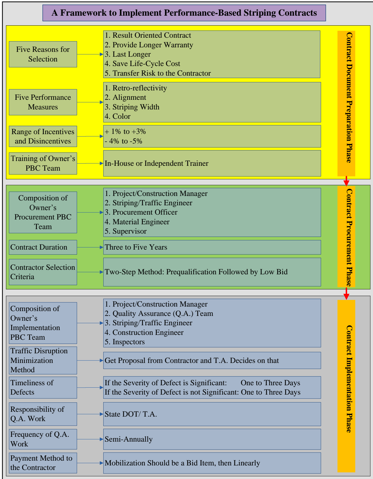
Figure 4.13 Frame work to implement PBC striping contracts
