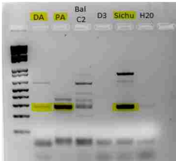
Figure 5.8: Electrophoresis gel ran for PCR products to identify presence of perchlorate reductase (Source: Touro University Laboratory, 2015).
