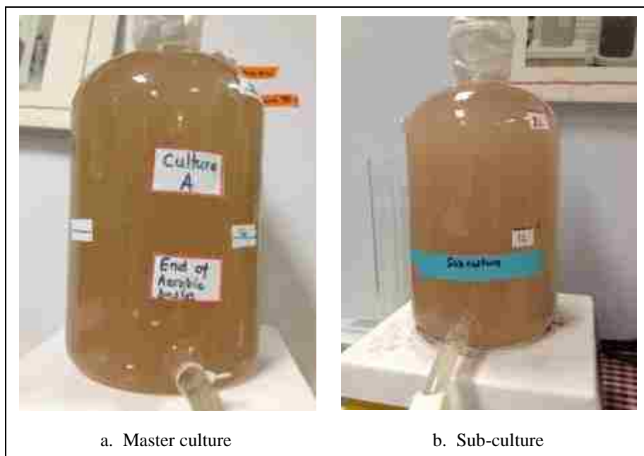
Figure 3.1: Perchlorate-reducing culture (master culture) enriched from returned activated sludge (a) and Sub-culture enriched from the master culture (b).
