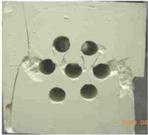
a- Tension Failure (Vertical to sub-vertical fractures)
