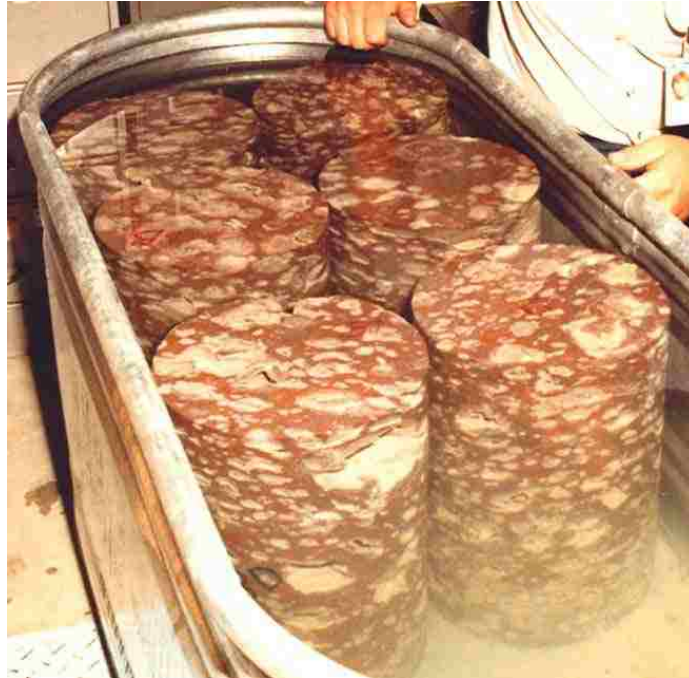
Figure (2.3) Photograph of the Large (267 mm) Diameter Cores from Busted Butte Samples (Rigby 2004)
