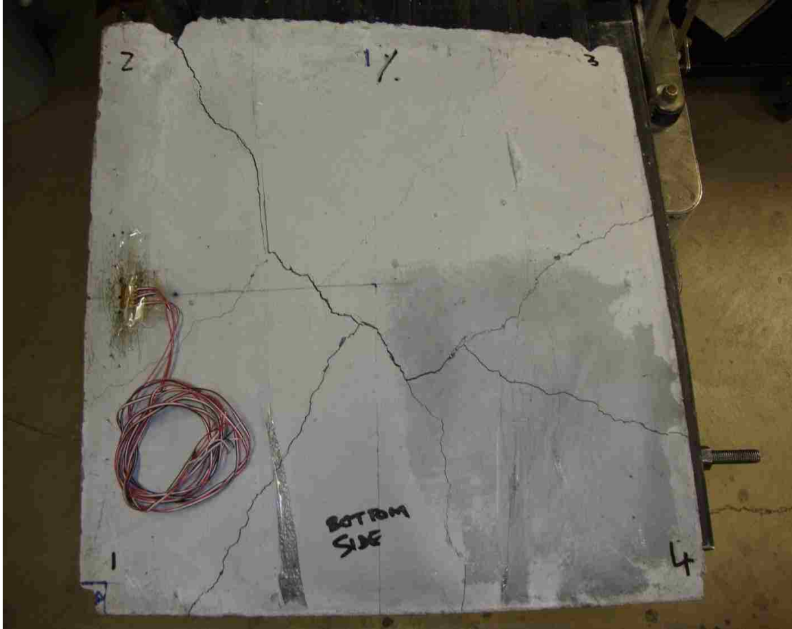
Figure 13.6: Rosette located, at bottom surface, 32 mm (1.25 in.) from the edge of the hyperbolic paraboloid shell
