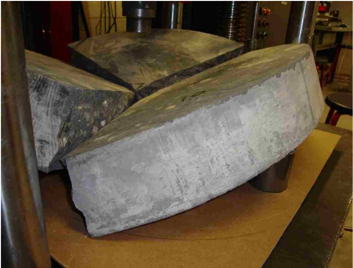
Figure 11.16: Crack and failure patterns for 0% HSSFRC circular plates under a concentrated center load
