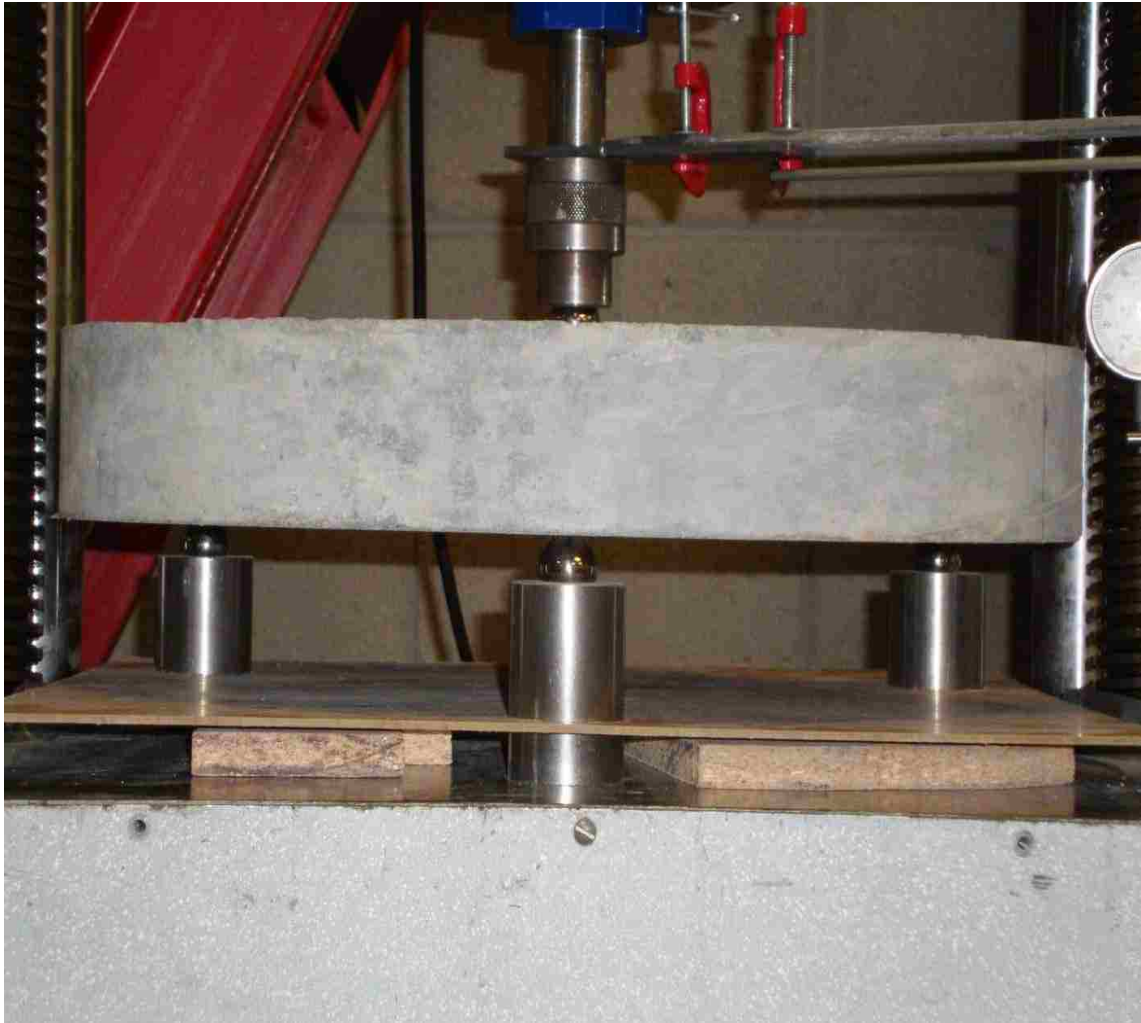
Figure 11.1: HSSFRC circular plate subjected to a transverse concentrated center load
