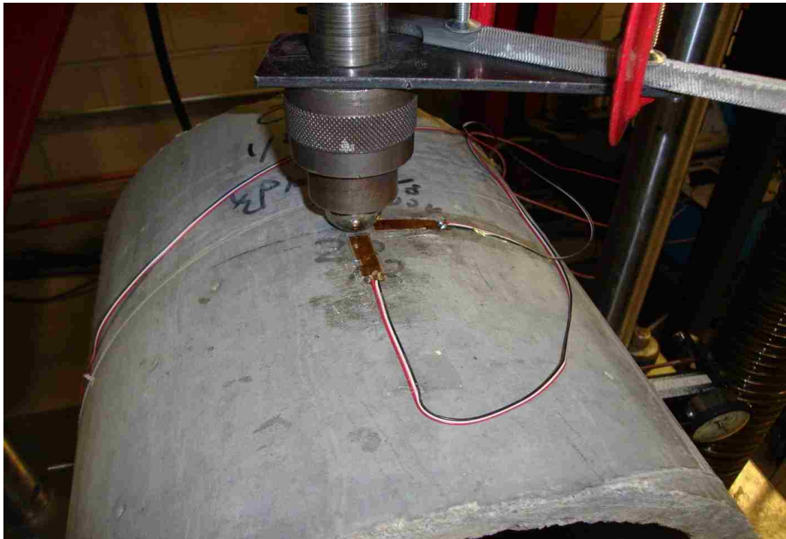
Figure 12.3: N2A-06-10CBE-350/E type strain gages located on the top surface of the circular cylindrical shell and 3 mm (0.125 in.) away from the center point load
