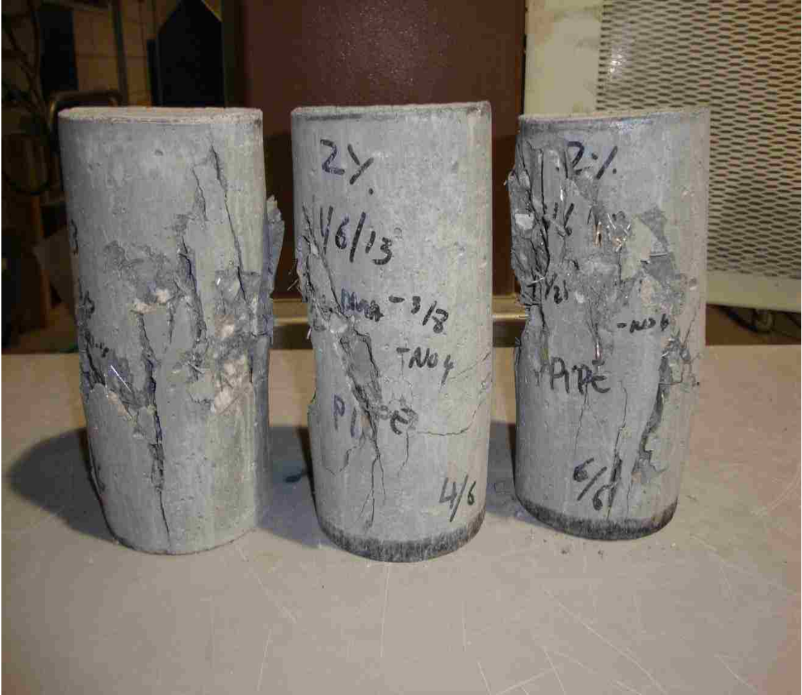
Figure 5.6: Failure mode for 2% HSSFRC cylinders under compression
