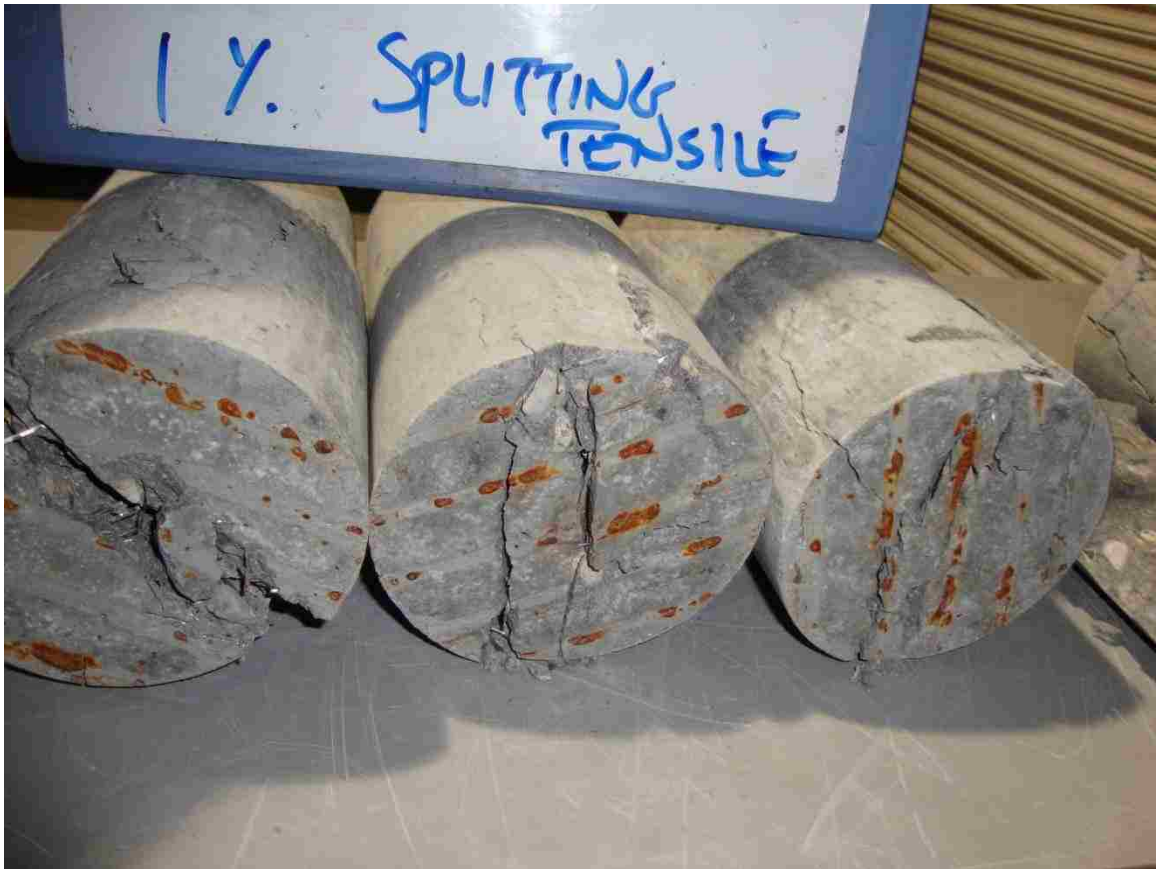
Figure 5.10: Failure mode for 1% HSSFRC cylinders under splitting tensile force
