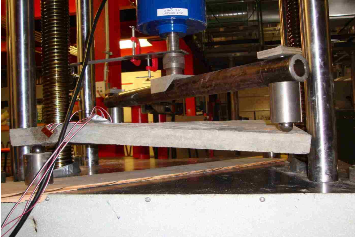
Figure 10.3: 45°- rectangular rosette located on the side of the square plate close to the support point
