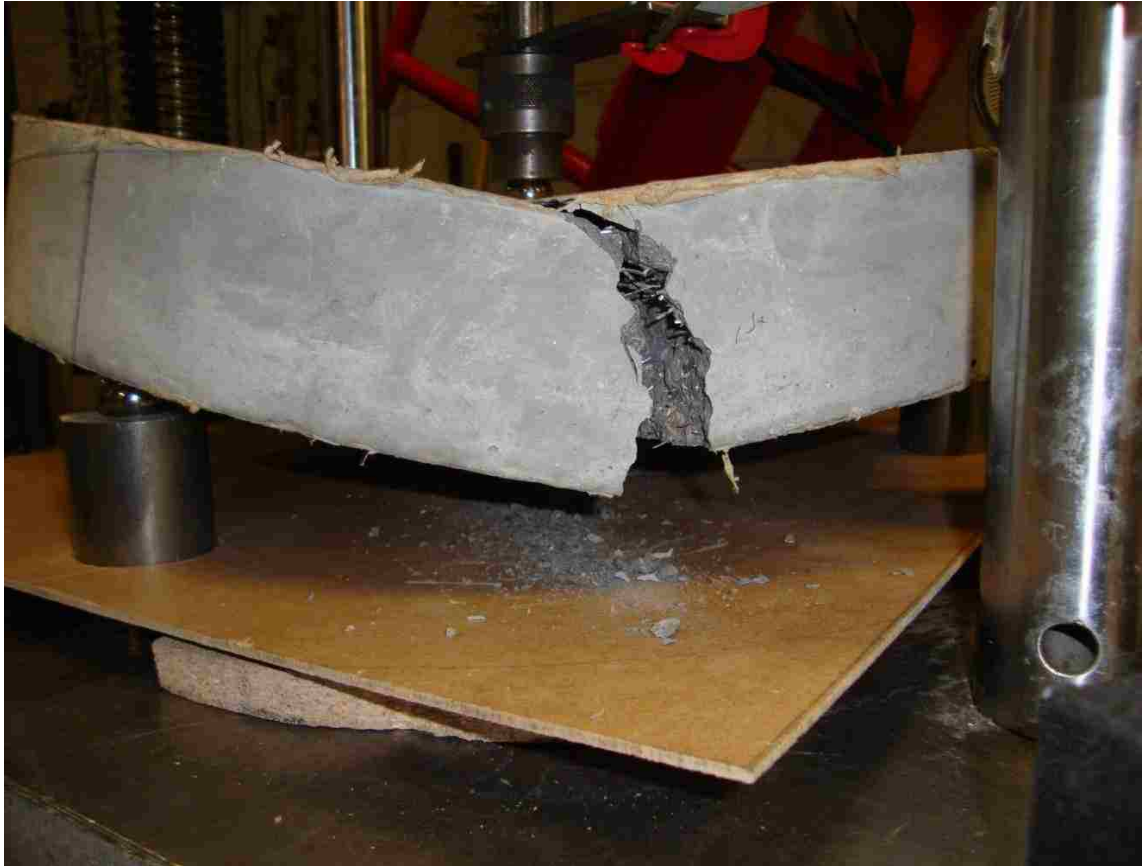
Figure 11.18: Crack and failure patterns for 2% HSSFRC circular plates under a concentrated center load
