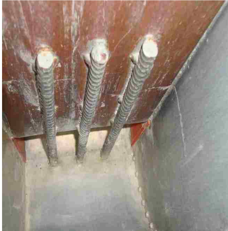
Figure 4.5: Rebar set-up in U-Box test apparatus
