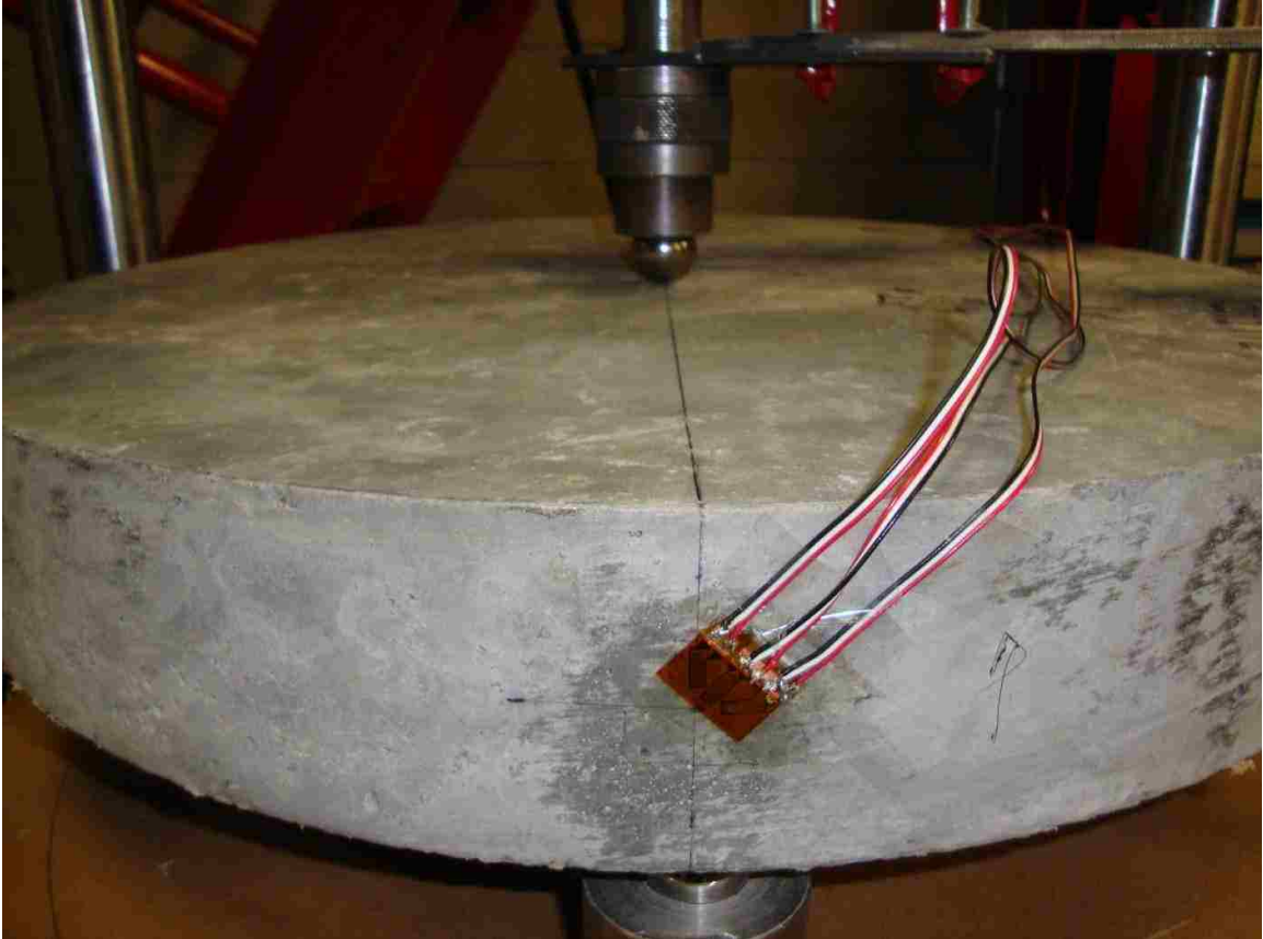
Figure 11.4: 45°- rectangular rosette located at mid depth of the circular plates
