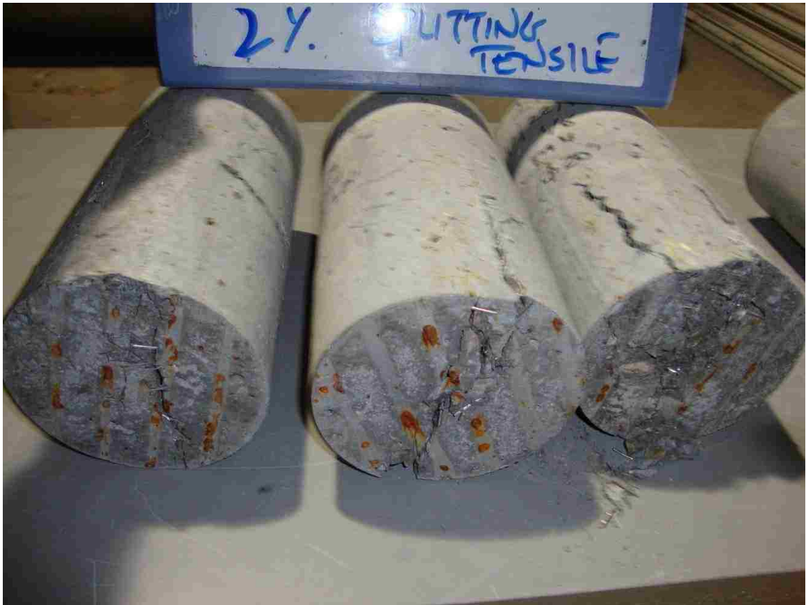
Figure 5.11: Failure mode for 2% HSSFRC cylinders under splitting tensile force
