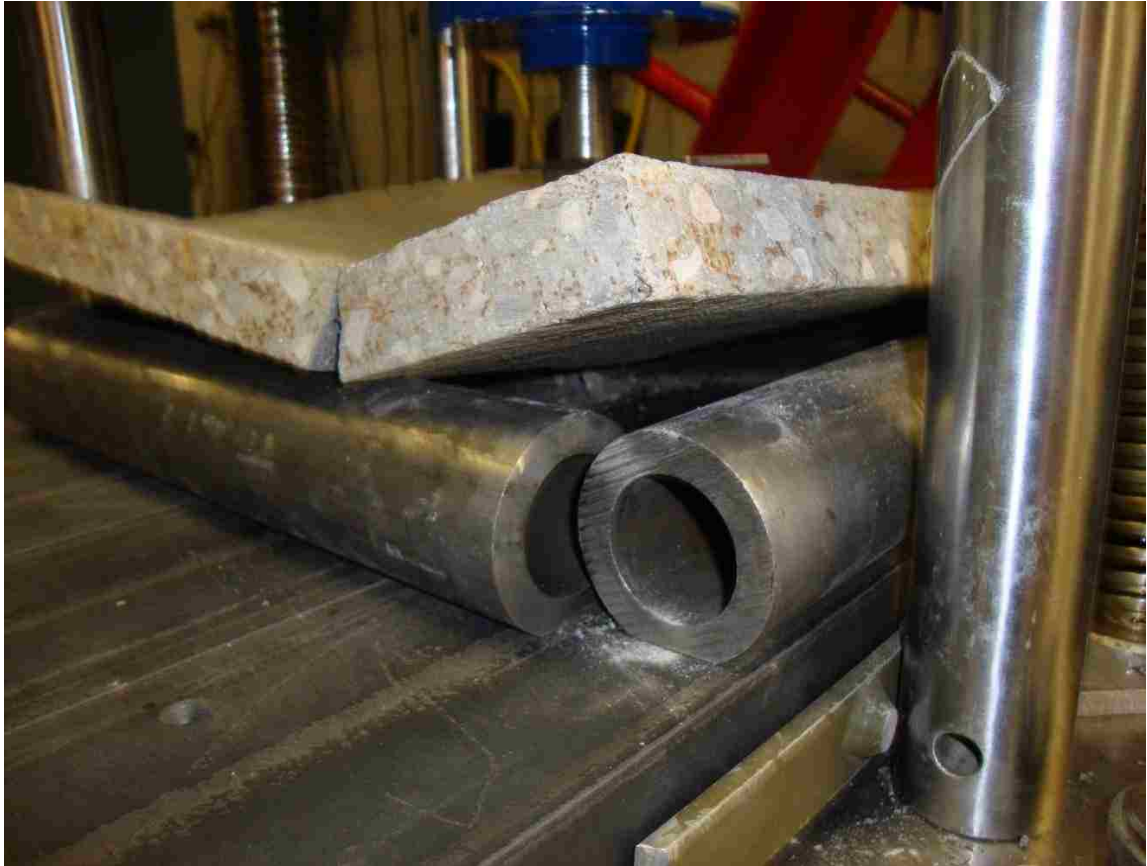
Figure 9.15: Lifting of corners and crack patterns for 2% HSSFRC square plates under center point load
