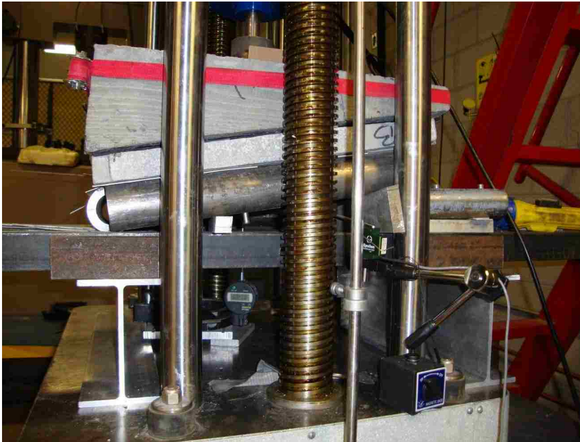
Figure 13.1: Test set up for HSSFRC Hyperbolic paraboloid shell structure subjected to a vertically applied uniformly distributed load, showing the steel supports and silica sand inside the concrete ring
