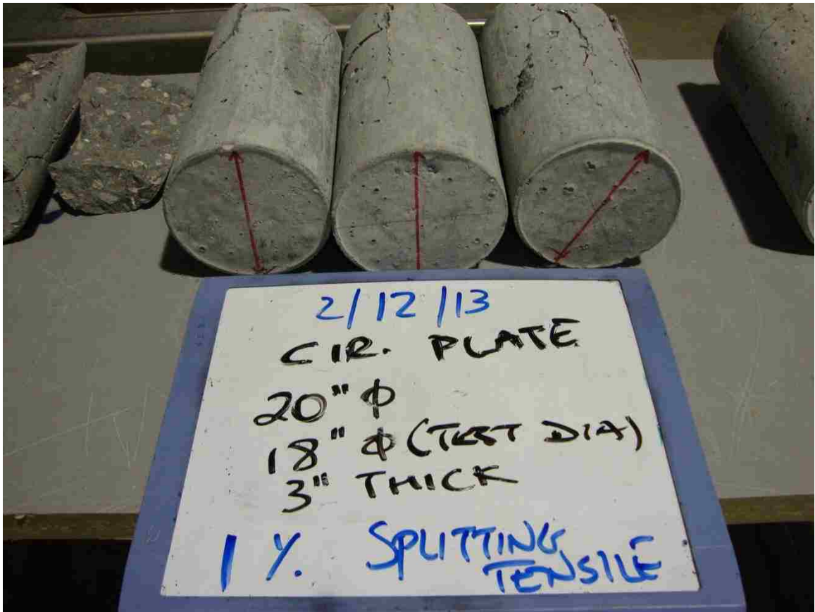
Figure 5.9: Failure mode for 1% HSSFRC cylinders under splitting tensile force
