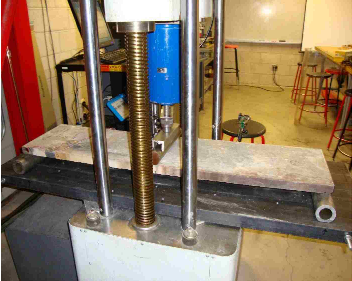
Figure 8.1.1: HSSFRC rectangular plate (48 in. x 12 in.) subjected to a transverse line load at mid span
