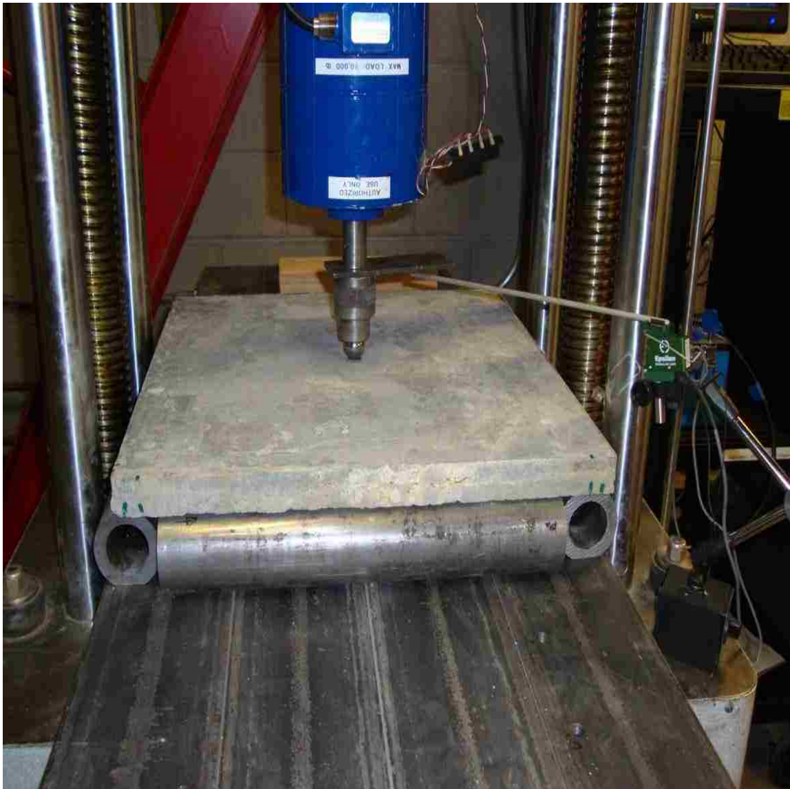
Figure 9.1: HSSFRC square plate subjected to concentrated load at the geometric center
