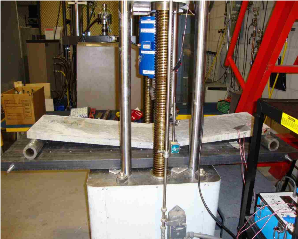
Figure 8.1.7: Support platform for HSSFRC rectangular test specimens, (48 in. x 12 in.)
