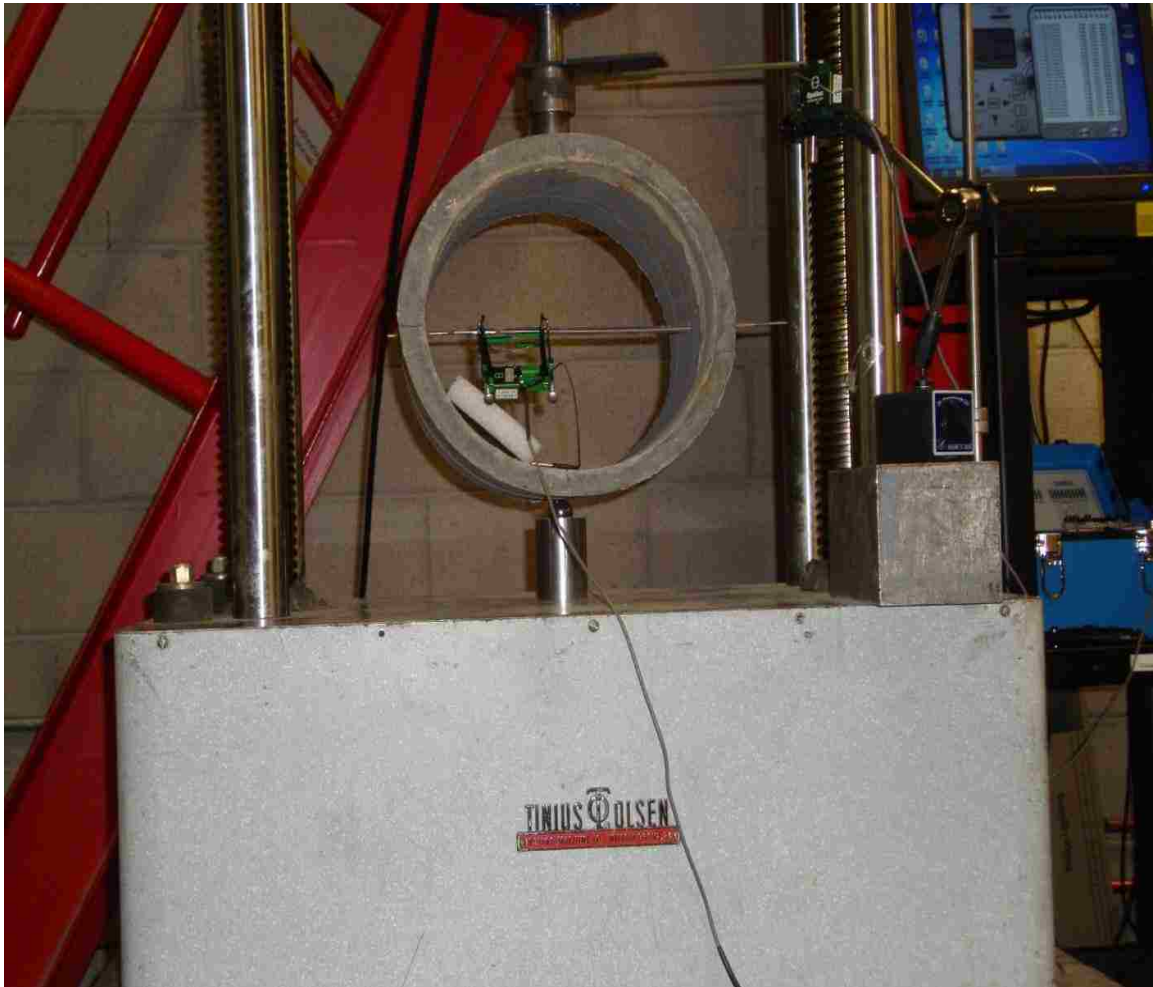
Figure 12.1: HSSFRC circular cylindrical shell subjected to a pinching center load
