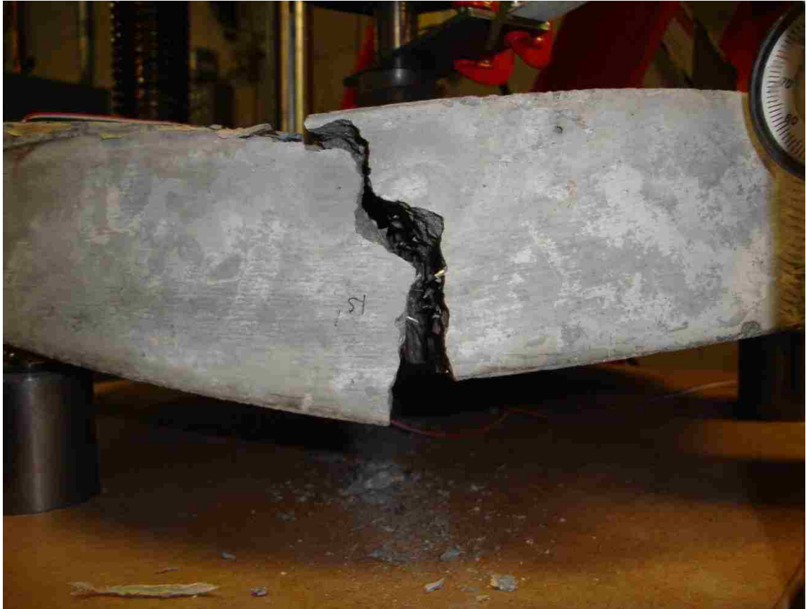
Figure 11.17: Crack and failure patterns for 1% HSSFRC circular plates under a concentrated center load
