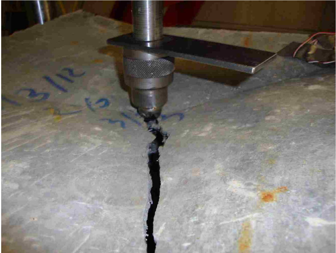
Figure 9.14: Crack sizes and patterns for 2% HSSFRC square plates under center point load
