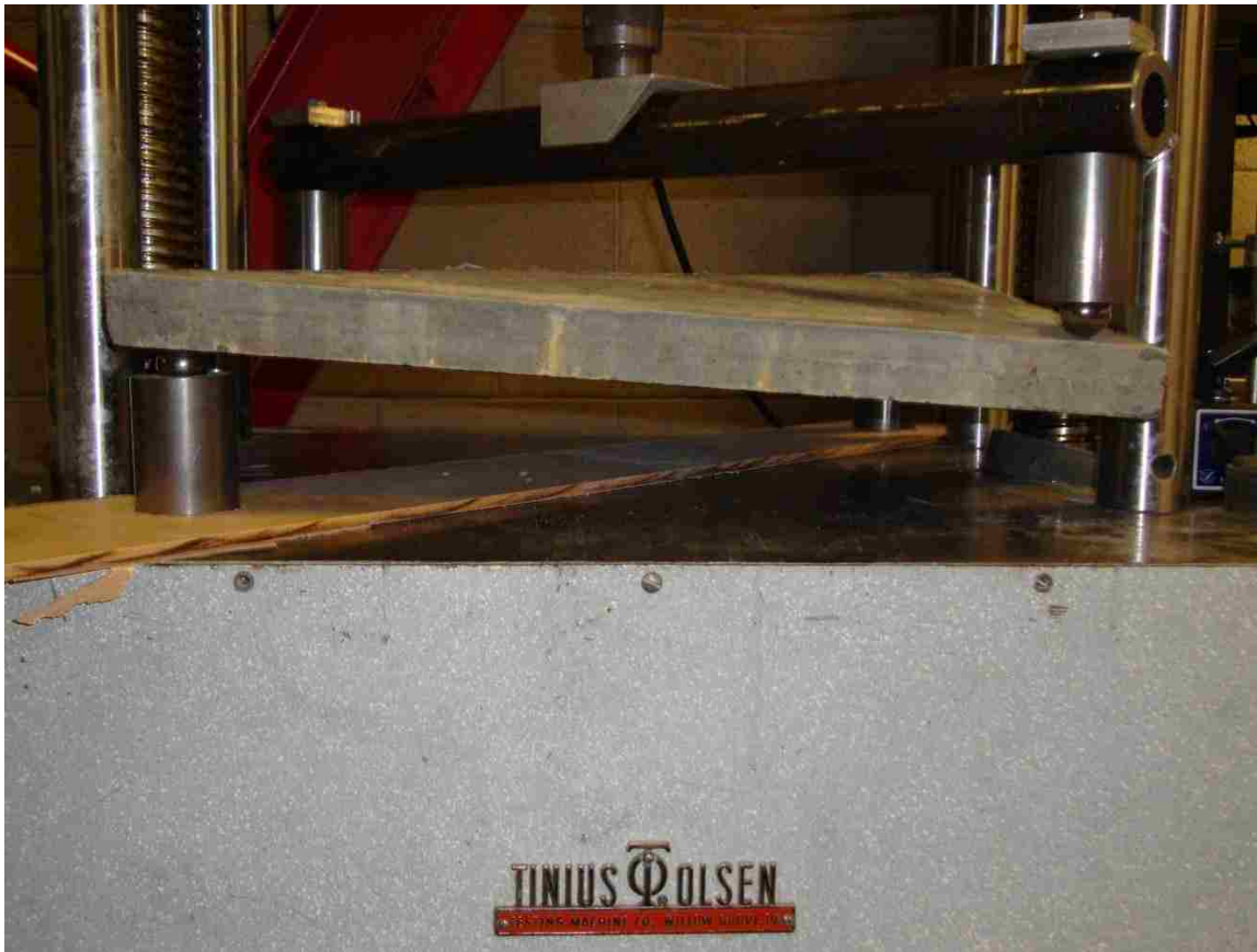
Figure 10.16: Failure and crack patterns for 2% HSSFRC square plates under concentrated opposite corner loads
