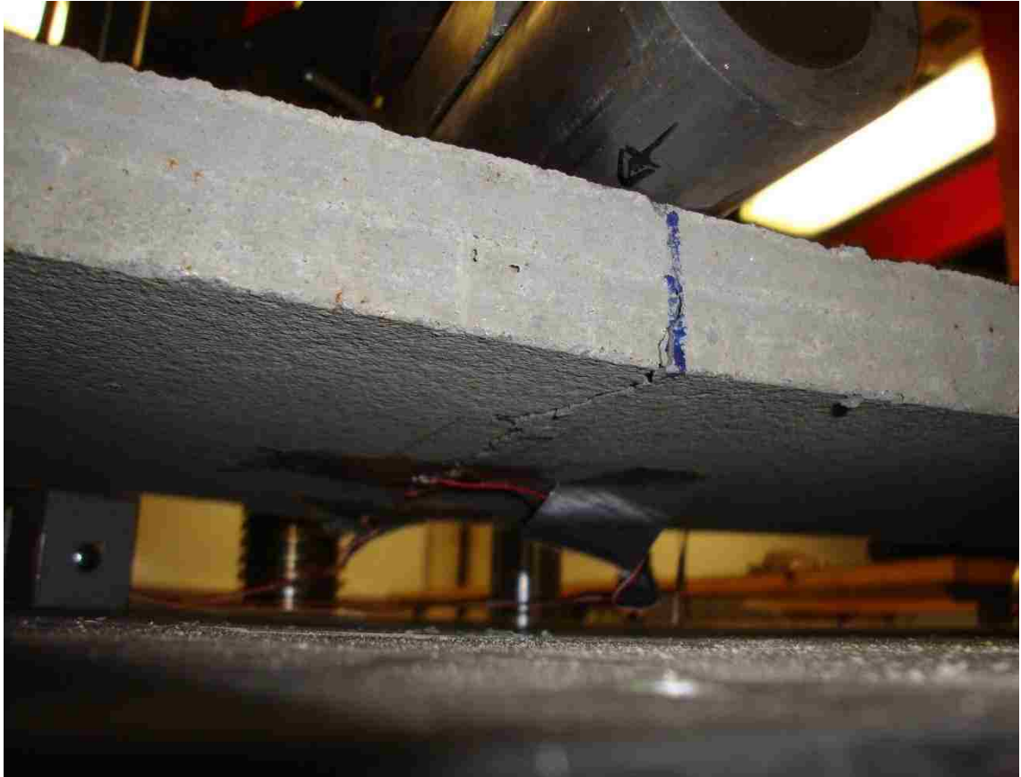
Figure 8.1.14: Failure patterns for long span 2% HSSFRC rectangular plates under transverse line load
