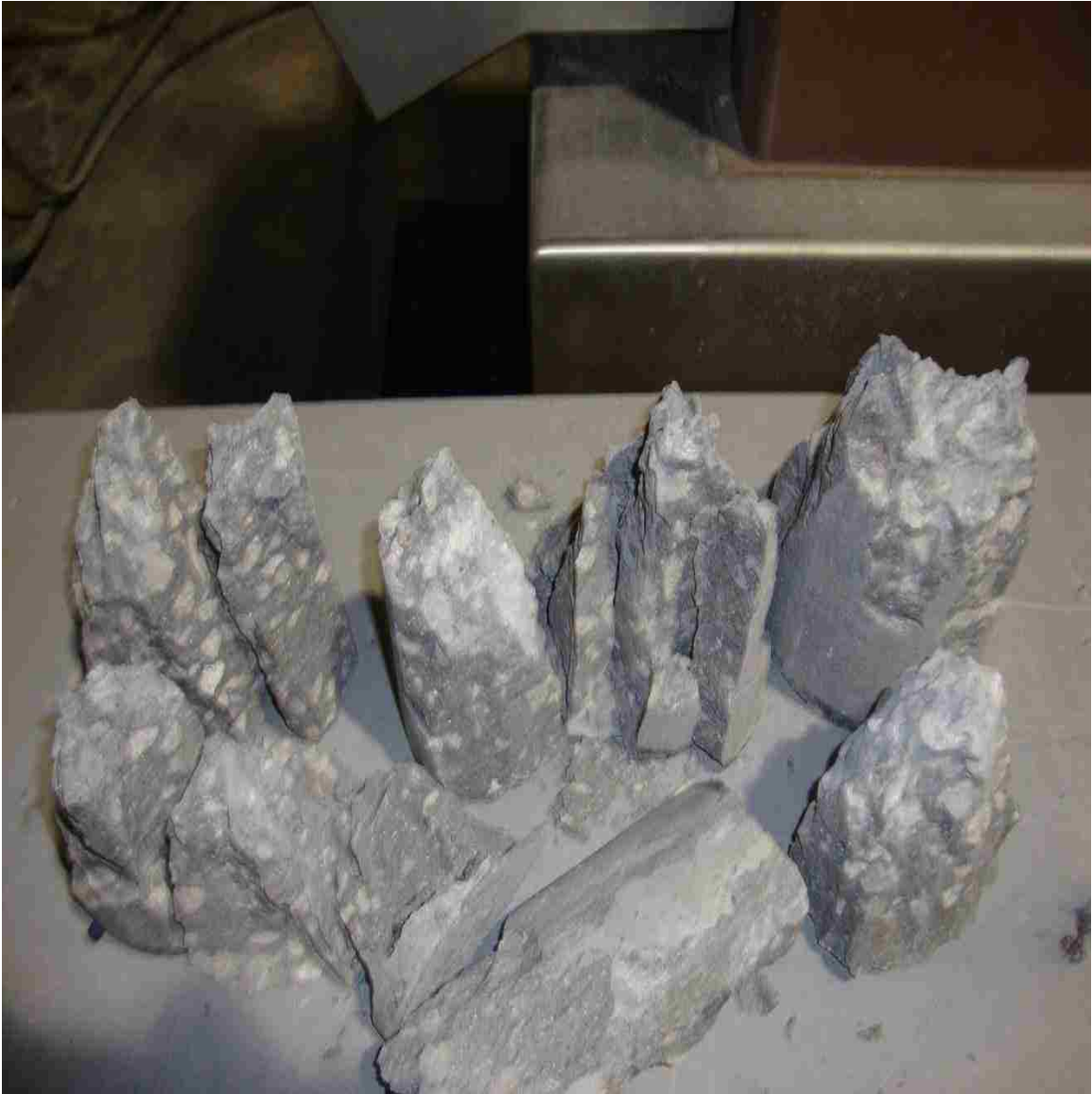
Figure 5.4: Failure mode for 0% HSSFRC cylinders under compression
