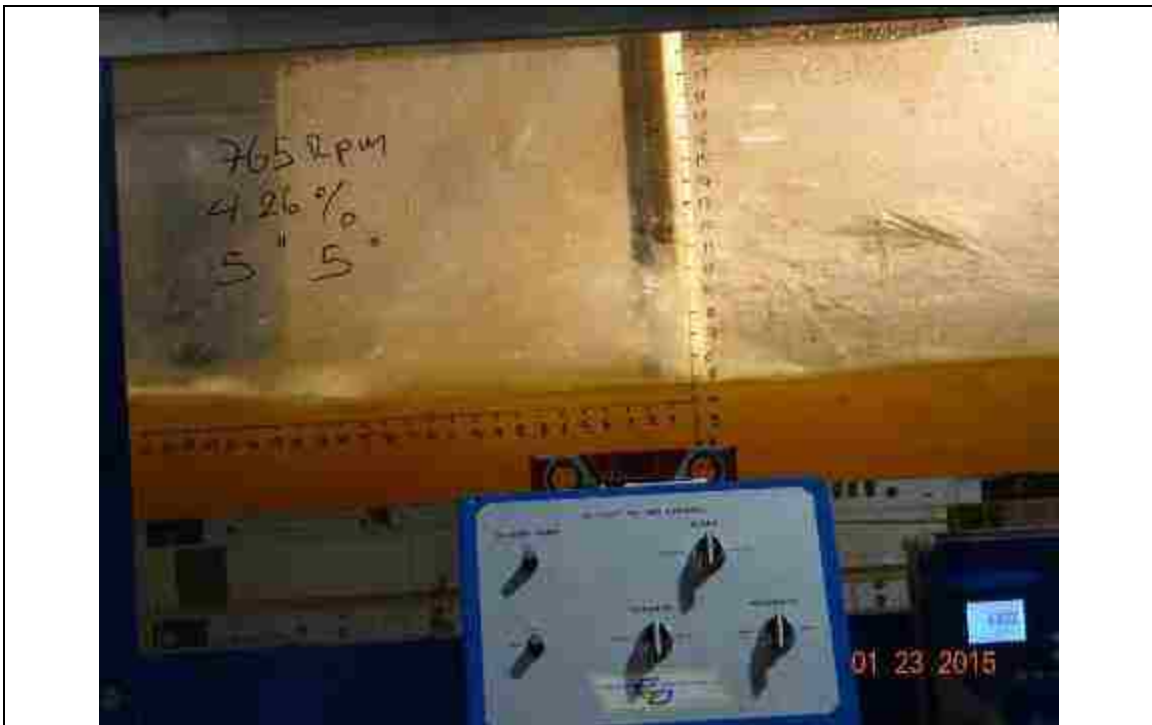
Figure 165. 765 RPM, slope: 4.26%, L_{bb}= 5'' , pitch angle = 5^\circ
