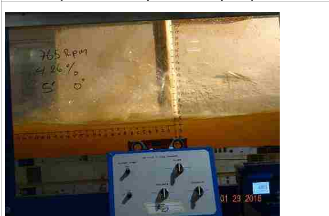
Figure 160. 765 RPM, slope: 4.26%, L_{bb}=5'' , pitch angle = 0^\circ
