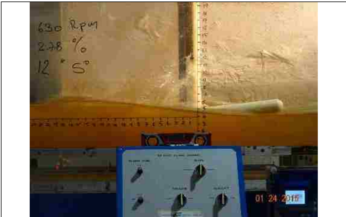
Figure 125. 630 RPM, slope: 2.78%, L_{bb}= 12'' , pitch angle = 5^\circ
