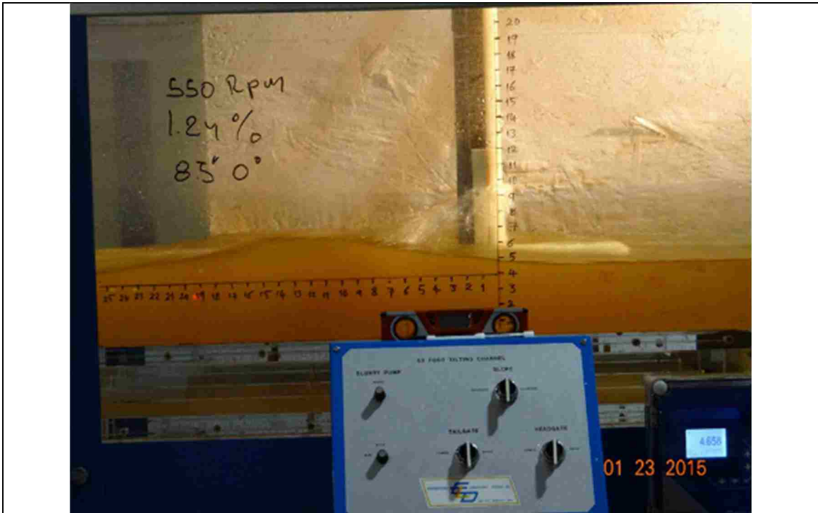
Figure 63. 550 RPM, slope: 1.24%, L_{bb}= 8.5'' , pitch angle = 0^\circ
