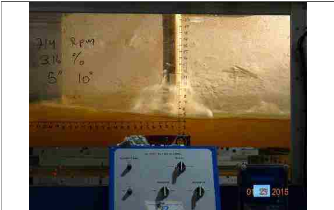
Figure 141. 714 RPM, slope: 3.16%, L_{bb}= 5'' , pitch angle = 10^\circ
