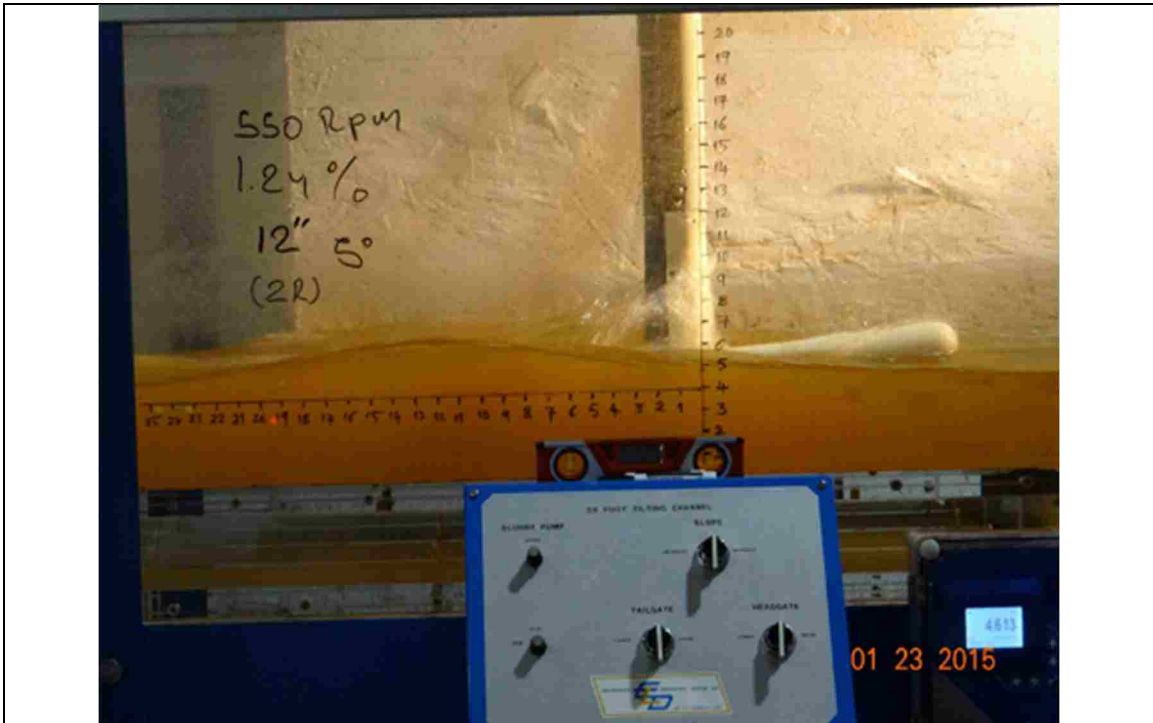
Figure 69. 550 RPM, slope: 1.24%, L_{bb}=12'' , pitch angle = 5^\circ
