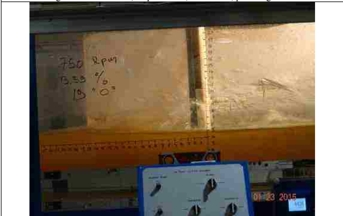
Figure 150. 750 RPM, slope: 3.59%, L_{bb}= 19'' , pitch angle = 0^\circ
