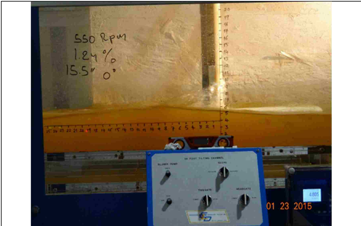
Figure 65. 550 RPM, slope: 1.24%, L_{bb} = 15.5", pitch angle = 0°
