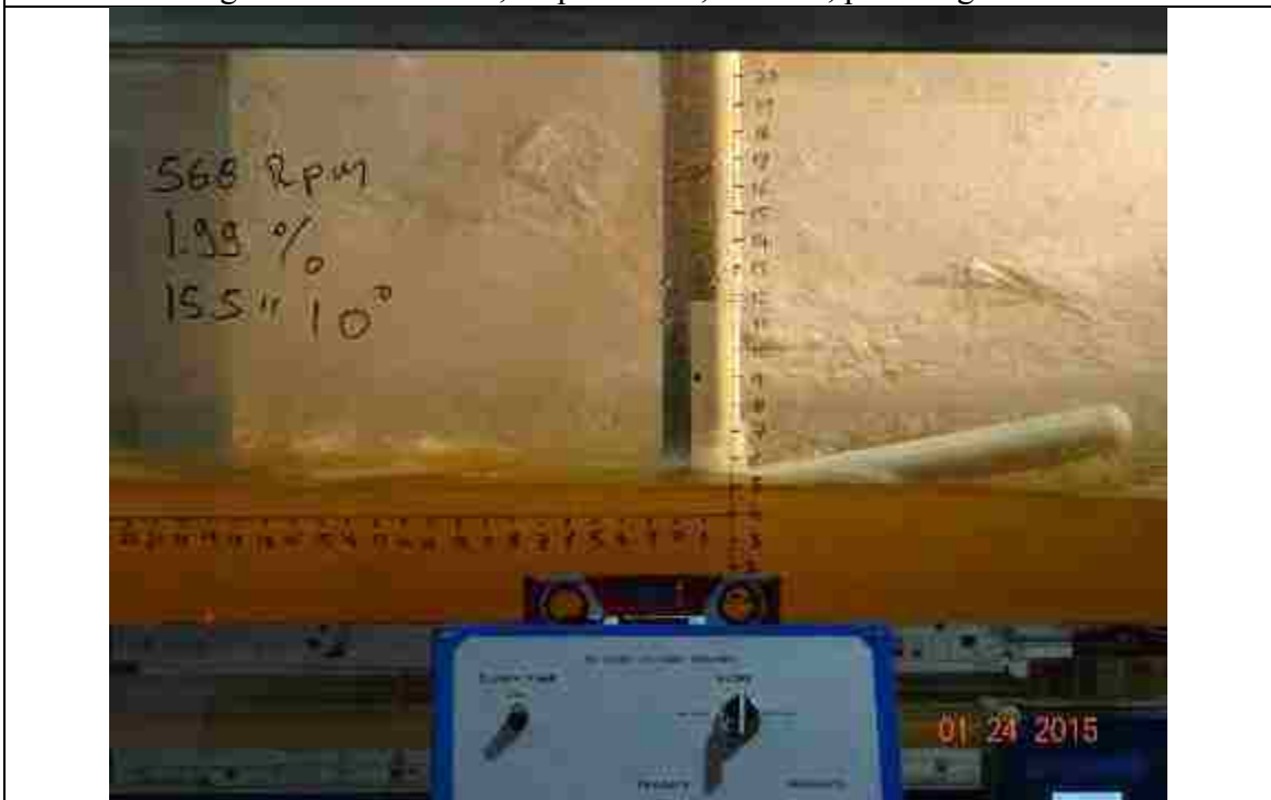
Figure 102. 568 RPM, slope: 1.99%, L_{bb} = 15.5'' , pitch angle = 10^\circ
