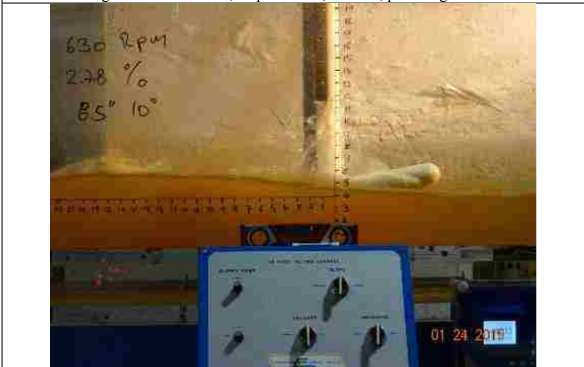
Figure 128. 630 RPM, slope: 2.78%, L_{bb}=8.5'' , pitch angle = 10^\circ
