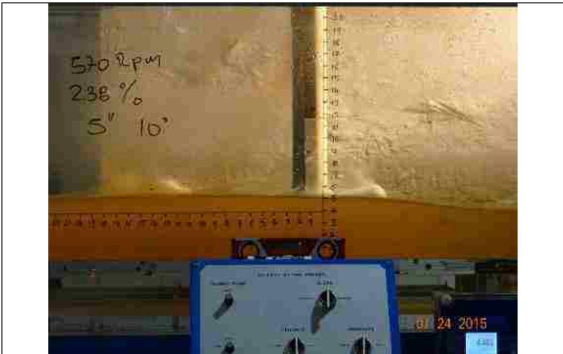
Figure 113. 570 RPM, slope: 2.38%, L_{bb}=5'' , pitch angle = 10^\circ
