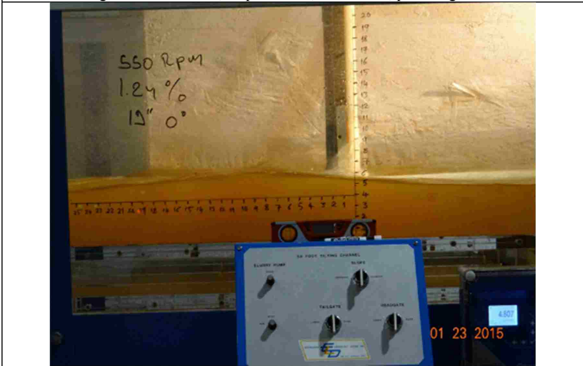
Figure 66. 550 RPM, slope: 1.24%, L_{bb} = 19", pitch angle = 0°
