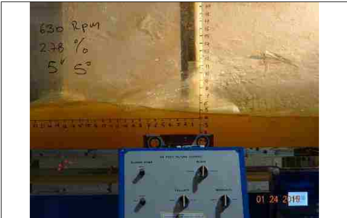
Figure 123. 630 RPM, slope: 2.78%, L_{bb}= 5'' , pitch angle = 5^\circ
