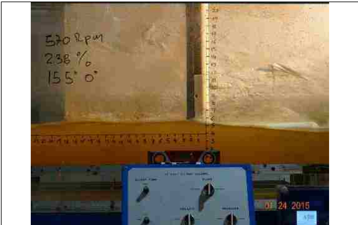
Figure 107. 570 RPM, slope: 2.38%, L_{bb}= 15.5'' , pitch angle = 0^\circ
