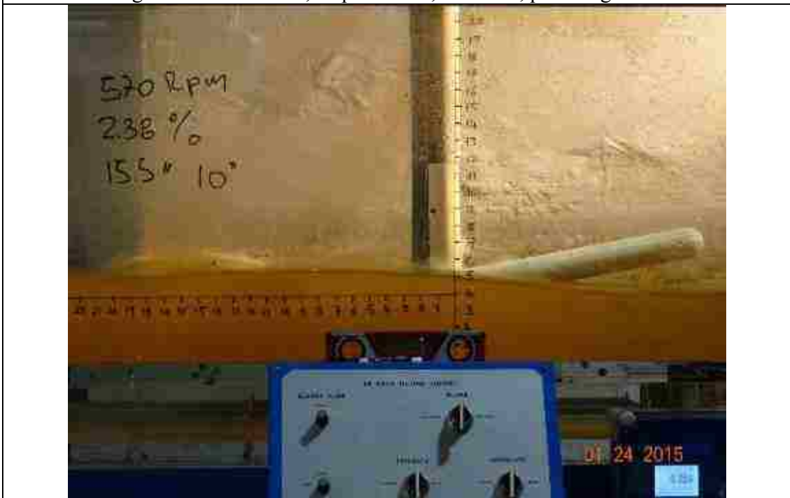
Figure 116. 570 RPM, slope: 2.38%, L_{bb}=15.5'' , pitch angle = 10^\circ
