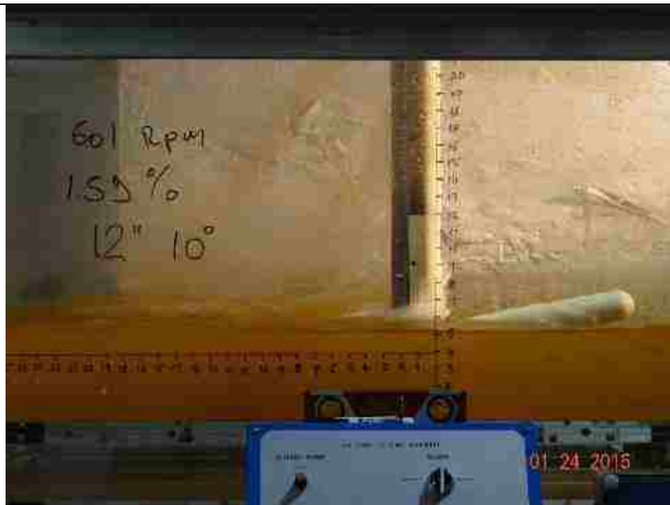
Figure 87. 601 RPM, slope: 1.59%, L_{bb}= 12'' , pitch angle = 10^\circ
