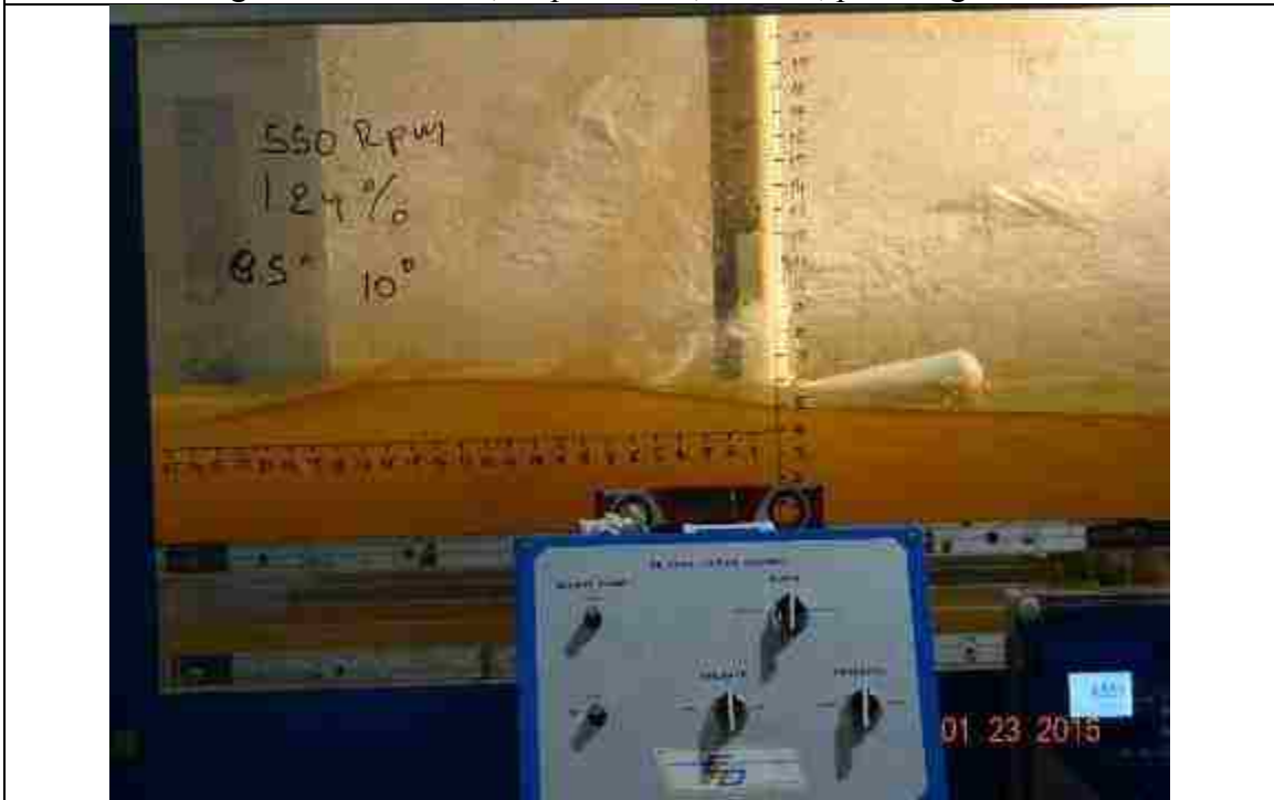
Figure 72. 550 RPM, slope: 1.24%, L_{bb}=8.5'' , pitch angle = 10^\circ
