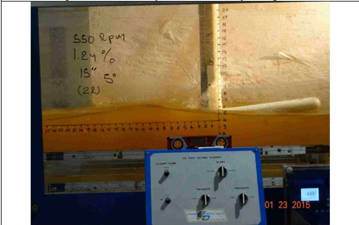
Figure 70. 550 RPM, slope: 1.24%, L_{bb}=15'' , pitch angle = 5^\circ
