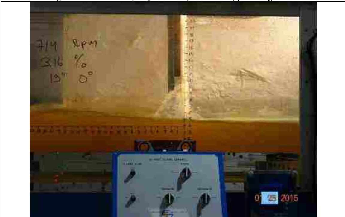
Figure 136. 714 RPM, slope: 3.16%, L_{bb}= 19'' , pitch angle = 0^\circ
