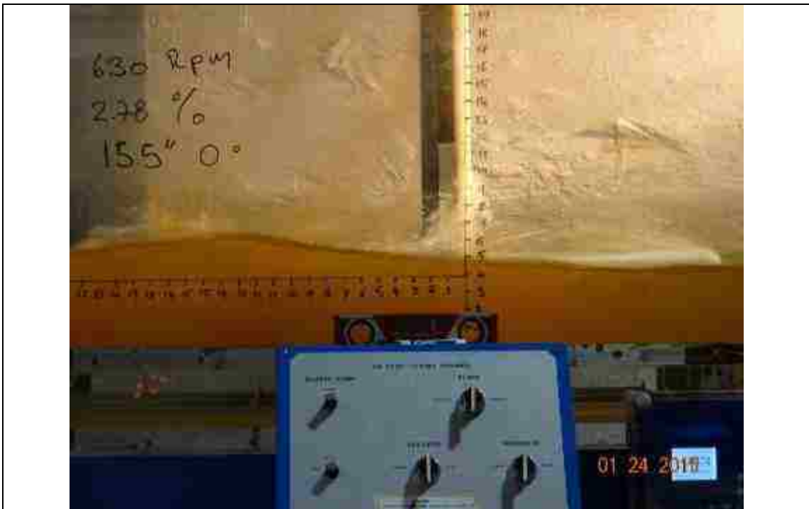
Figure 121. 630 RPM, slope: 2.78%, L_{bb}=15.5'' , pitch angle = 0^\circ
