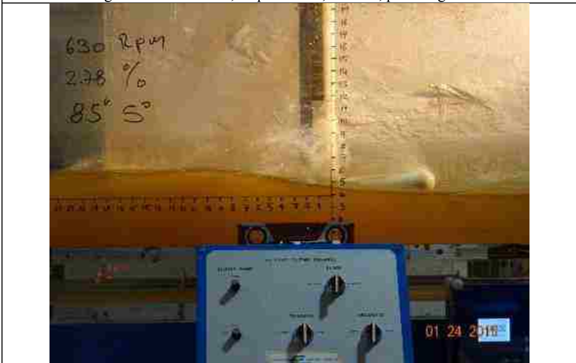
Figure 124. 630 RPM, slope: 2.78%, L_{bb}= 8.5'' , pitch angle = 5^\circ
