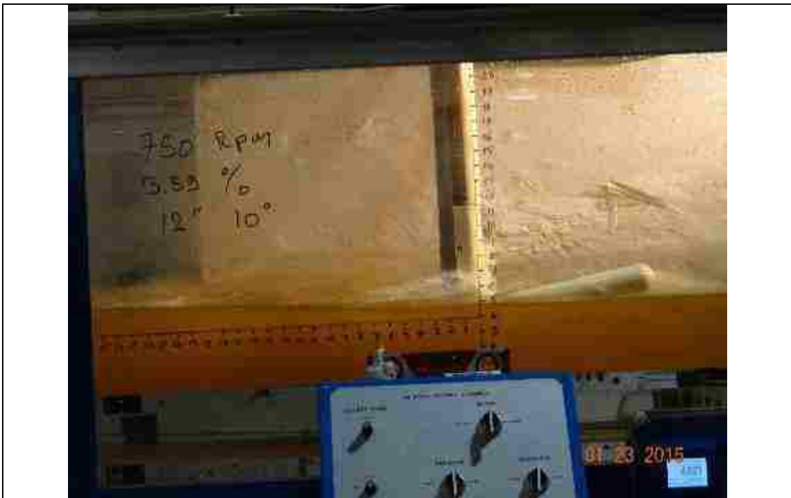
Figure 157. 750 RPM, slope: 3.59%, L_{bb}=12'' , pitch angle = 10^\circ
