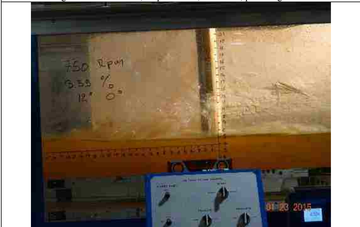
Figure 148. 750 RPM, slope: 3.59%, L_{bb} = 12'' , pitch angle = 0^\circ
