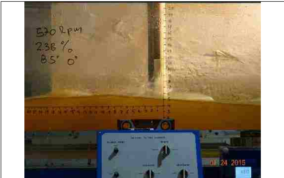
Figure 105. 570 RPM, slope: 2.38%, L_{bb} = 8.5'' , pitch angle = 0^\circ
