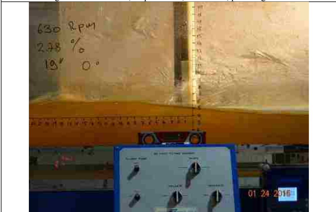
Figure 122. 630 RPM, slope: 2.78%, L_{bb}=19'' , pitch angle = 0^\circ
