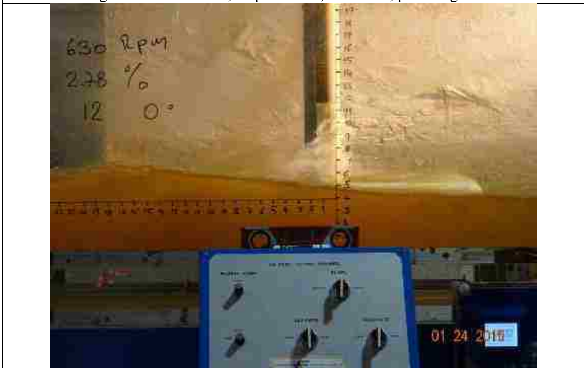
Figure 120. 630 RPM, slope: 2.78%, L_{bb}= 12'' , pitch angle = 0^\circ
