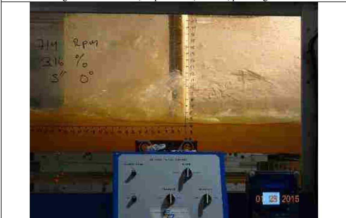
Figure 132. 714 RPM, slope: 3.16%, L_{bb} = 5'' , pitch angle = 0^\circ
