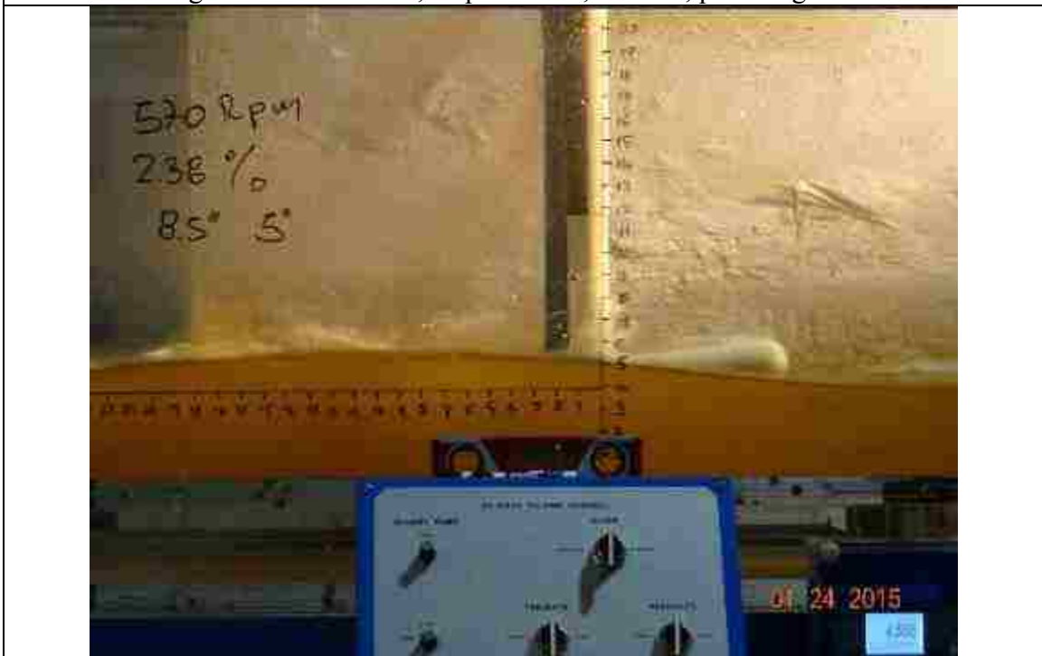
Figure 110. 570 RPM, slope: 2.38%, L_{bb} = 8.5'' , pitch angle = 5^\circ
