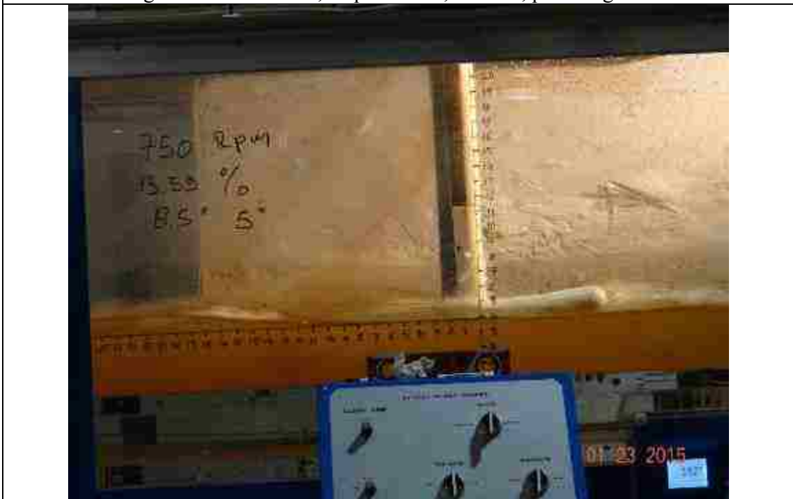
Figure 152. 750 RPM, slope: 3.59%, L_{bb} = 8.5'' , pitch angle = 5^\circ
