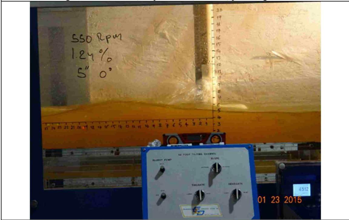
Figure 62. 550 RPM, slope: 1.24%, L_{bb}=5'' , pitch angle = 0^\circ
