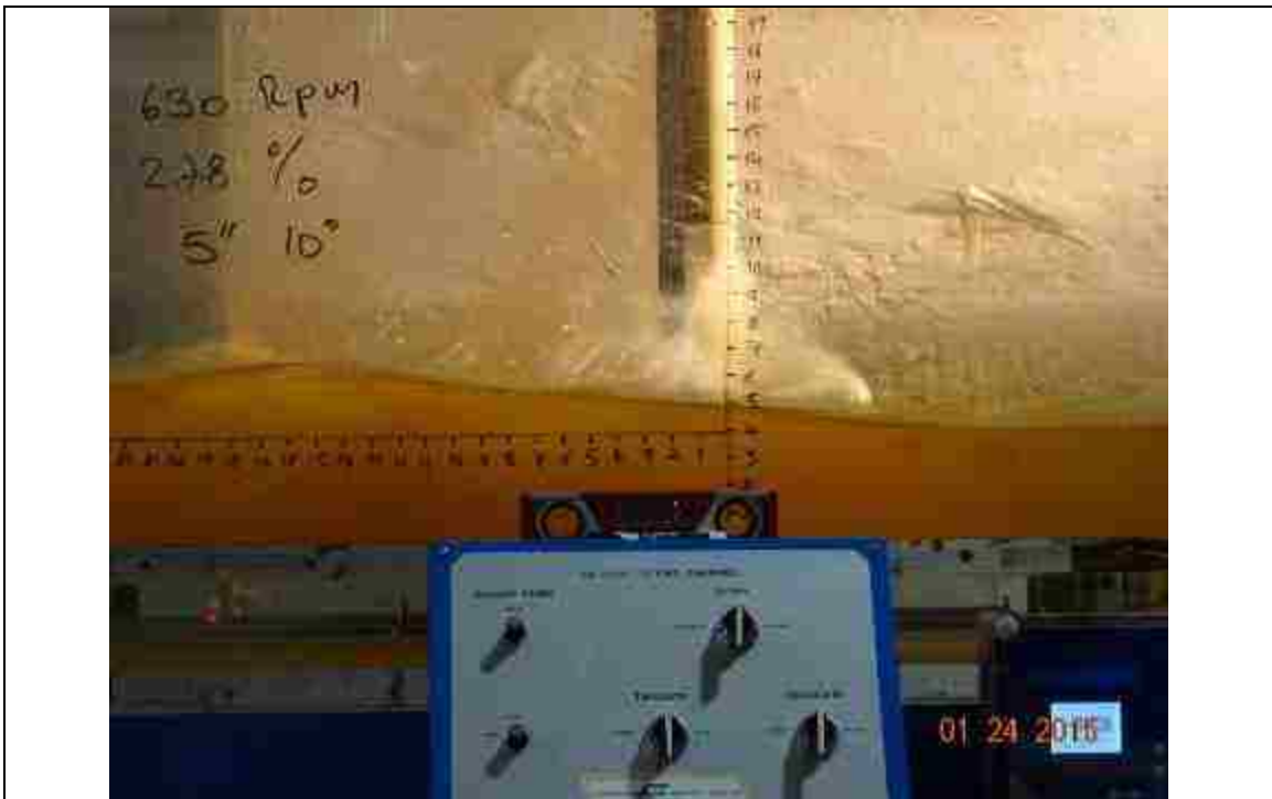
Figure 127. 630 RPM, slope: 2.78%, L_{bb}=5'' , pitch angle = 10^\circ
