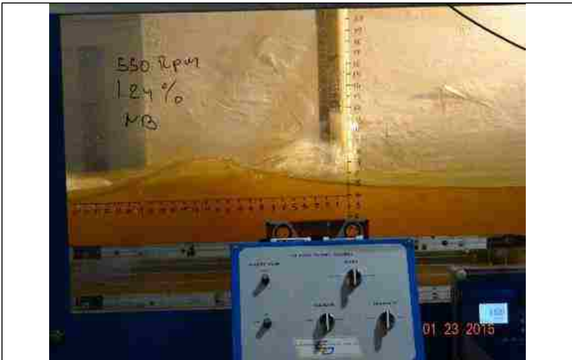
Figure 61. 550 RPM, slope: 1.24%, L_{bb}=0'' , pitch angle = 0^\circ
