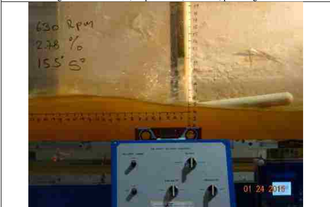
Figure 126. 630 RPM, slope: 2.78%, L_{bb}= 15.5'' , pitch angle = 5^\circ
