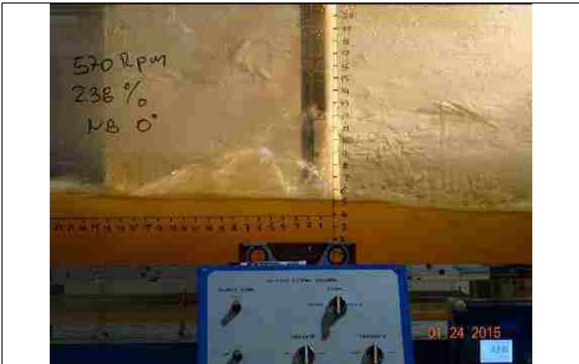
Figure 103. 570 RPM, slope: 2.38%, L_{bb} = 0'' , pitch angle = 0^\circ
