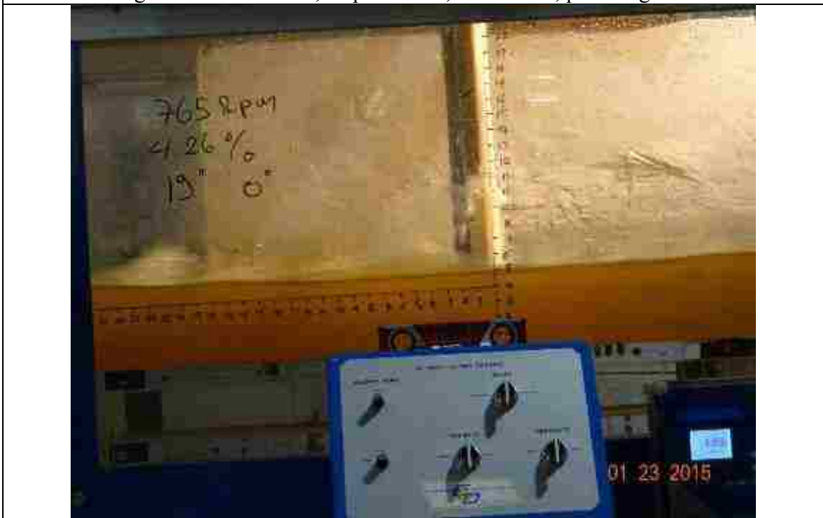
Figure 164. 765 RPM, slope: 4.26%, L_{bb}=19'' , pitch angle = 0^\circ
