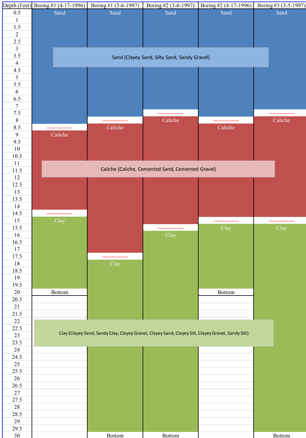
Figure 1.2 Simplified interpretation of borehole logs from the Engineering Geophysics Test Site. Borehole locations are shown on Figure 1.1. The nearest borehole to the cavities is displayed on the far left and the farthest on the far right. The water table is at 3.5 meters (11.5 feet) in depth. (Modified from http://agc.unlv.edu/egts/SoilTrenchLogs )
