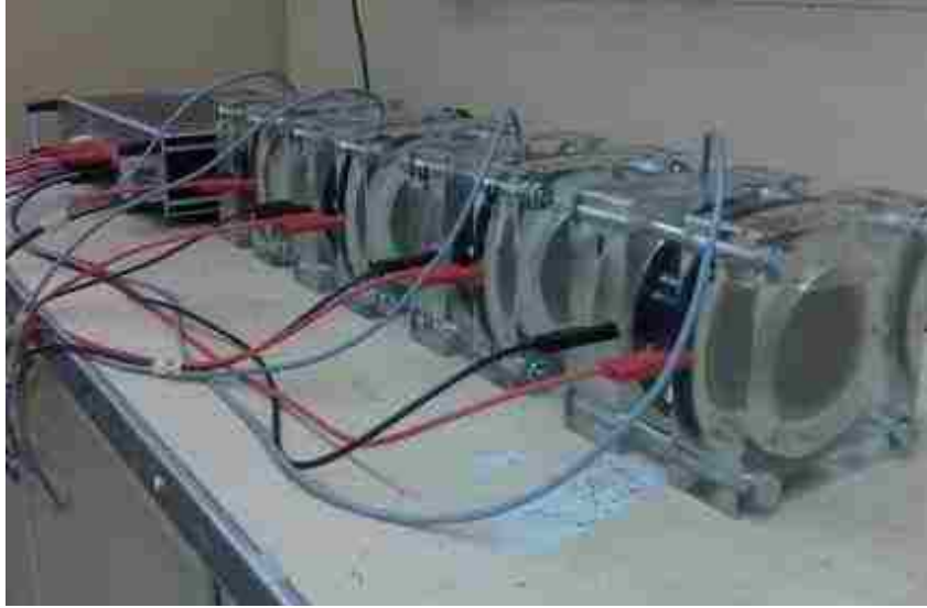
Figure 18 The rapid chloride permeability test setup.
