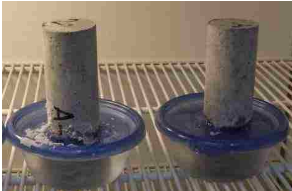
Figure 31 Specimens partially immersed at the early cycles of testing.
