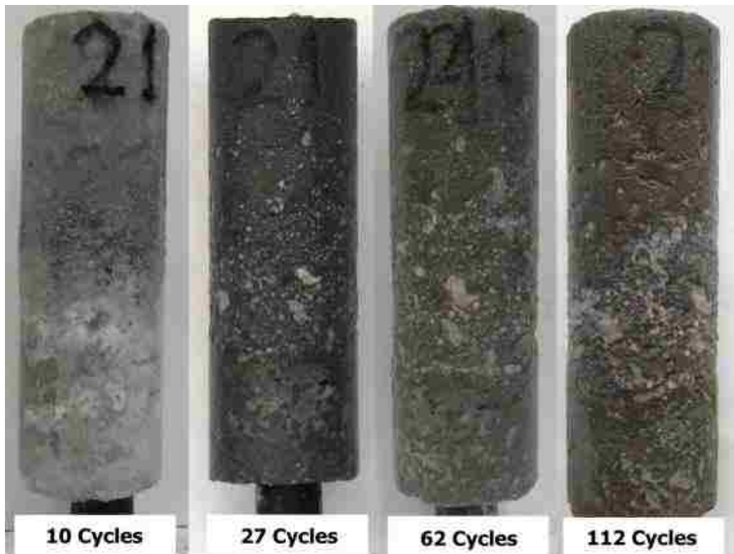
Figure 39 Damage in B-2 specimen at different ages of exposure.
