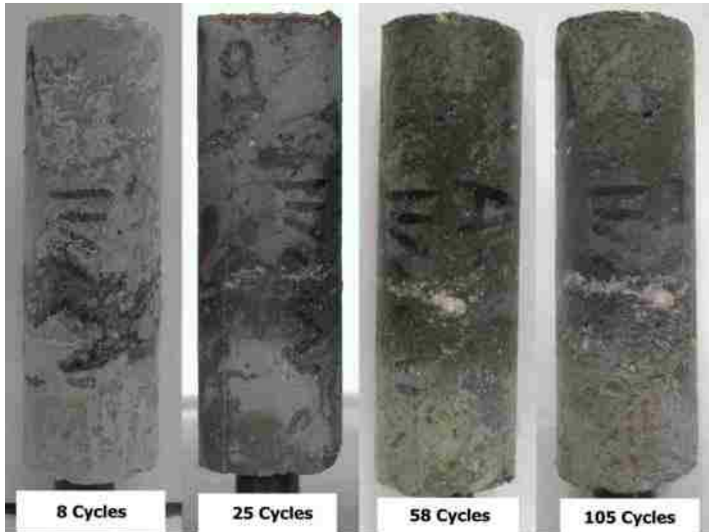
Figure 36 Damage in A-2 specimen at different ages of exposure.
