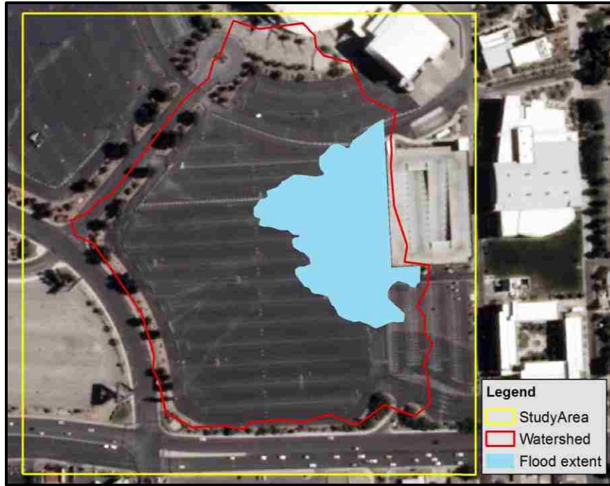
Figure 5.1-18: Inundation extent after 590 minutes of rainfall in Blacklot watershed
