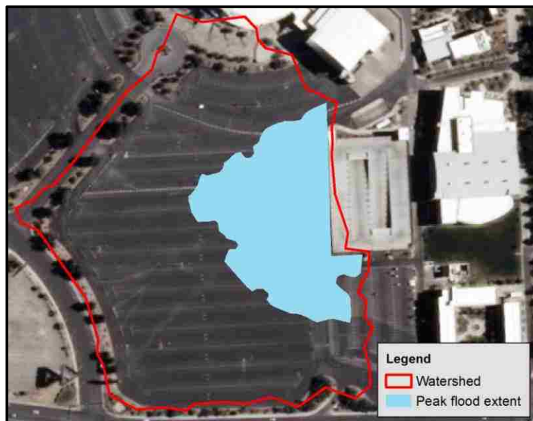
Figure 6.3-9: Peak inundation extent for grass swale strip
