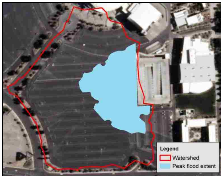
Figure 6.3-6: Peak inundation extent for gravel swale strip
