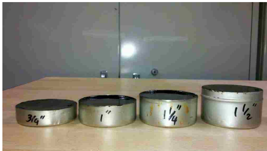
Figure 5-15 Samples with Different Thicknesses Tested to Obtain the Minimum Thickness
