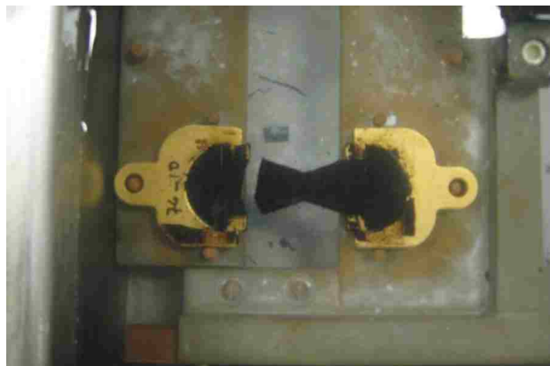
Figure 6-4 Type 3 Failure in the Ductility Test
