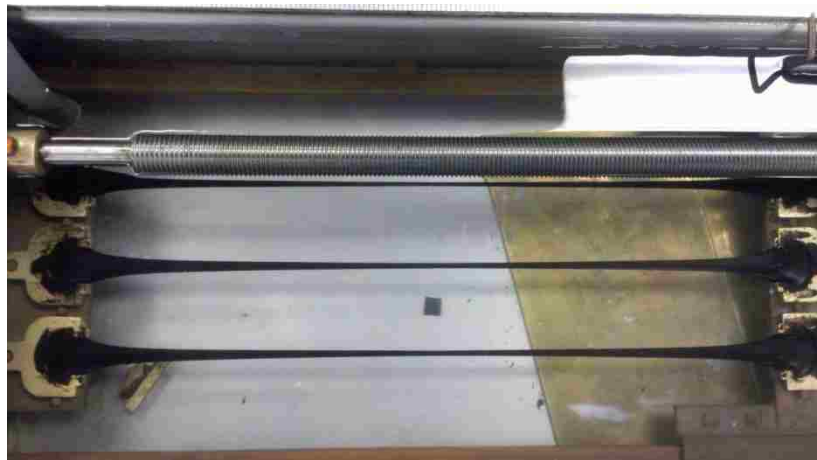
Figure 6-2 Type 1 Failure in the Ductility Test
