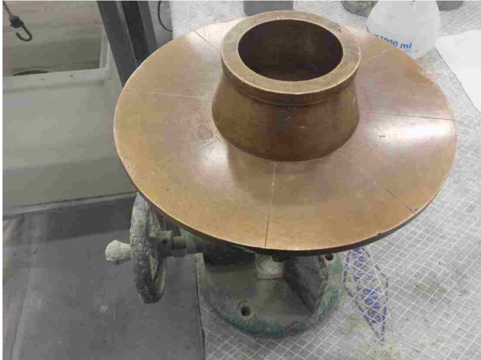
Figure 2.4. Flow Table used for Slump Flow Measurements
