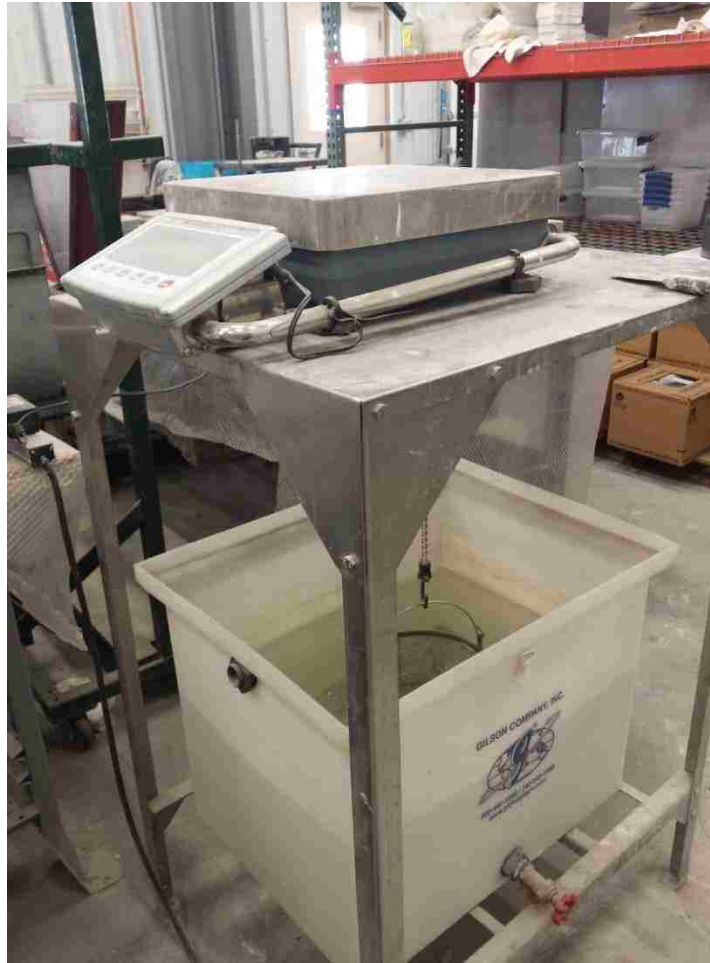
Figure 2.15. Scale used for the Measure Mass of Test Sample in Water
