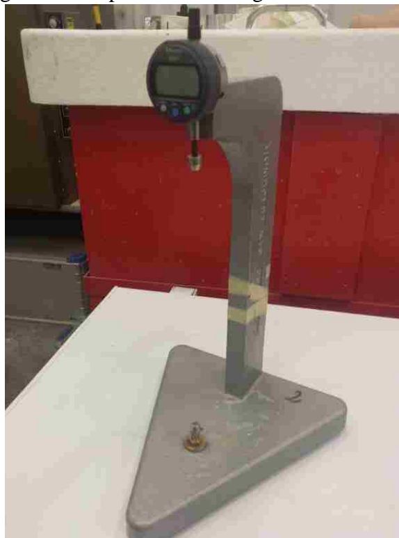
Figure 2.8. Length Comparator and Digital Indicator used for Sulfate-Induced Expansion Measurements
