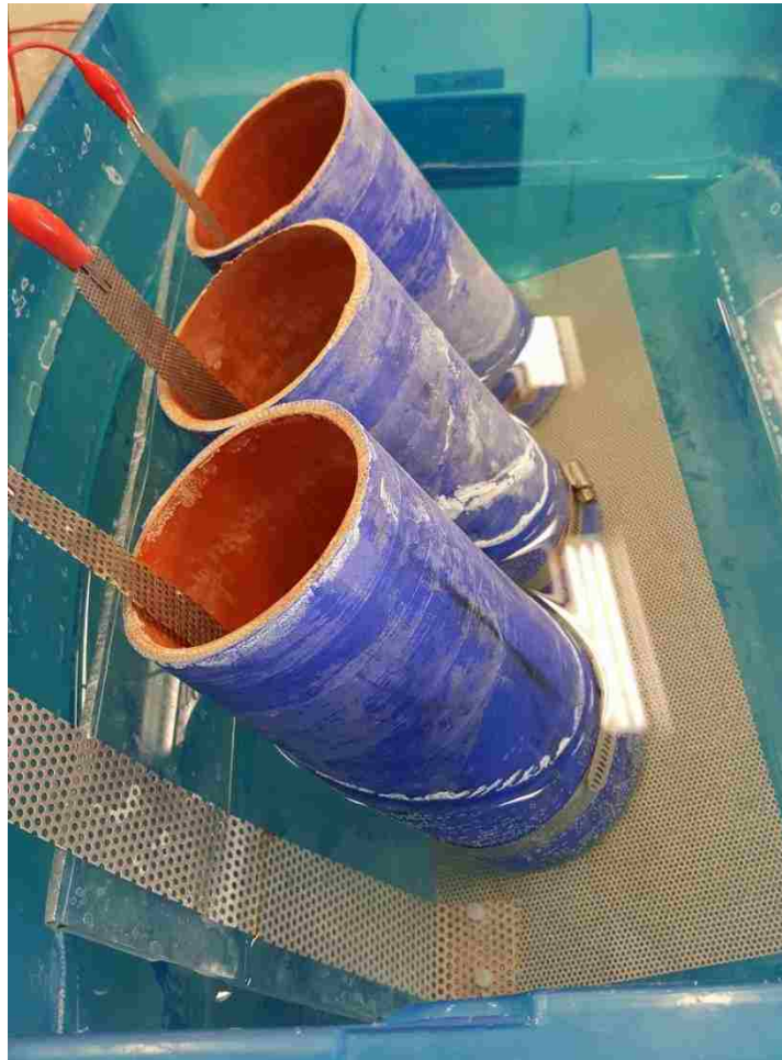
Figure 2.14. Rapid Chloride Migration Sample Test Set-Up
