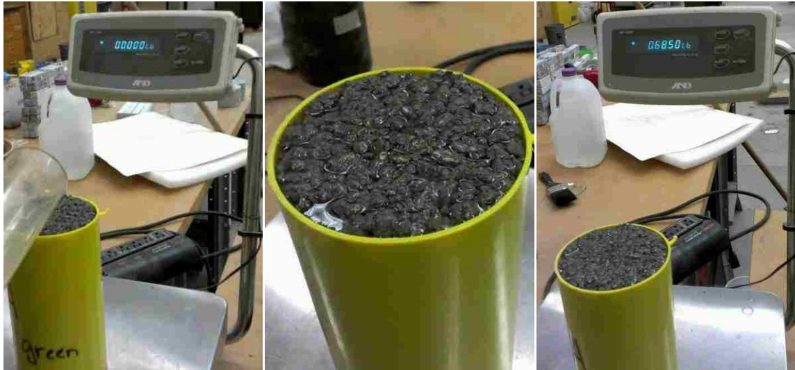
Figure 3.8. Images of porosity testing process
