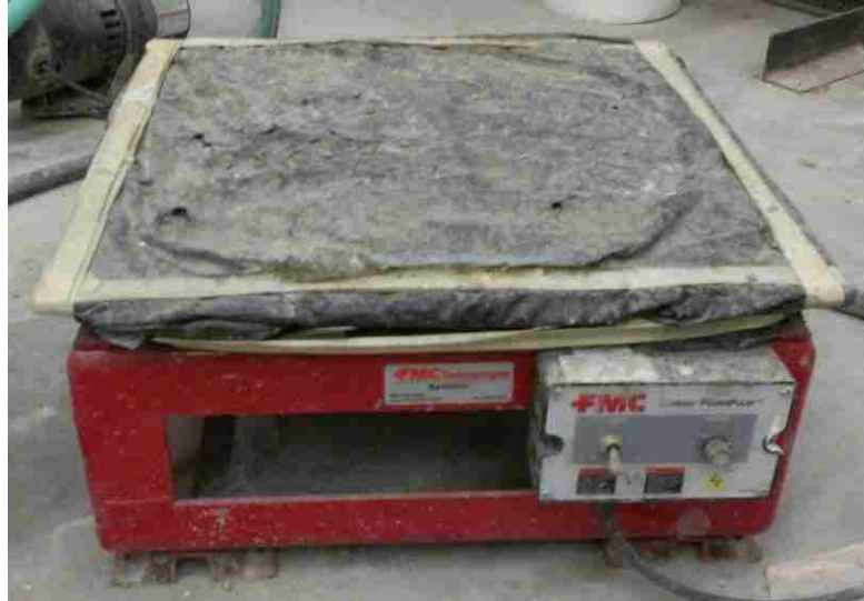
Figure 3.3. Machine used to assist in concrete compaction
