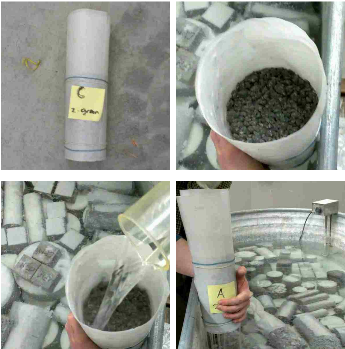
Figure 3.9. Various stages of the permeability testing process
