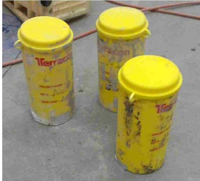
Figure 3.1. Concrete 4" x 8" cylinder molds
