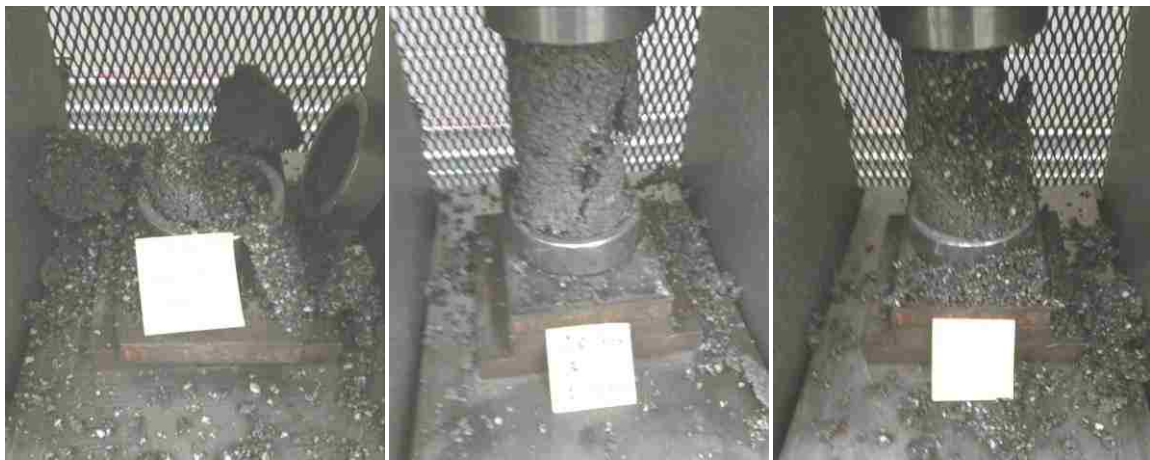
Figure 3.13. Select compression failures (left to right) for plain, 5% and 10% PC
