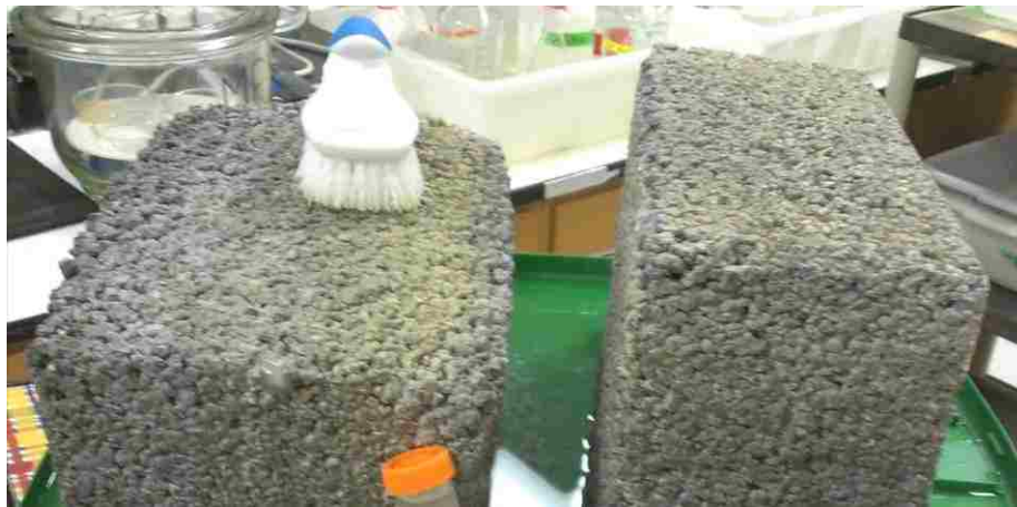
Figure 3.5. Residue on PC slabs after curing
