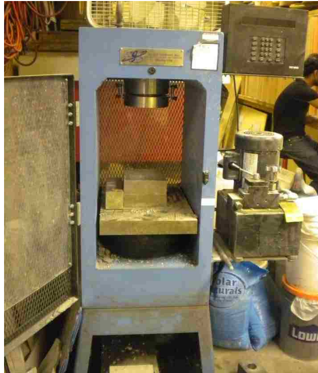
Figure 2.5: Compressive testing machine
