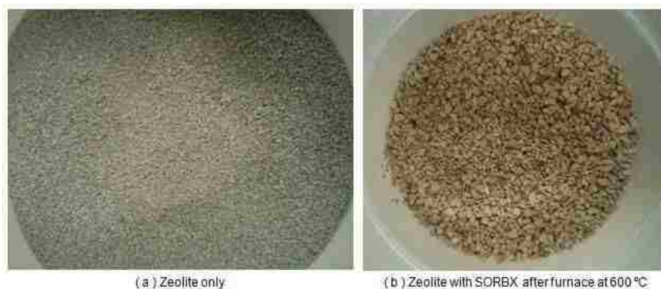
Figure 5: Media preparation with modified media preparation with 0.4 M Sorbx-100 5% (w/w) with zeolite. a) virgin zeolite; b) zeolite with Sorbx-100 anthracite after furnace dry at 600°C.
