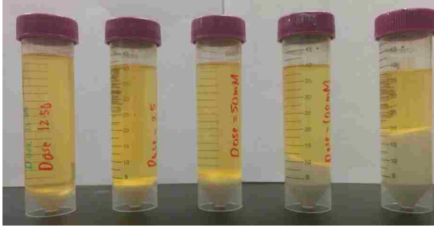
Figure 20: Sludge production with increasing cerium dose on SCS solution, with initial fluoride concentration 41 mg/L.
