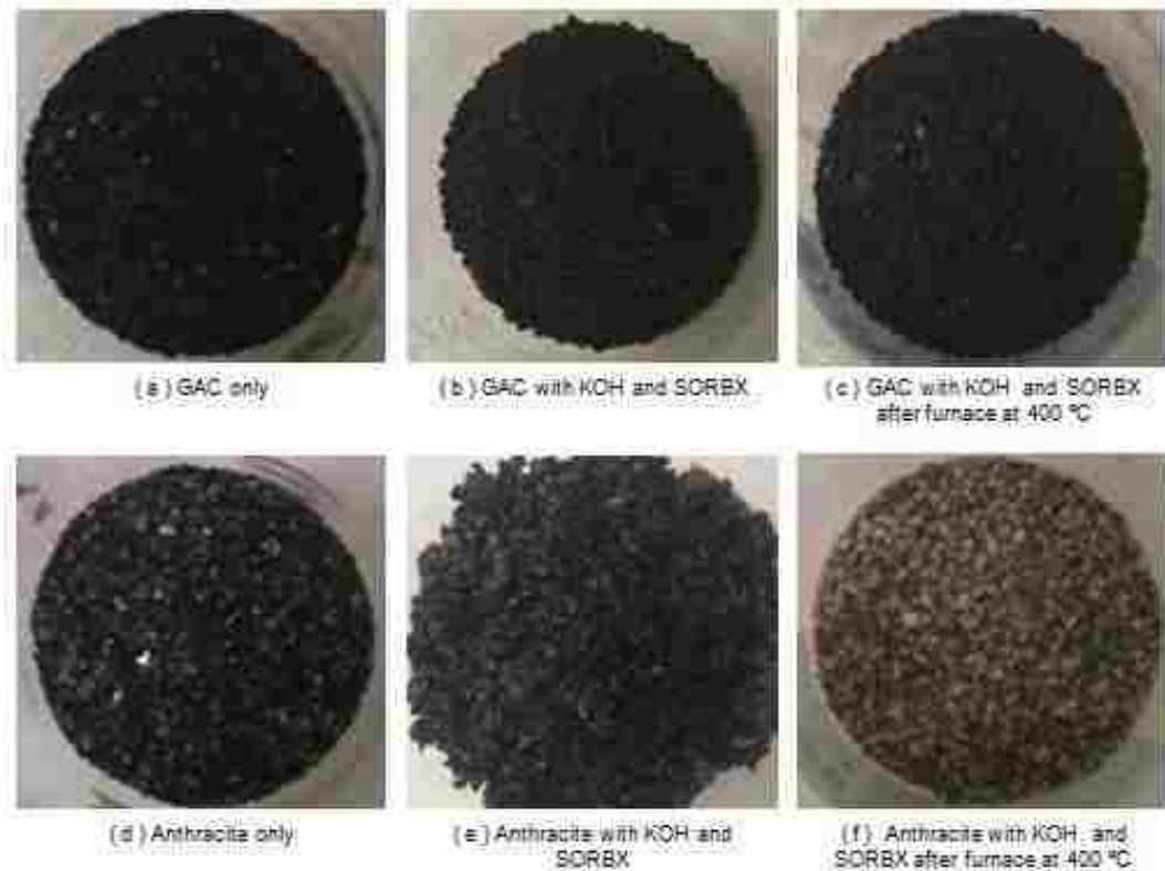
Figure 4: Media preparation with different reactants. a) virgin GAC; b) GAC with KOH and Sorbx-100; c) GAC after furnace dry at 400 °C; d) virgin anthracite; e) anthracite with KOH and Sorbx-100; f) anthracite after furnace dry at 400 °C.
