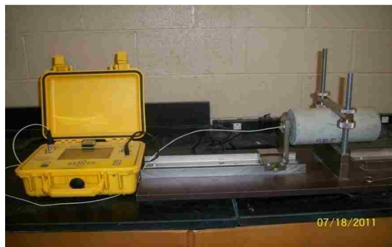
Figure 19. Concrete dynamic Young's modulus of elasticity using E-meter MK II.
