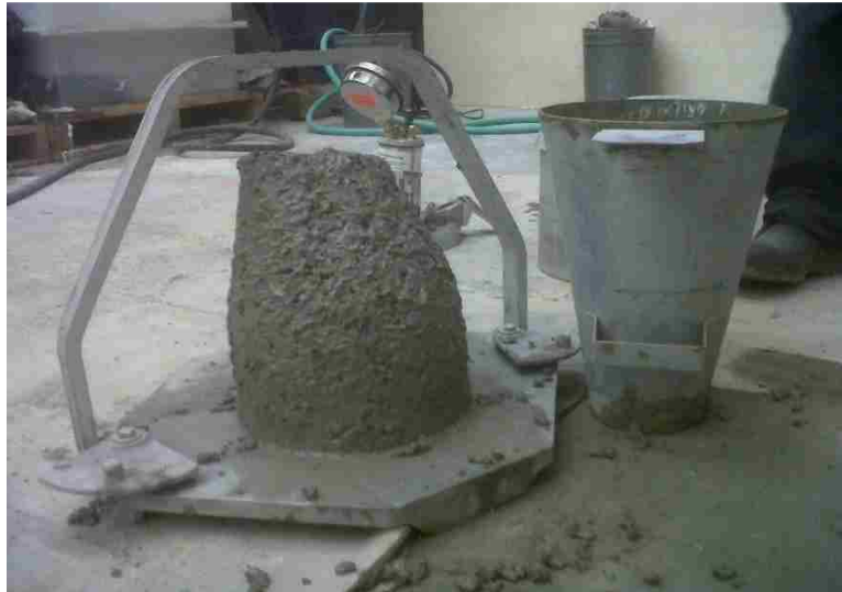
Figure 11. Concrete slump test.
