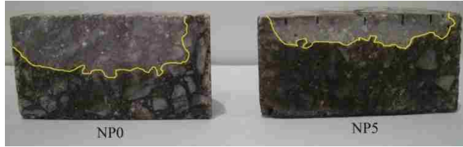
Figure 33. NP0 and NP5 Chloride ion penetration depths at 28 days.
