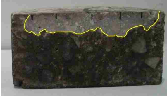
Figure 21. Specimen after rapid chloride ion migration test.
