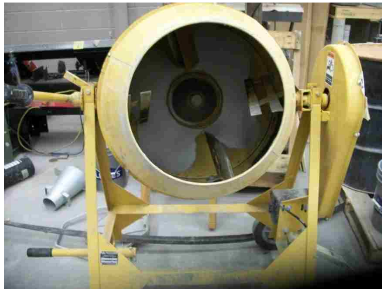
Figure 22. Steel drum mixer.
