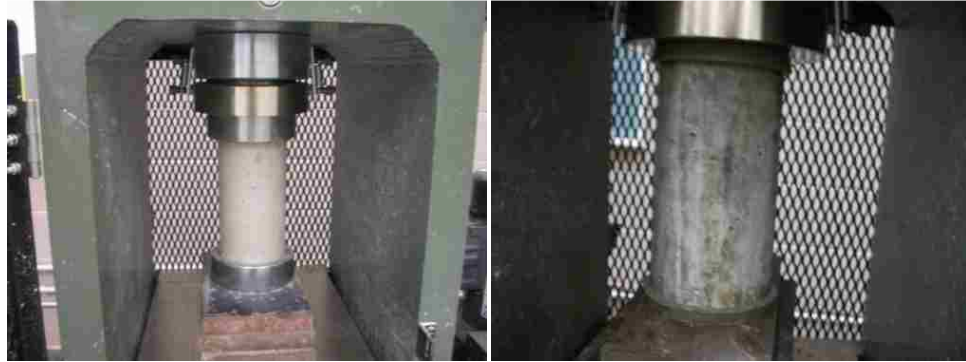
A- Test with unbounded capping
