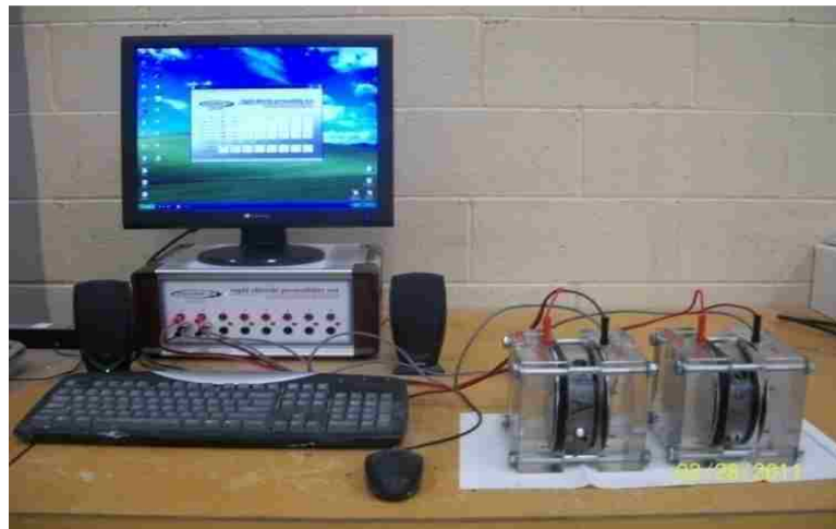
Figure 20. Concrete rapid chloride ion penetration test setting.
