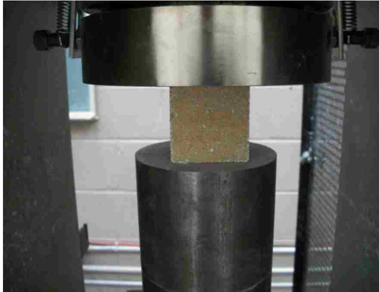
Figure 10. Mortar cube compressive strength test.
