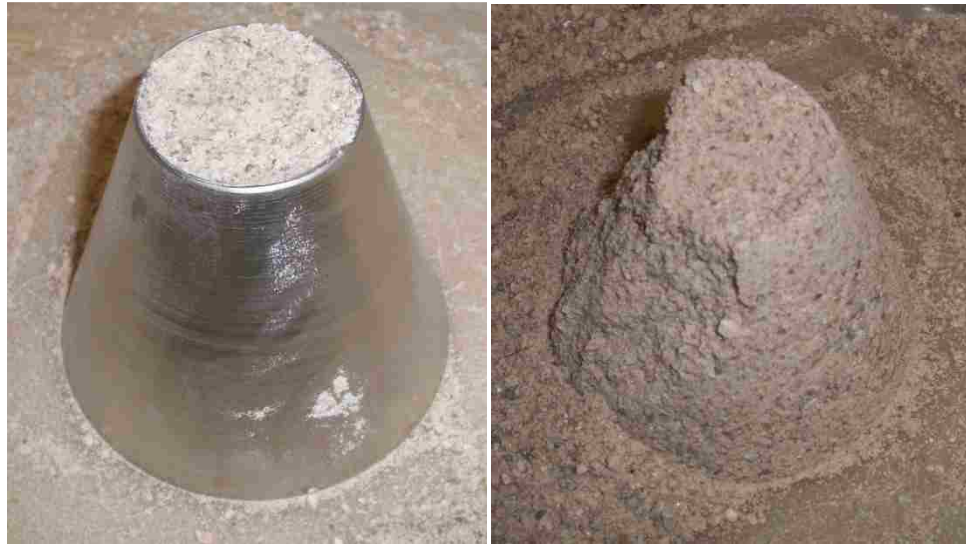
Figure 41. Cone test for surface moisture.
