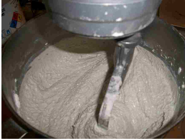
Figure 55. Metakaolin based geopolymer mortars preparation.
