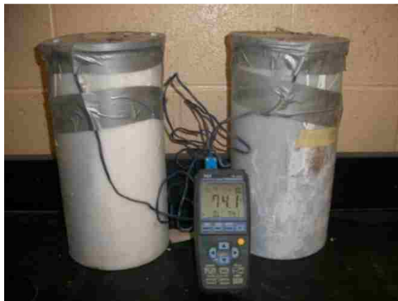
Figure 14. Temperature of freshly mixed concrete test setting.
