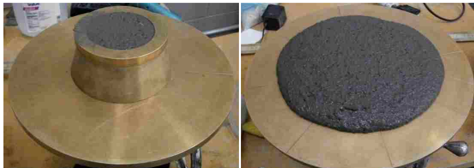
Figure 38. Geopolymer mortar flow test.
