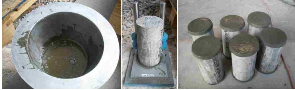
Figure 15. Sulfur capping preparation.
