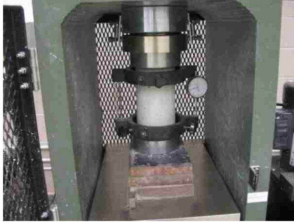
Figure 18. Concrete static modulus of elasticity test setting.
