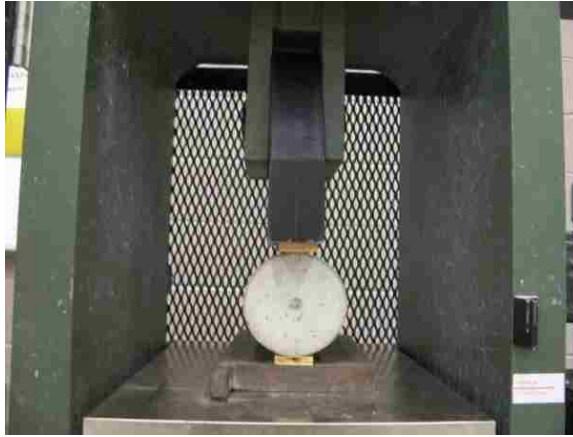
Figure 17. Concrete splitting tensile strength test setting.
