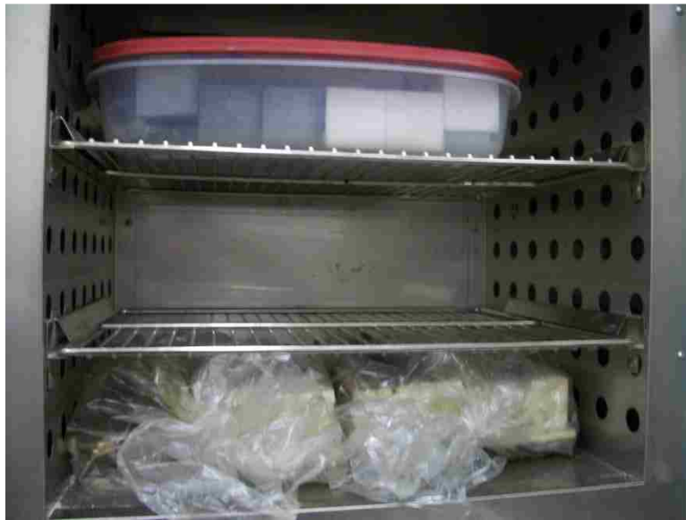
Figure 42. Geopolymer mortars specimens inside an oven.
