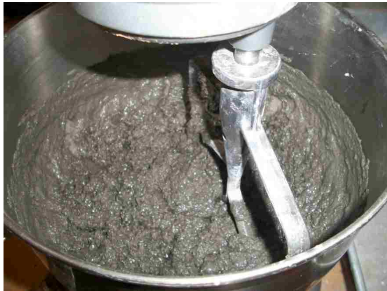
Figure 44. Fly ash based geopolymer mortar mixing.
