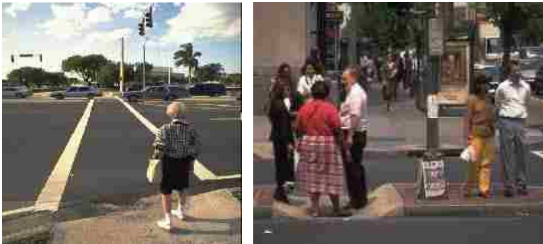
Figure 2-12. Pedestrian on Left Cannot Safely Cross. Pedestrian Island, on Right. (Campbell et al., 2004, p. 85-86)
