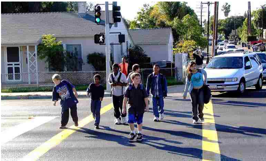
Figure 2-7. Standard Pedestrian Button-Activated Traffic Signal (Turner et al., 2006)
