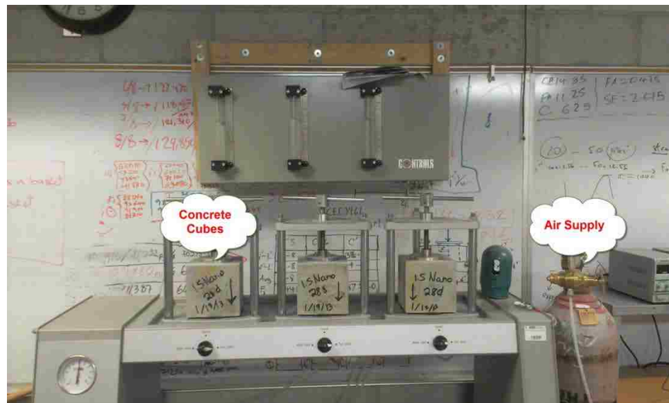
Figure 3.11: Concrete Water Penetration Testing Apparatus
