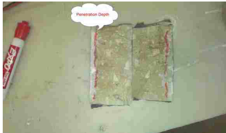
Figure 3.15: Chloride Penetration Depth after Applying Silver Nitrate to the Freshly Split Sections
