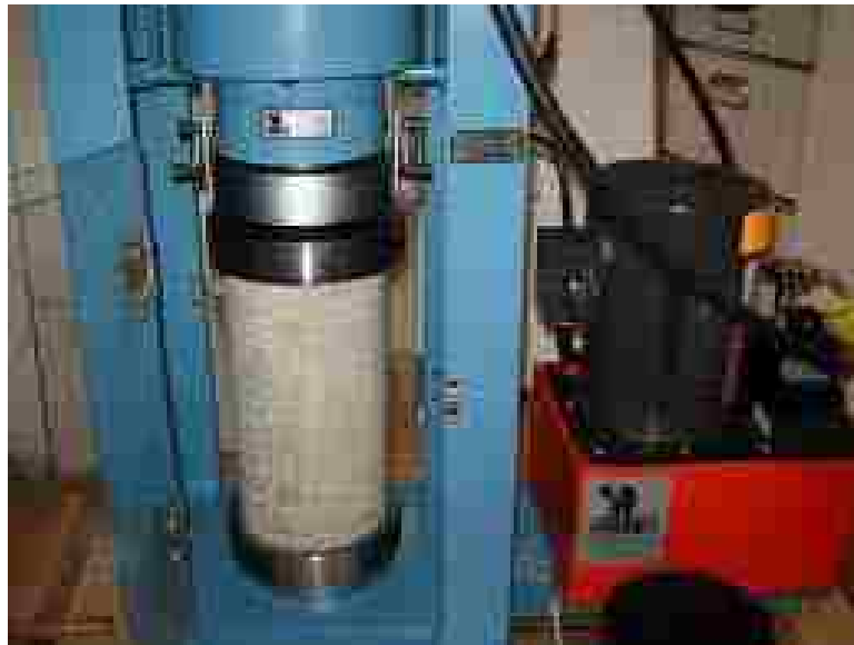
Figure 3.7: Concrete Cylinder Experiencing Axial Load
