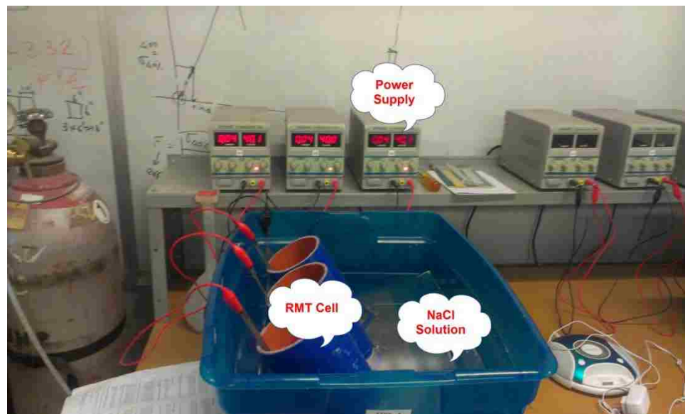
Figure 3.14: Rapid Migration Test Setup
