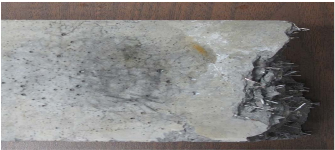
Fig. 5-10: Fiber orientations of a beam sample.
