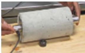
Fig. 5-1: Longitudinal measurement for cylindrical samples.
