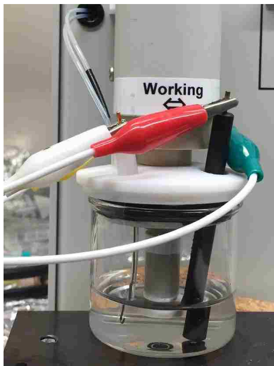
Figure 2-4. RRDE experimental set up. The electrode connections 1) Green for disk electrode 2) Red for counter electrode 3) White for reference electrode 4) Yellow for ring electrode. 5) Two white tube, one for argon out and another for out.
