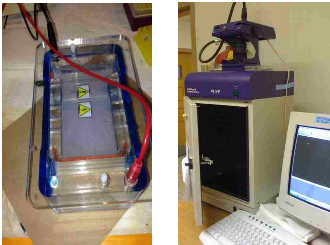
Figure 20 Agarose gel electrophoresis (left) and Foto/UV 26 where the gel is exposed to UV radiation and picture obtained.
