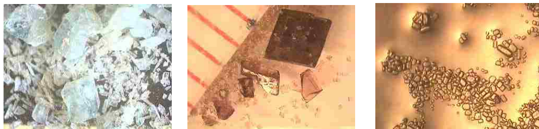
Figure 2.4. Left: Photograph of the mixture of crystals obtained after recrystallization of 1 by vapor diffusion of Et 2 O into a 0.025 M CH 3 CN, filtering, and after drying under vacuum producing a mixture of large blocks of co-1 and smaller plate-like needles of cis-1 and trans-1 . Center: Photograph of crystals of trans-1 ·2CH 3 CN obtained after cooling a CH 3 CN solution of 1 to -20°C, decanting the mother liquor and (immediately) after drying under a nitrogen stream. Right: Crystals of trans-1 ·4CH 3 CN in their mother liquor. Each photograph was taken under the same magnification.
