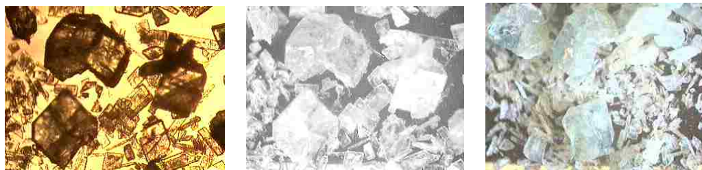
Figure 3.1. Photographs (left and center are the same but under different external lighting) of the mixture of crystals obtained after recrystallization of 1 by vapor diffusion of \text{Et}_2\text{O} into a 0.025 M \text{CH}_3\text{CN} , filtering, and after drying under vacuum.
